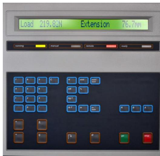
Figure 20 Control panel during Indentation force deflections test showing a 219.82N compression load and a deflection (Extension on the panel) of 76.7mm
