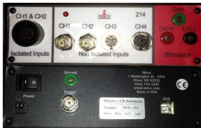
Figure 14 Front and rear panels of IWX/214
