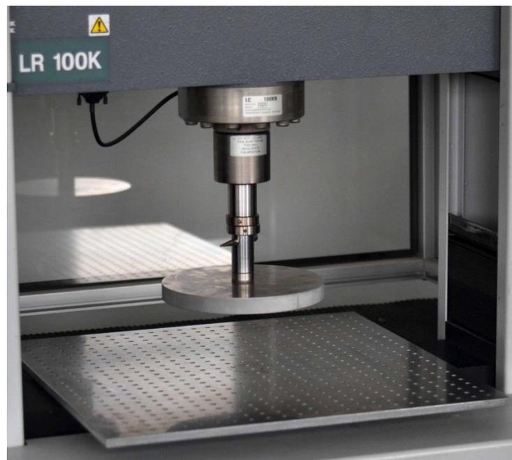
**Figure 18** Screw-driven test machine (LR 100K, Lloyds Instrument, Bognor Regis, UK) with a 100kN load cell showing the 203mm indenter foot above the perforated horizontal support plate
