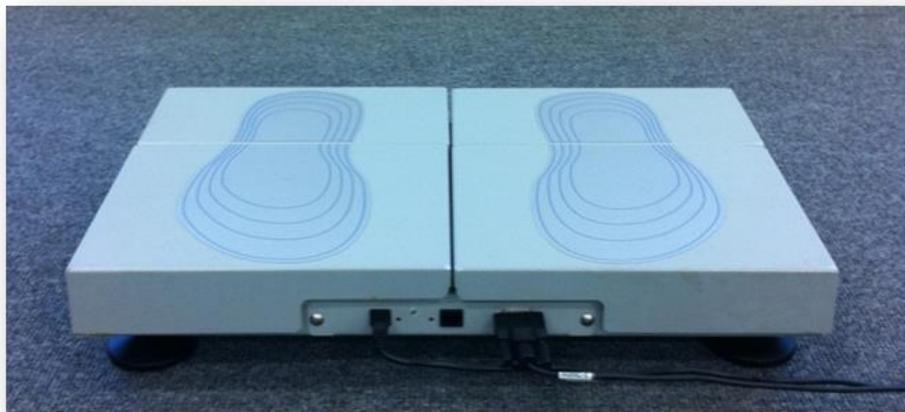
**Figure 11 Force platform: QPS-200, and software; Posture Analyser**
