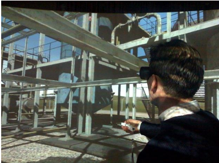
Figure 2.2 Operator training in a 3D virtual reality environment [Source: Virthualis company, www.virthualis.com ]
