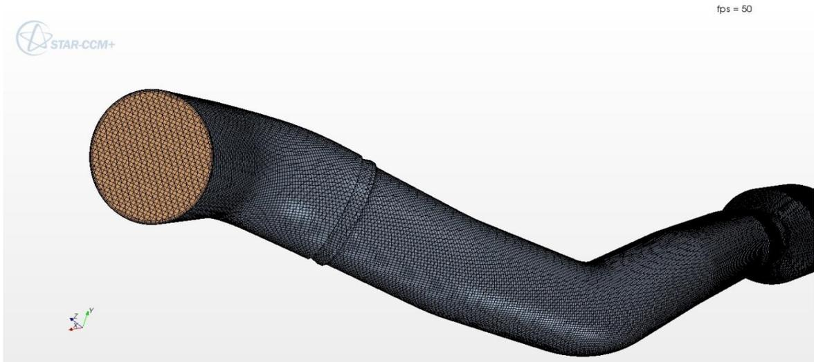
Figure 128: CAC resonator upstream pipe and inlet volume mesh
