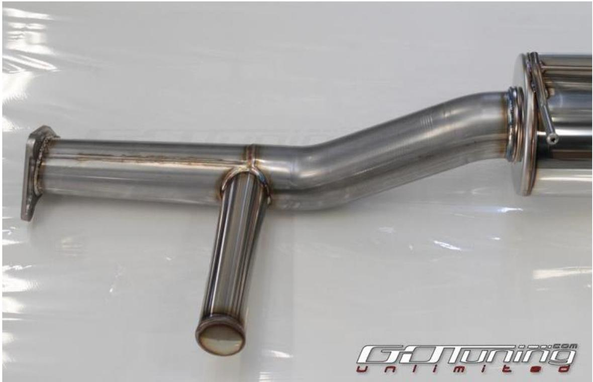
Figure 1: A typical exhaust with closed side-branch (Go Tuning Unlimited, 2010)
