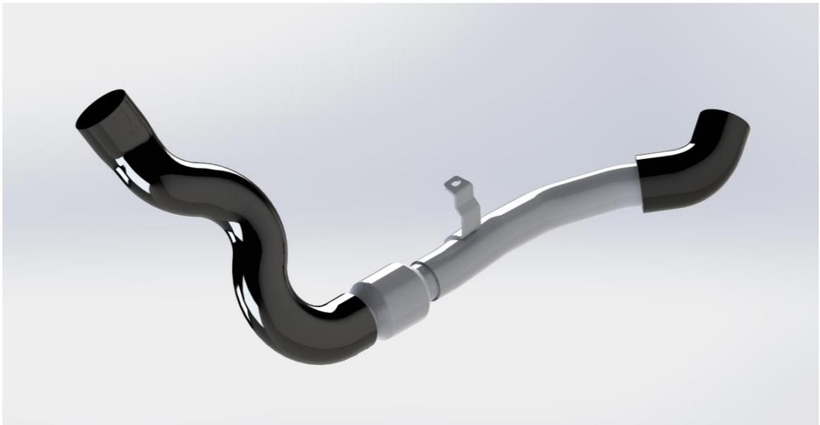
**Figure 125: CAC tract geometry - CAD representation**
