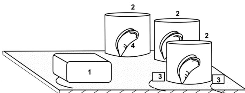
**Figure 5.2 Schematic of experimental setup used to expose *M. edulis* to vibration, consisting of three arenas in an arc around a vibration source, vibration source (1), experimental arena (2), position of acceleration and velocity sensors (3), *M. edulis*, one in each arena for solitary tests four per arena for grouped tests (4).**
