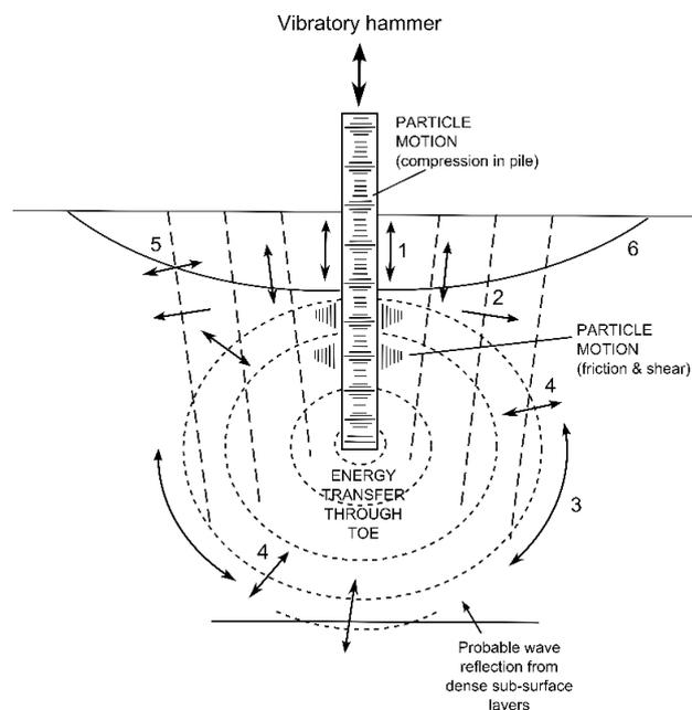
**Figure 1.5 Mechanisms of seismic waves during pile driving (vibratory or impact) into soil 1. Particle motion within the pile (compressional), 2. Shear wave front, 3. Body wave front S-wave spherically expanding, 4. P-wave, 5. Interaction between reflected P wave and S wave causing surface motion, 6. P-wave reflection (minor surface reflection), adapted and expanded from Athanasopoulos and Pelekis (2000); Kim and Lee (2000).**
