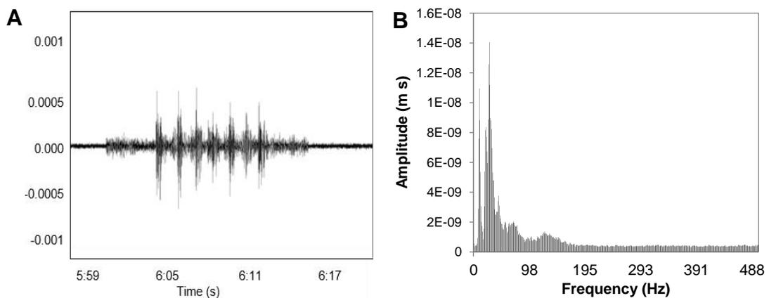
**Figure 4.17 Time history of impulsive vibration exposures (shell auger piling) within the experimental tank (A); Amplitude spectrum of the playback signature (B).**
