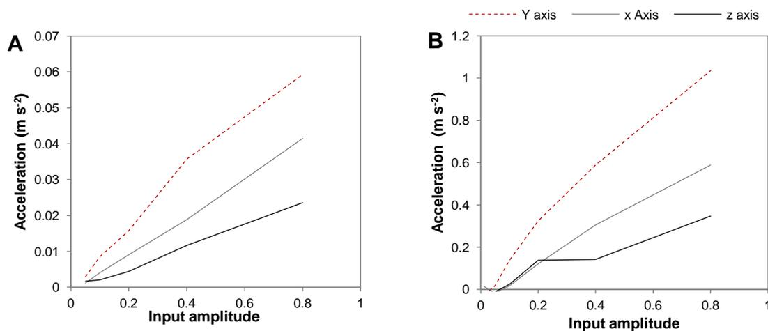
**Figure 4.12** The relative proportion in each axis (x, y, z) of the sinusoidal signal, for example at 40 Hz (A) and at 210 Hz (B). Maximum input amplitude (x axis) is 0 dB, denoted as 1, reducing in -6 dB steps.
