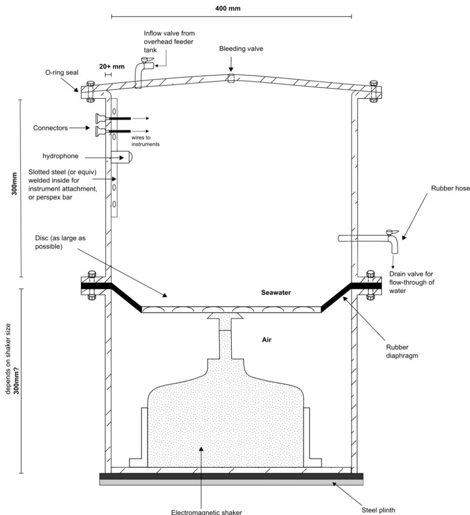
**Figure 4.20 Schematic of a tank specifically designed to investigate the response of crustaceans to the particle motion component of sound (based on discussion with A. Hawkins *Pers. Comm.*<sup>6</sup>, as part of the SoundWaves consortium). The tank would be constructed from a thick walled steel tube, with a diaphragm at the base connected to an electromagnetic shaker.**
