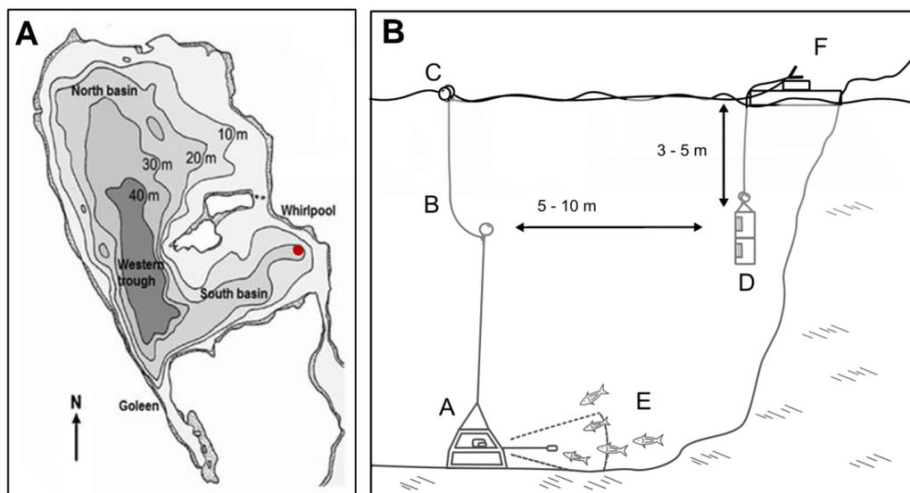
**Figure 3.9** Sampling location for BRUV deployments in the Whirlpool area of Lough Hyne (A), circled in red, may 2012; Deployment diagram of the BRUV and sound projector array from the shore (B), A. BRUV frame, B. subsurface buoy, C. Pellet for retrieval of frame with umbilical cable to shore, D. Transducer array (2 – 6 projectors), E. Field of view, F. Observer station on shore with laptop and playback controls.
