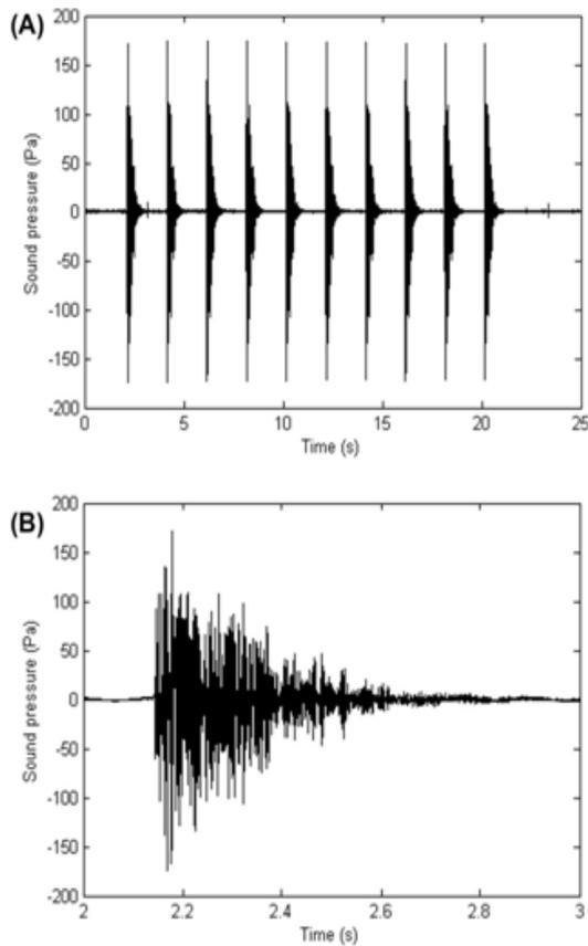
FIG. 6. Time history of sound pressure measurements for one complete 20 s playback of synthetic piling noise. (B) Expanded view of the first strike. These sound measurements were made 5 m below the sound projectors.
