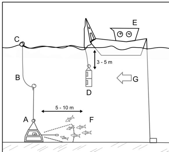
**Figure 3.7** Deployment diagram of the BRUV and sound projector array from an anchored vessel. **A.** BRUV frame, **B.** subsurface buoy with umbilical cable to boat, **C.** Pellet for retrieval of frame, **D.** Transducer array (2 – 6 projectors), **E.** experimental vessel with A frame for deployment of equipment, **F.** Field of view, **G.** tidal direction.
