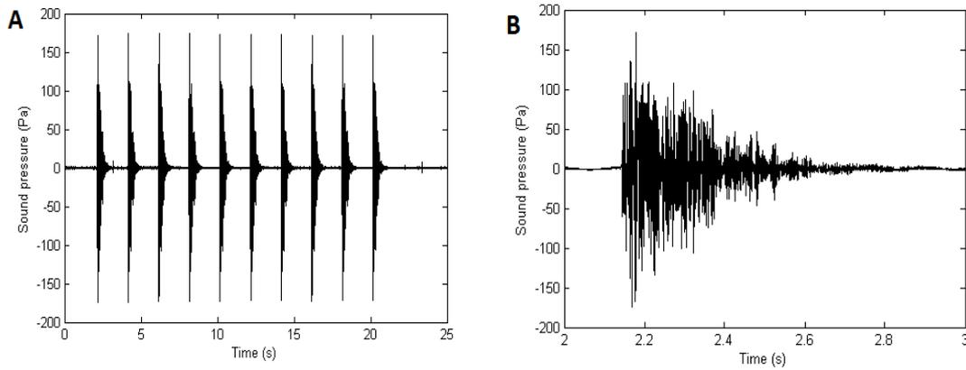
**Figure 2.5** Sound measurements taken at 4 m (5 m from the sound projectors) on 19<sup>th</sup> March 2013. Time history of sound pressure measurements of one 20 s playback of synthetic piling (A); Expanded view of a single playback strike (B). Data courtesy of Subacoustech Ltd.
