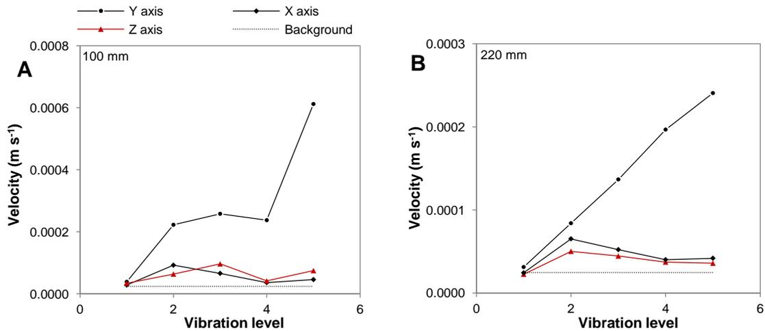
Figure 5.5 Velocity measurements of the five vibration levels (1 – 5), taken at either 220 mm (A) or 100 mm (B) distance from the vibration box. A dashed line indicates average background levels ( $\text{m s}^{-1}$ ).
