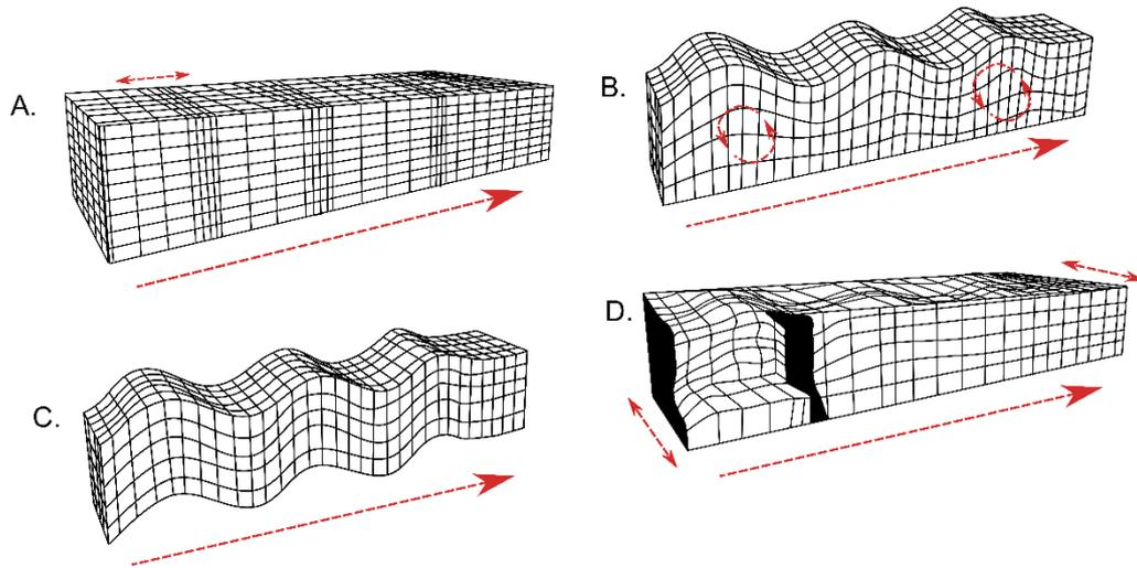
**Figure 1.3 Block diagram of types of waves in a 3D medium with propagation direction marked with arrows, compressional (A), Rayleigh (B), shear (C) and Love waves (D), redrawn and adapted from Aicher and Tautz (1990) and Peterie *et al.* (2014).**
