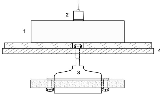
**Figure 4.8 Schematic of the geophone calibration setup, consisting of geophone system (1, uncalibrated), 4370 accelerometer (2), electromagnetic shaker (3), acrylic platform (4).**
