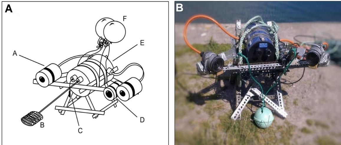
**Figure 3.2** Initial prototype consisting of an iron frame equipped with two stereoscopic cameras and a hydrophone connected to a central subsea housing. A. stereoscopic cameras, B. Bait bag, C. Hydrophone connected to DVR recorders for synchronization of video and sound, D. Bullet camera for live video feed, E. Subsea housing containing mini DVR recorders and power supplies (A); Photo of the initial BRUV prototype at Lough Hyne during trials (B).
