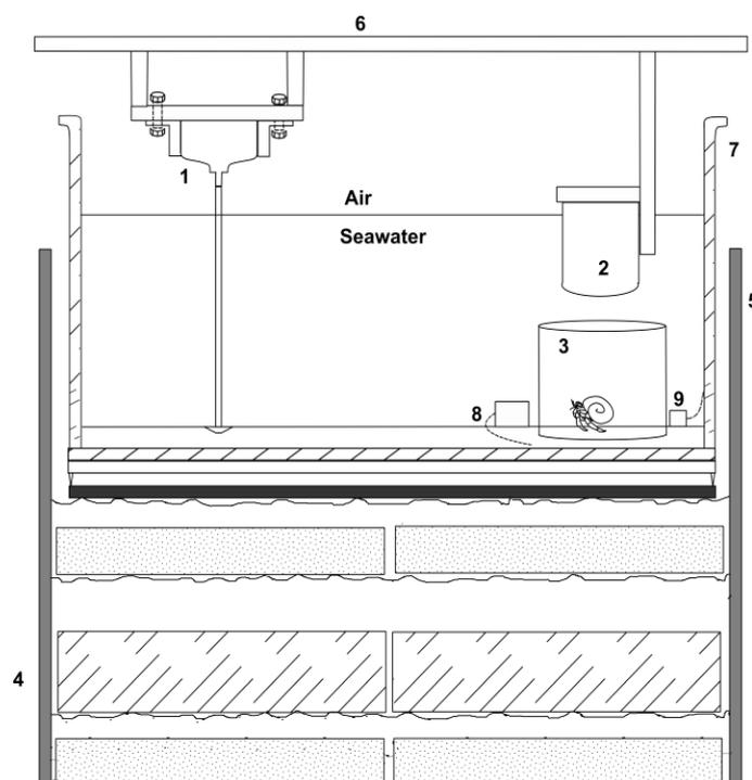
**Figure 4.1 Schematic of experimental setup, consisting of electromagnetic shaker and stinger rod (1), underwater camera (2), experimental arena (3), layered base made up of mixed hard and soft insulation and concrete (4), wooden support structure (5), steel frame separate from the base (6), experimental tank with needlepoint legs (7), position of geophone system (8), position of accelerometer (9).**
