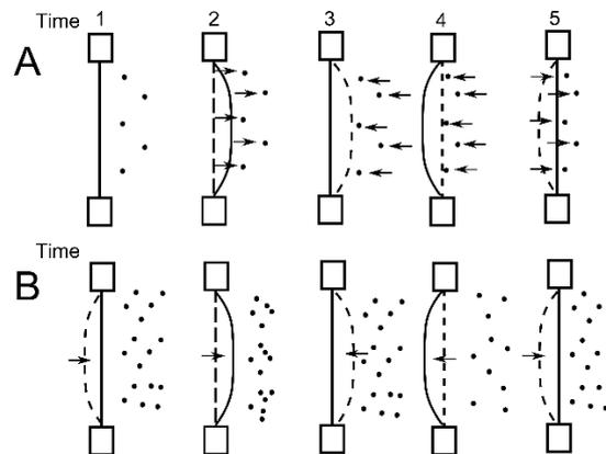
**Figure 1.1 A speaker membrane producing sound. Particle velocity component, displacement of fluid particles (A), pressure, compression of nearby fluid (B), figure redrawn from Breithaupt (2002).**
