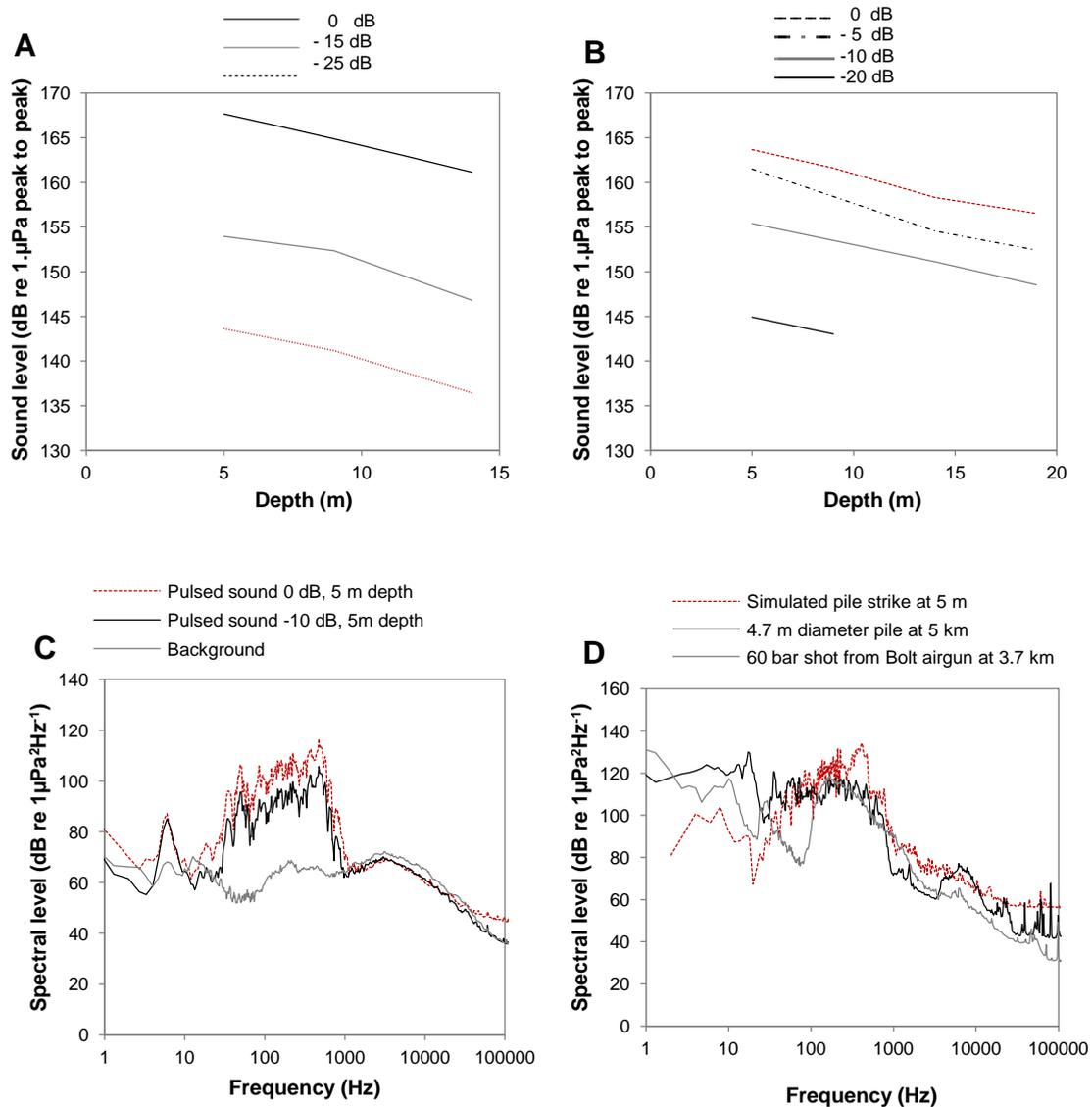
Figure 2.6 Sound pressure levels at different depths from the sound projector, 23<sup>rd</sup> October (A), 27<sup>th</sup> October (B). The sound at -20 dB on 27<sup>th</sup> was not distinguishable above background; The spectra of playbacks on 27<sup>th</sup> October (C); A comparison of playback to recordings of piling and airguns (D). Piling data reanalysed from (Nedwell *et al.*, 2007). Data courtesy of Subacoustech Ltd.
