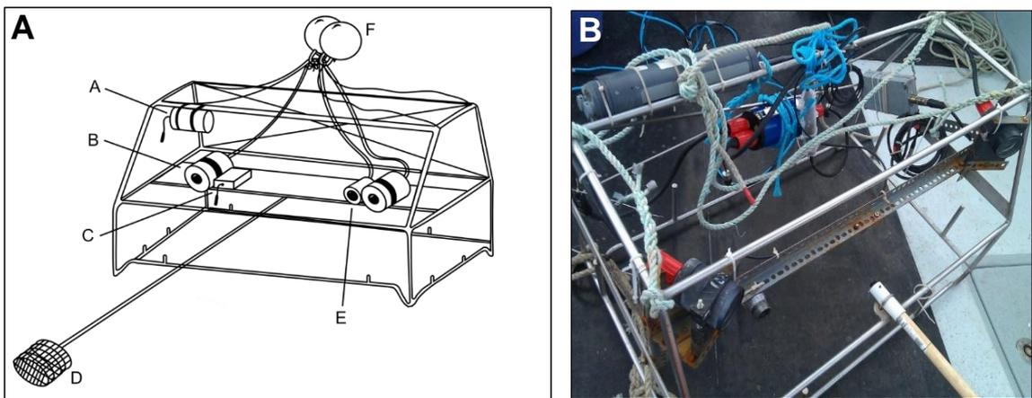
Figure 3.5 Third BRUV prototype (A), consisting of two stereoscopic cameras wired via an armoured umbilical cable to surface DVR recorders and power supplies. Two remote recording pods with hydrophones recorded sound levels. Letters as above except E. IP camera for live video link to surface, F. Subsurface buoy. Photo of Figure 3.5 on deck (B) during trials.
