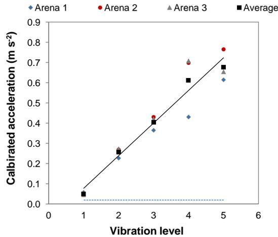
Figure 5.4 Average acceleration ( $\text{m s}^{-2}$ ) corresponding to levels of vibration (1 – 5), for each of the three arena (1 – 3), and average ( $\text{m s}^{-2}$ , RMS), data from February 2013. The lowest threshold of *M. edulis*, as found in Figure 5.7 is represented by a dotted line.
