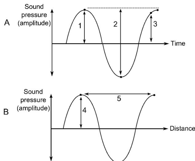
**Figure 1.2 The pressure variation of an acoustic wave over time and distance (A), the waveform showing the commonly measured features of the wave (B). 1. Peak, 2. Peak-to-peak, 3. Root mean square (RMS), 4. peak amplitude, 5. wavelength (adapted from OSPAR, 2009).**
