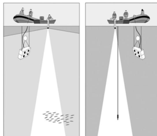
FIG. 1. A rigid-hull inflatable boat (RIB), with an outboard motor, and a small rowing boat were tethered together and allowed to drift without power. A sonar system was attached to the rowing boat to observe fish, and a sound projector array suspended from the RIB to transmit sounds.
