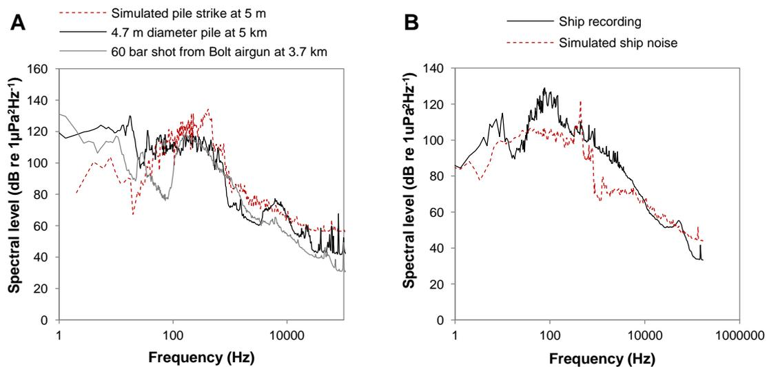
**Figure 3.8** A comparison of playback of synthetic impulsive sound from the sound projector array to recordings of pile driving and airguns, data from Subacoustech Ltd. Piling data reanalysed from Nedwell *et al.* (2007) (A); A comparison of playback of boat noise to the original recording of a large container ship, data courtesy of Subacoustech Ltd (B).
