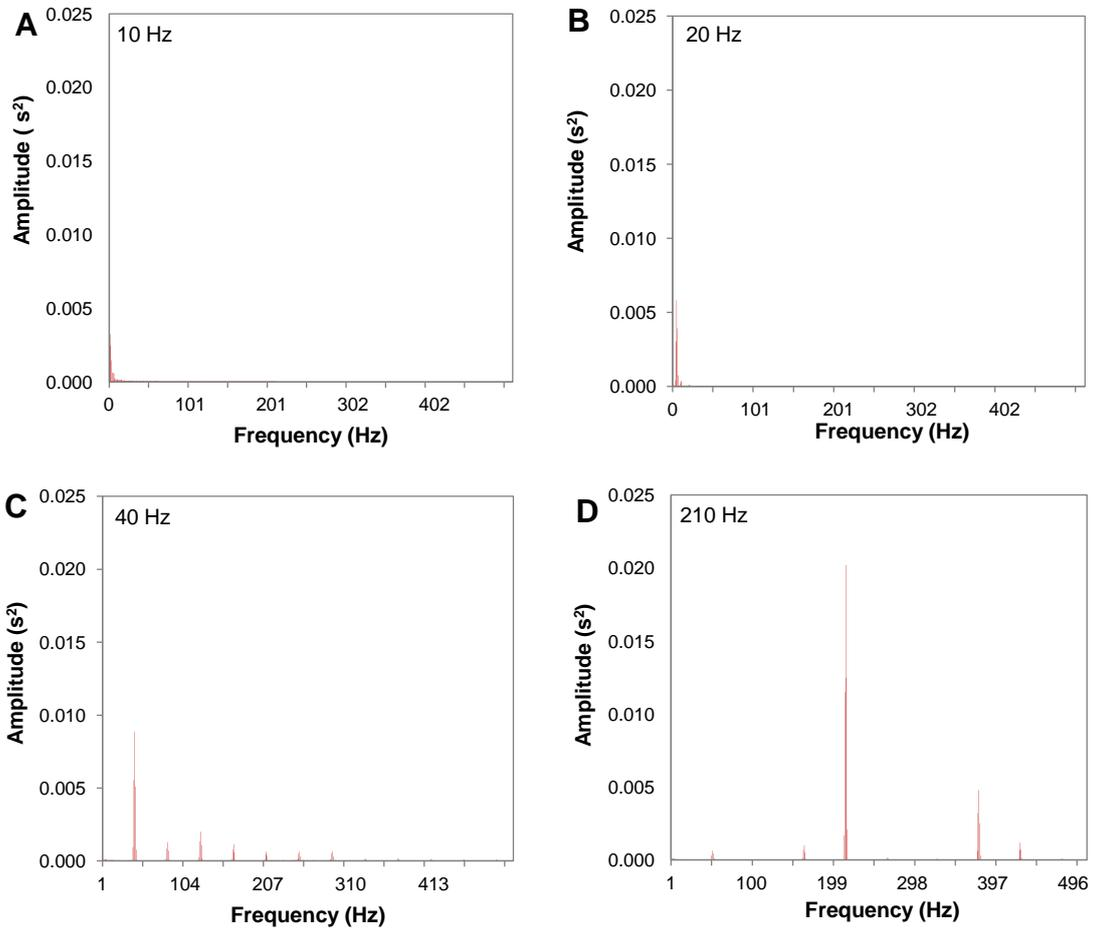
Figure 4.11 Example spectra of measured shaker signals from 8<sup>th</sup> and 9<sup>th</sup> December 2013, 10 Hz (A), 20 Hz (B), 40 Hz (C) with small resonant peaks, 210 Hz (D).
