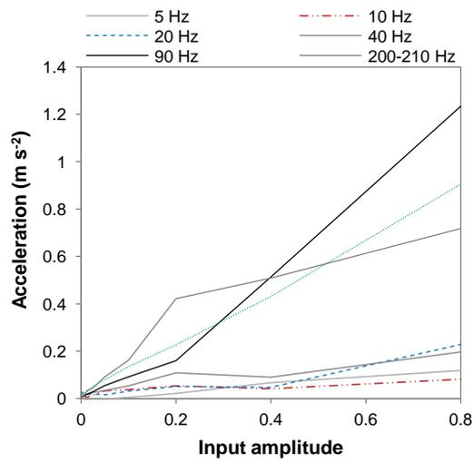
Figure 4.10 Dynamic range of the shaker excitation system ( $\text{m s}^{-2}$ ).
