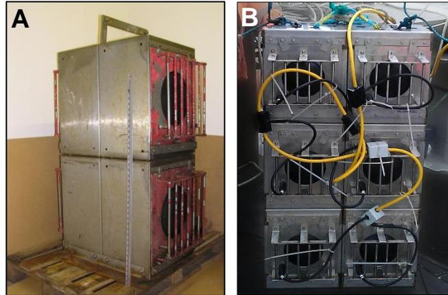
**Figure 3.1 Initial prototype sound projector array, consisting of two sound projectors, 150 kg, metre rule shown for scale (A); Final transducer array consisting of six units bolted together, 15 kg each (B).**
