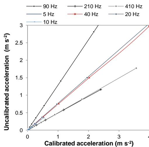
Figure 4.6. Calibration chart, as derived from calibration measurements, for the type 4333 Brüel & Kjær accelerometer used in the current work.
