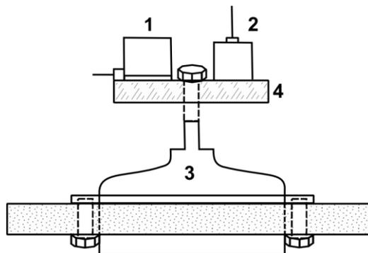
**Figure 4.5 Schematic of accelerometer calibration setup, consisting of Type 4333 accelerometer (uncalibrated, 1), 4370 accelerometer (2), electromagnetic shaker (3), acrylic platform (4).**
