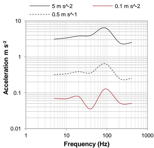
Figure 4.7 Frequency response chart for type 4333 Brüel & Kjær accelerometer (5 – 410 Hz), calibrated using a type 4370 Brüel & Kjær accelerometer. Three reference accelerations are provided.
