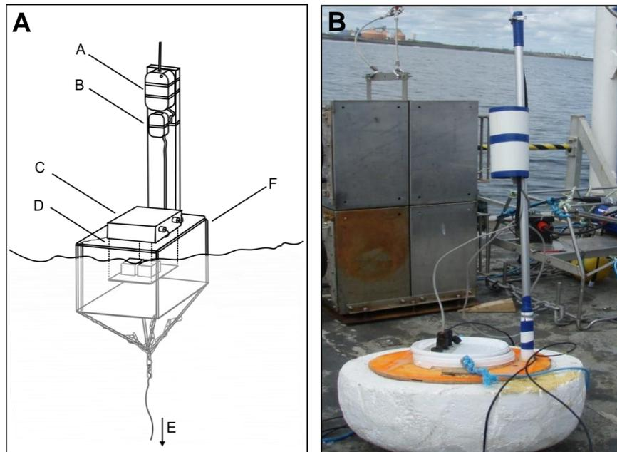
**Figure 3.3** Buoy built to transmit a live IP camera signal remotely to the boat (A), consisting of power supply and waterproof wireless router. A. Wireless router, B. Power supply, C. Pelicase containing wiring, D. Battery supplies held inside the buoy, E. Umbilical cable attached to the BRUV on the seabed, F. Slotted steel frame containing polystyrene cube; Photo of the final prototype of the buoy, after rounding of corners (B).
