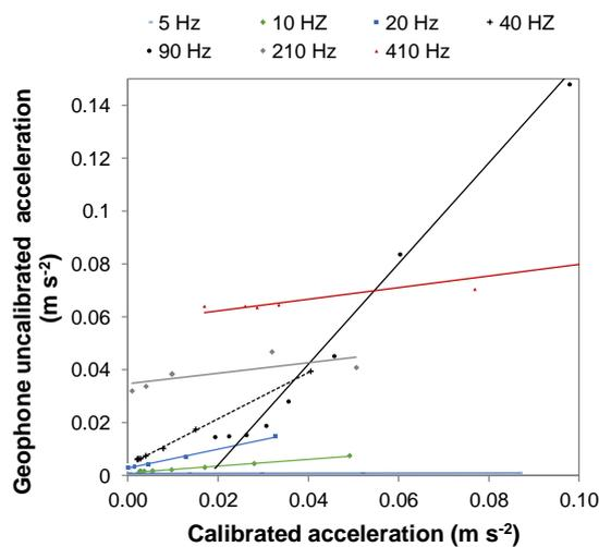
**Figure 4.9 Calibration chart for the vertical axis of the geophone system (SM-7 375 ohm, IO, sensitivity 28.8 V m s<sup>-1</sup>).**
