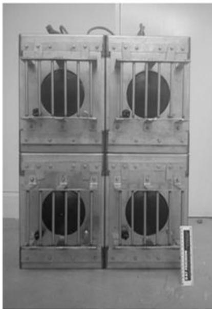
FIG. 2. The array of underwater sound projectors used for the playback of synthetic piling noise, with a 15 cm long ruler shown for scale.
