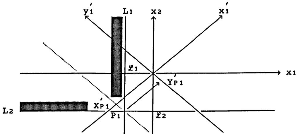
Fig[4.2] Condition for a positive slope (up-crossing) of level zero in time interval  $\Delta t_1$ .
