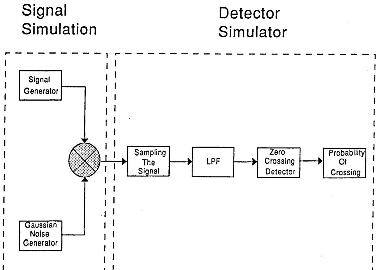
Fig[7.1] Block diagram of experimental set up.
