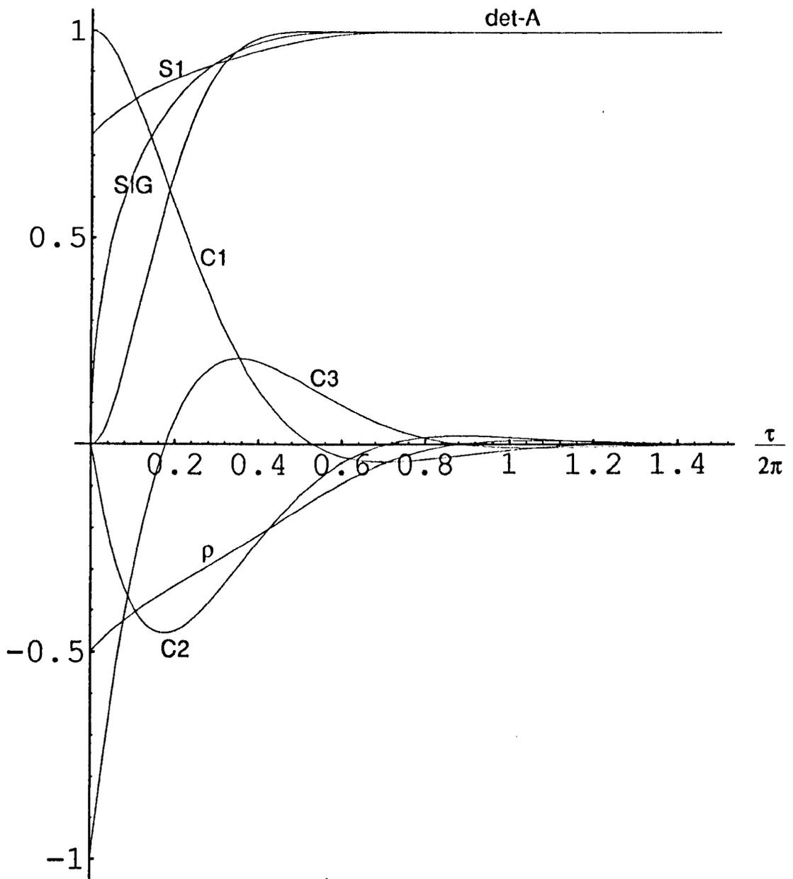
Fig[5.1] Normalised coefficient for Butterworth filter.
