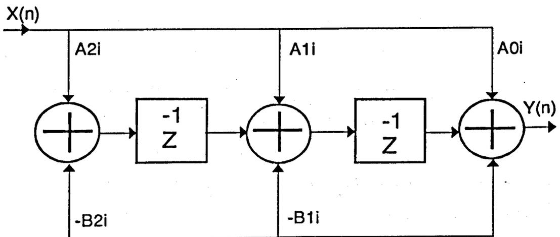
Fig[7.2] Structure of a biquad elements for use in implementing IIR filter.
