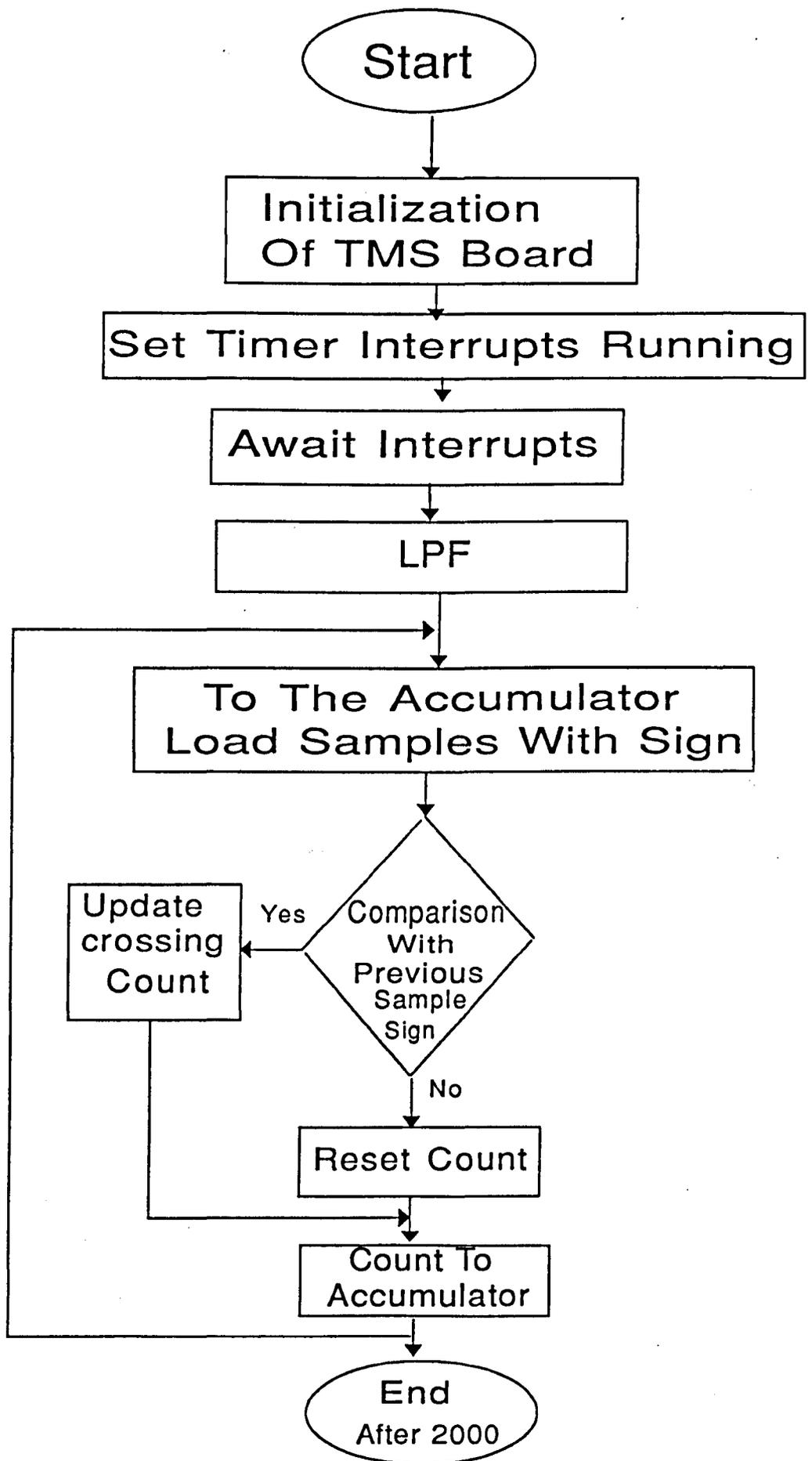
Fig[7.3] Zero Crossing detector flow diagram.
