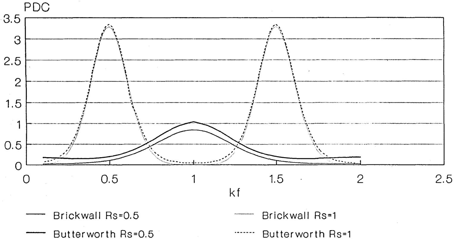
Fig[5.6c] PDC for SNR=1, for the case of no correlation with same time scaling.
