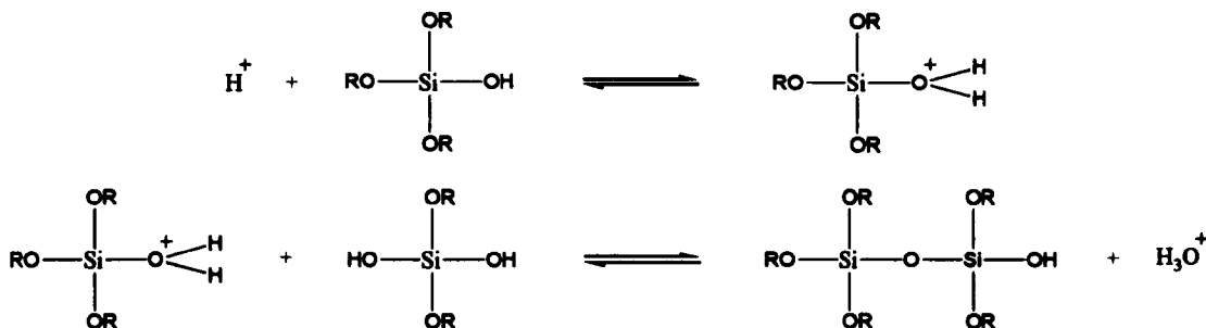
Figure 1.13: Proposed mechanism for acid condensation of silica sol-gels.
