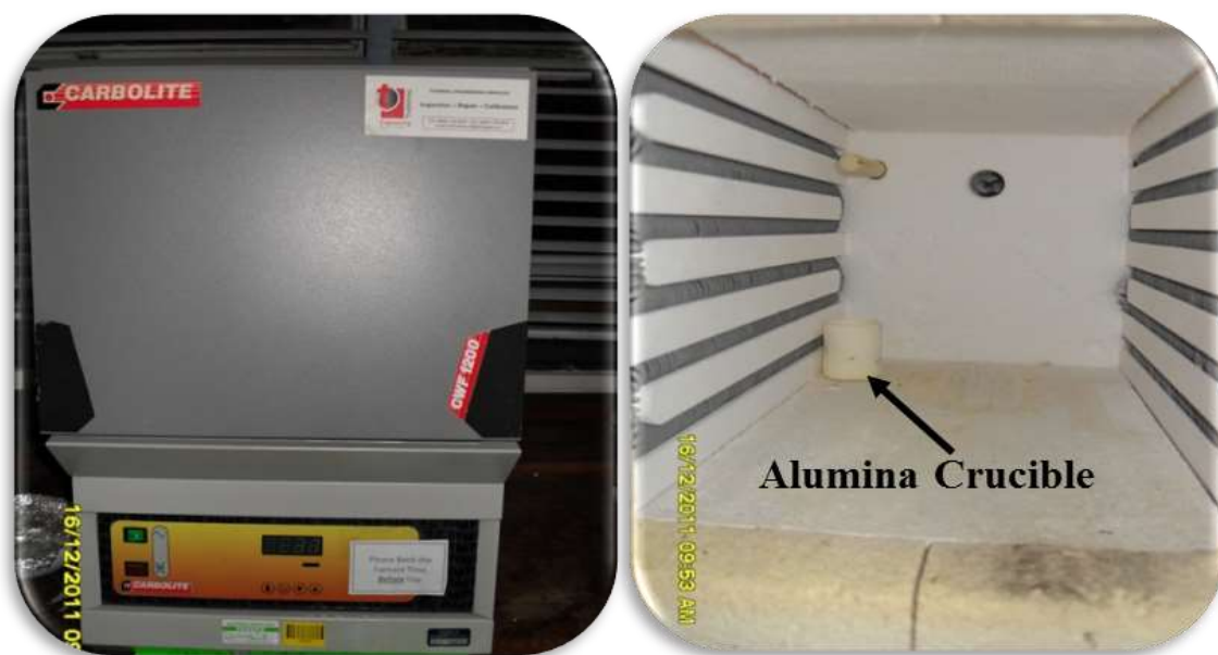
Figure 2- 1: The interior and exterior of the box furnace used in this project.
