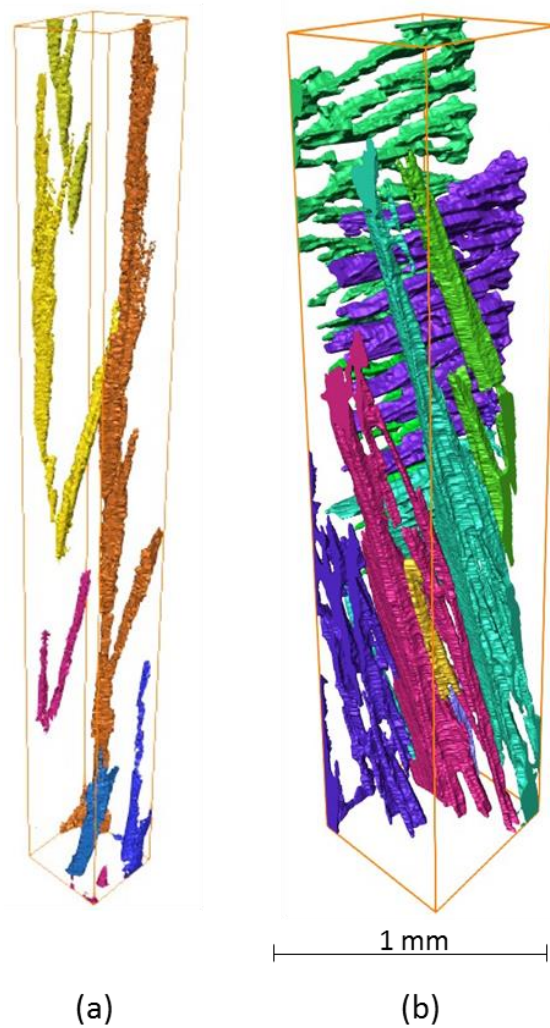
Fig. 5.21. The 3-D primary \theta phases of Al-35Cu samples (by segmenting out the rest of the matrix) cast (a) without EMP; and (b) with EMP of 1Hz, 120 V. The X-ray images taken from lab based X-ray CT scan.
