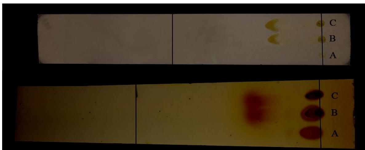
**Figure 7-9: Comparison of the chromatographic separation for (top) the silicon diimide gel TLC plate and (bottom) the reference silica gel TLC plate.**
