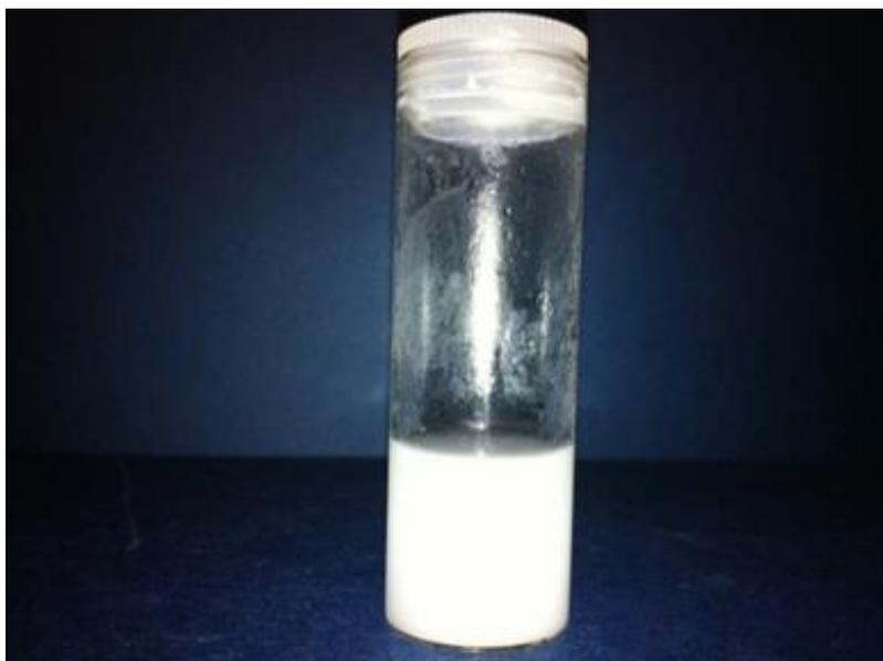
**Figure 3-5: Aqueous colloidal suspension of CMC-stabilised SMS039 B, prepared in the presence of 0.5% CMC, at  $\text{pH} = 2$ .**
