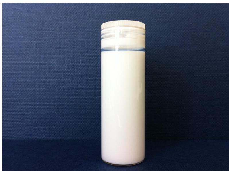
**Figure 4-5: Stable aqueous colloidal solution of TiO<sub>2</sub> rutile after standing one month prepared by method 3.**
