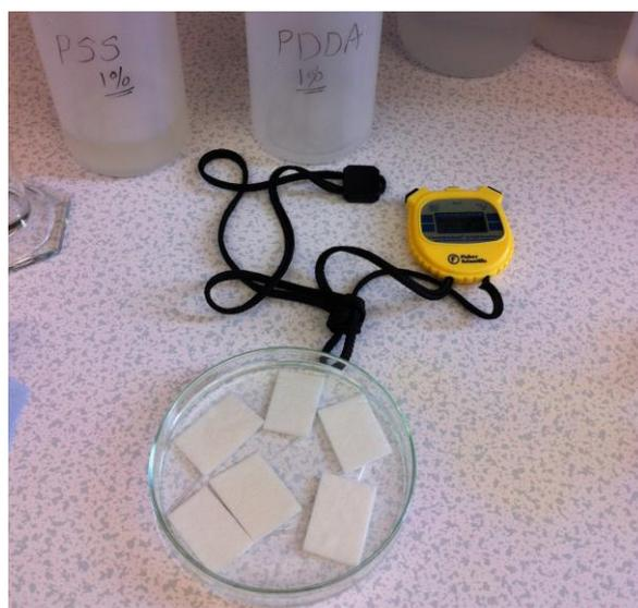
**Figure 5-13: Coating process for LBL paper with PDDA, PSS and then PDDA.**
