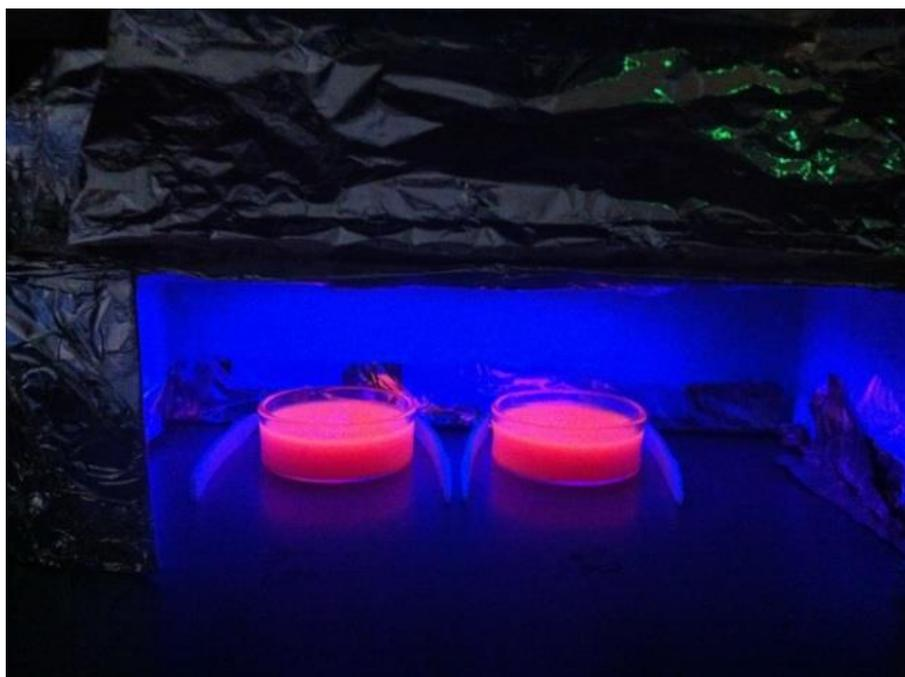
**Figure 6-12: mixture of TiO<sub>2</sub>/APTES and Rhodamine B samples observed under illumination with UV light.**
