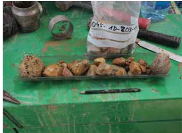
**Figure 8.** Rounded gravel and pebbles in core catcher material (DEEP site, hole 1D at 569 m b.l.f.) indicate fluvial transportation.
