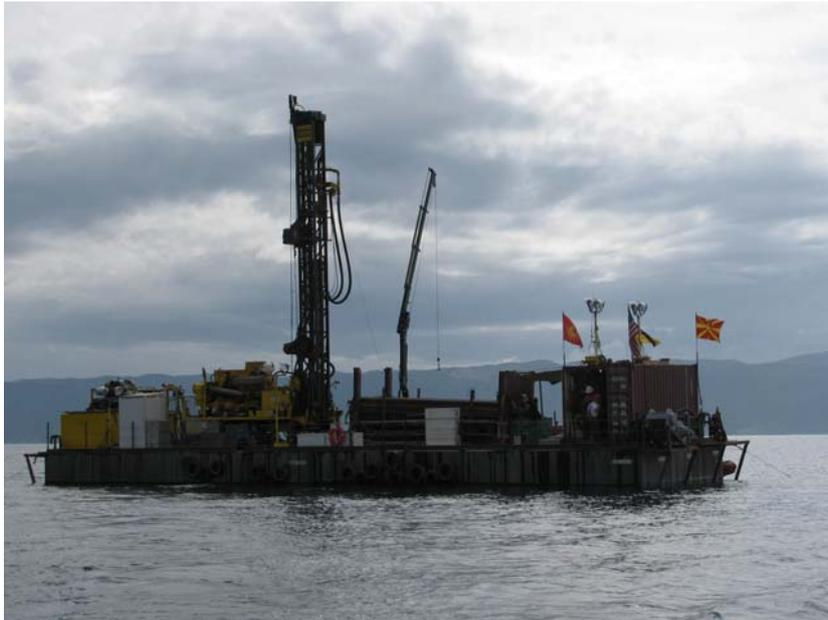
**Fig. 3.1** The barge of the Deep Lake Drilling System, DOSECC.
