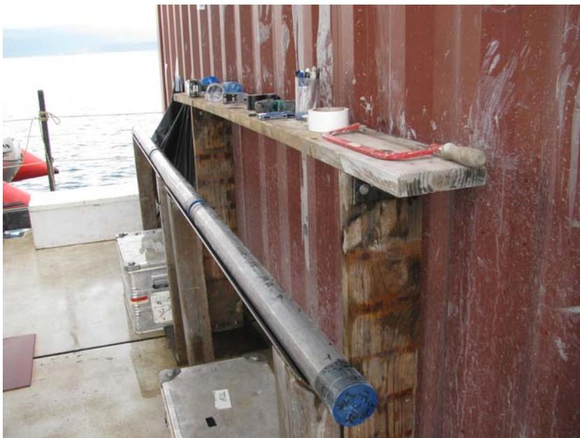
**Fig. 3.2** The core cutting facilities on the barge.
