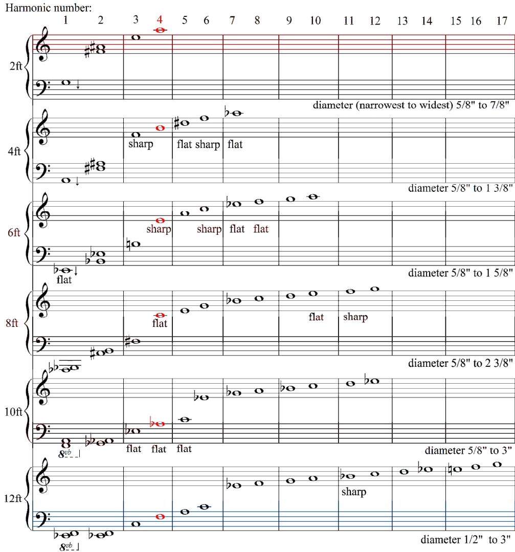
App. 1 Fig. 2. Harmonics of a conical tube (lengths of carbon-fibre alphorn) of different lengths.
