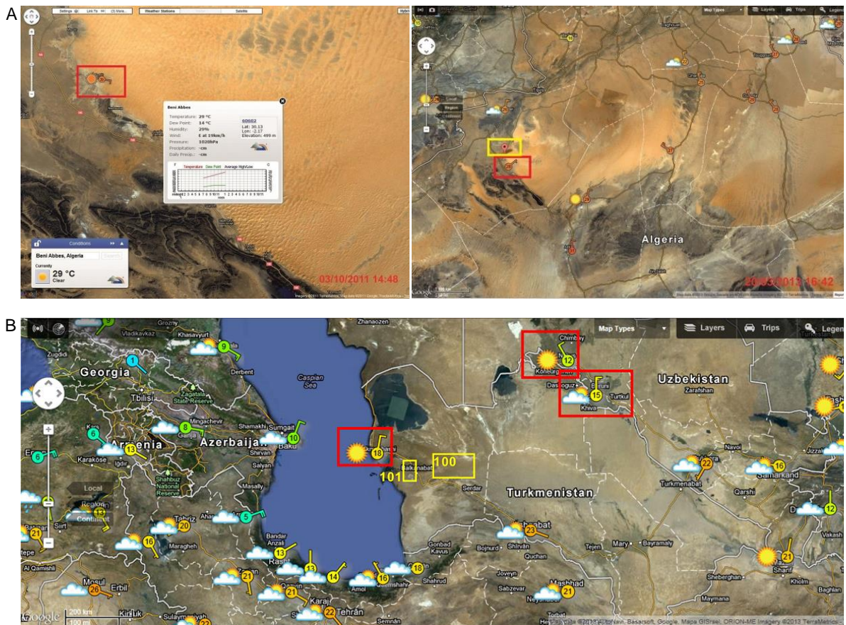
Figure 3-2 Identification of wind direction by referring to meteorological station records. Study sites are circled in yellow rectangles and stations that have been referred to are circled in red rectangles. A) Igli, Algeria (30°31'05.99" N 2°19'48.04" W). The meteorological records had been referred from nearby station and been accessed on 3rd October, 2011 and 20th March, 2013, separately; B) Two sites in Turkmenistan (39°42'51.53" N 55°33'35.18" E and 39°37'31.05"N 54° 9'55.13"E). Three meteorological stations records had been compared. (data source: weatherunderground.com).
