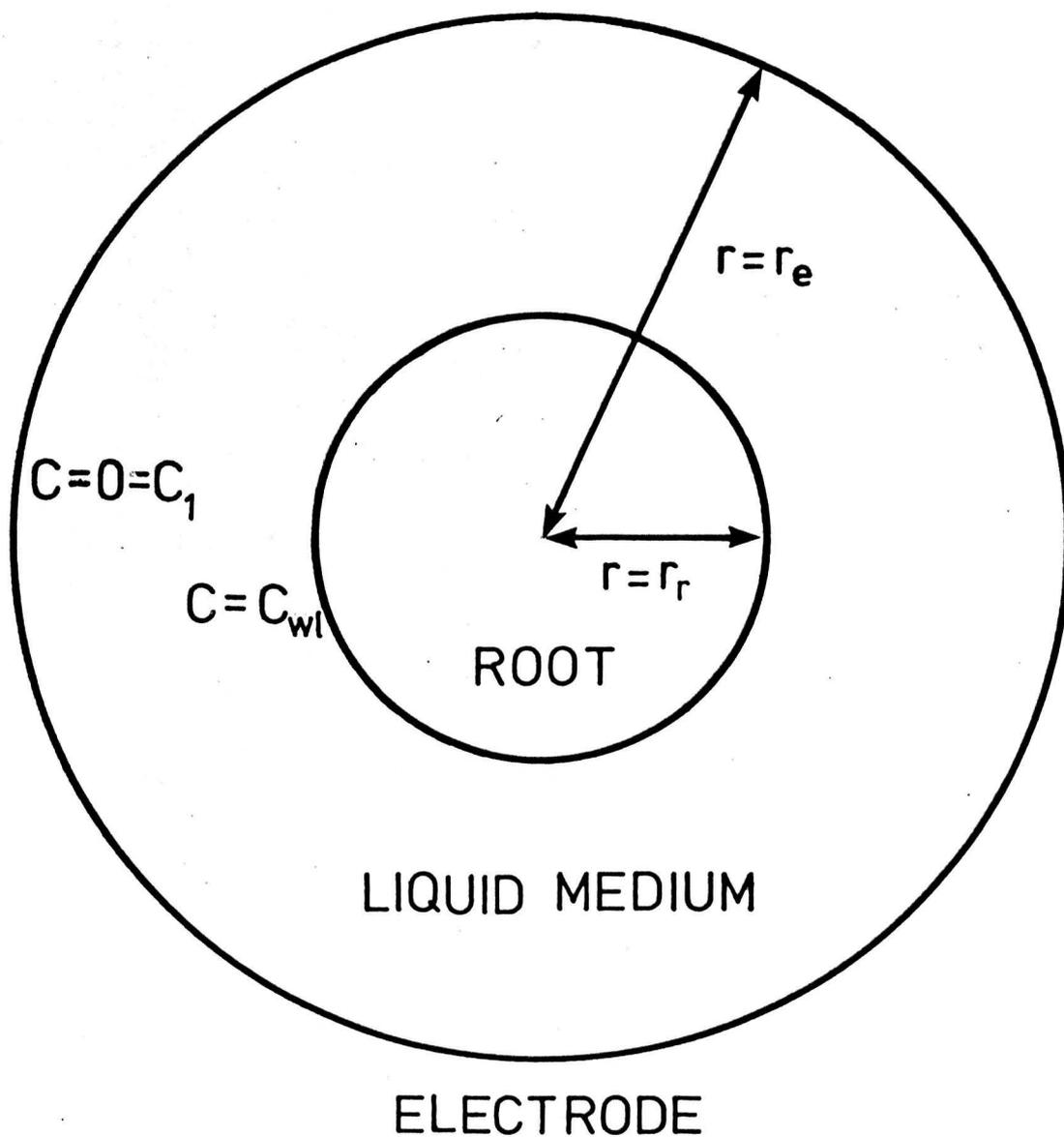
FIG. 2.3 Oxygen diffusion from a root to a cylindrical Pt electrode.
