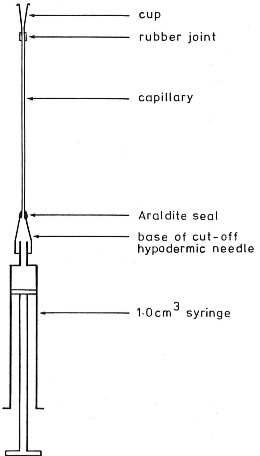
FIG. 4.6 Gas analyser (actual size)
