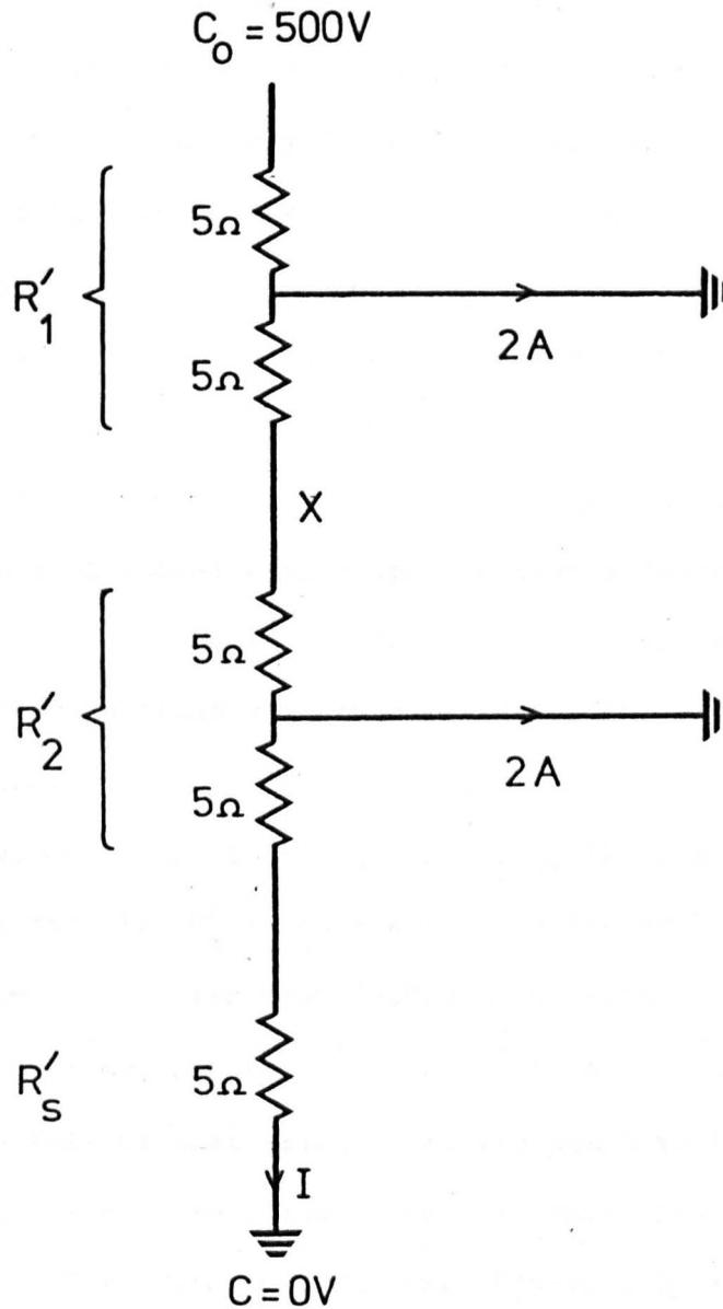
FIG. 7.3 Circuit to illustrate the effective resistance of a plant segment excised and in situ
