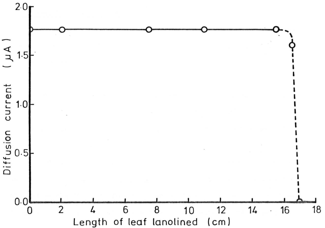
FIG. 6.4 Effect of lanolining on oxygen diffusion current. Single-leaf preparation, lanolined from apex to base. Leaf length 26.5 cm, submerged to sheath level (9.5 cm)
