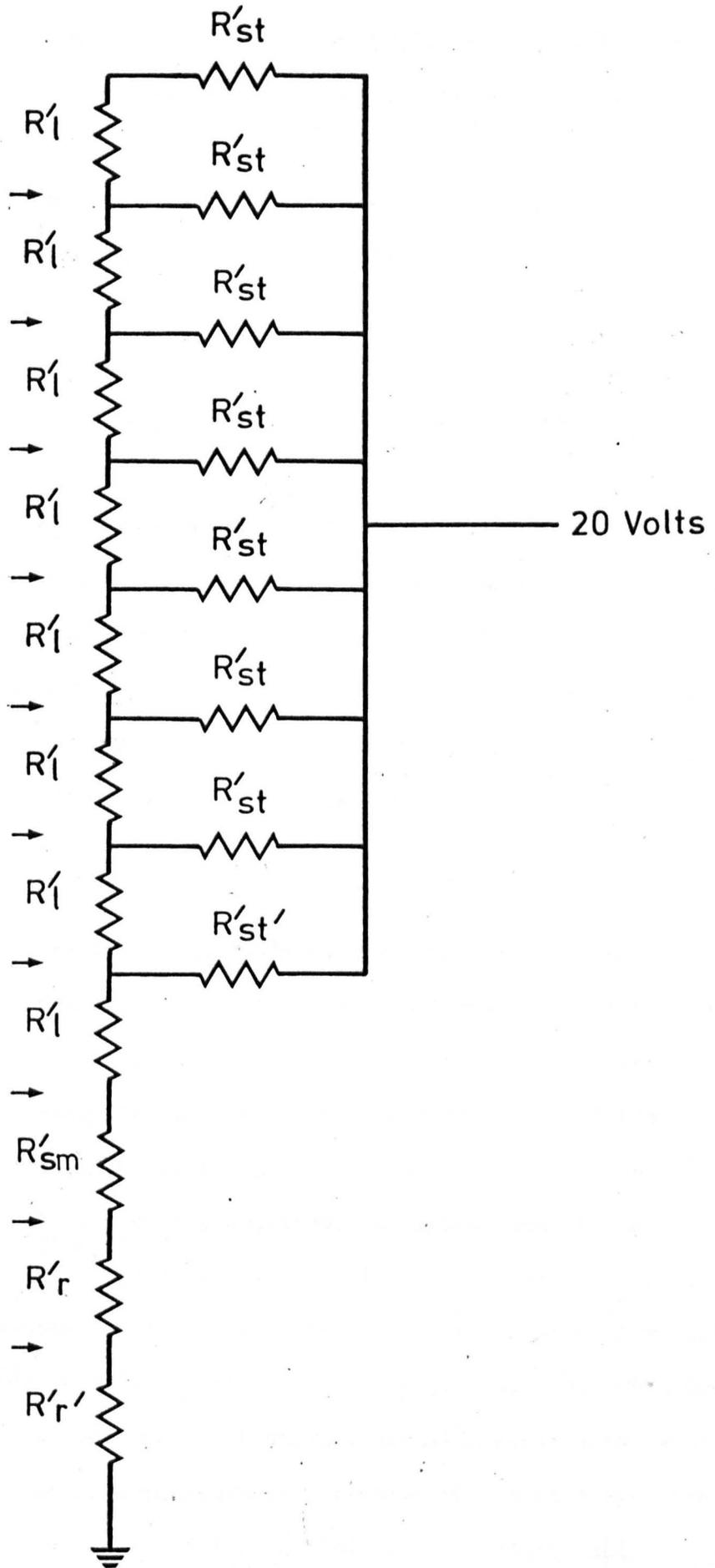
the calculations; in the "unsealed" condition the atmospheric potential is applied to the non-stomatal resistor currently at the top of the series, as well as to the stomatal resistors so long as these remained.
