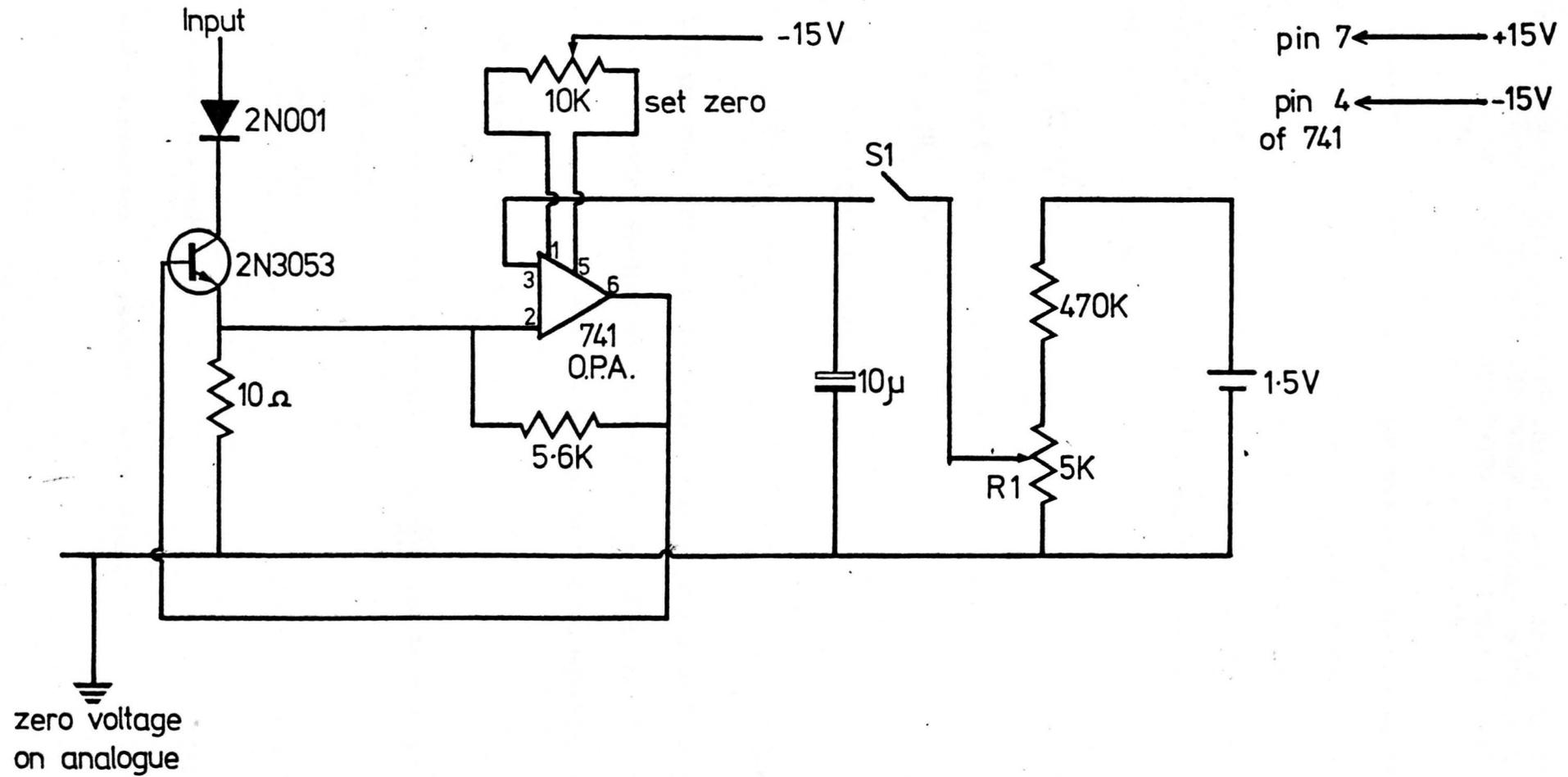
FIG. A3.2 Electrical analogue : additional circuit details . Constant current device
