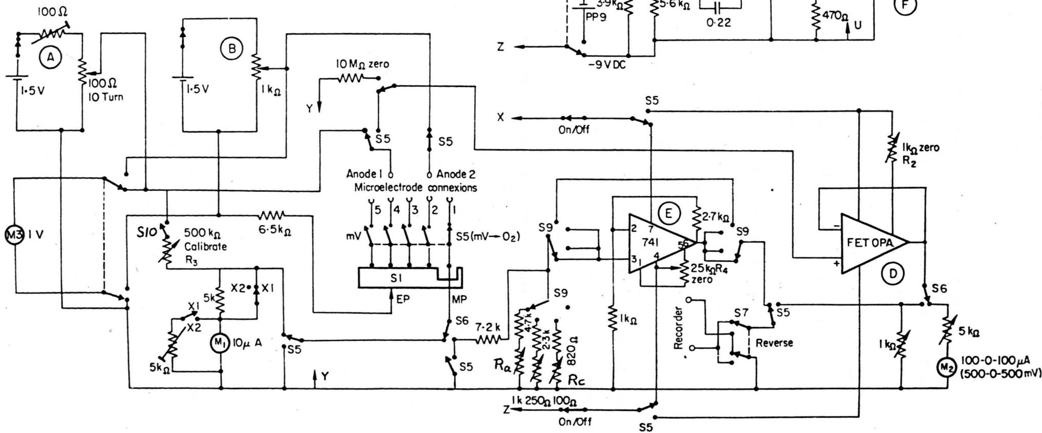
Circuit unit (E) is an amplifier which enables current in (A) to be displayed on a chart recorder (Goerz "Multiscript 3"). The instrument has a six-centimetre scale graduated 0-50 $\mu$ A. The amplifier provides three further scales of 0-5, 0-10 and 0-25 $\mu$ A, which may be selected using S9. (The 0-5 and 0-10 $\mu$ A ranges were most suitable for the measurements made in the present study).
