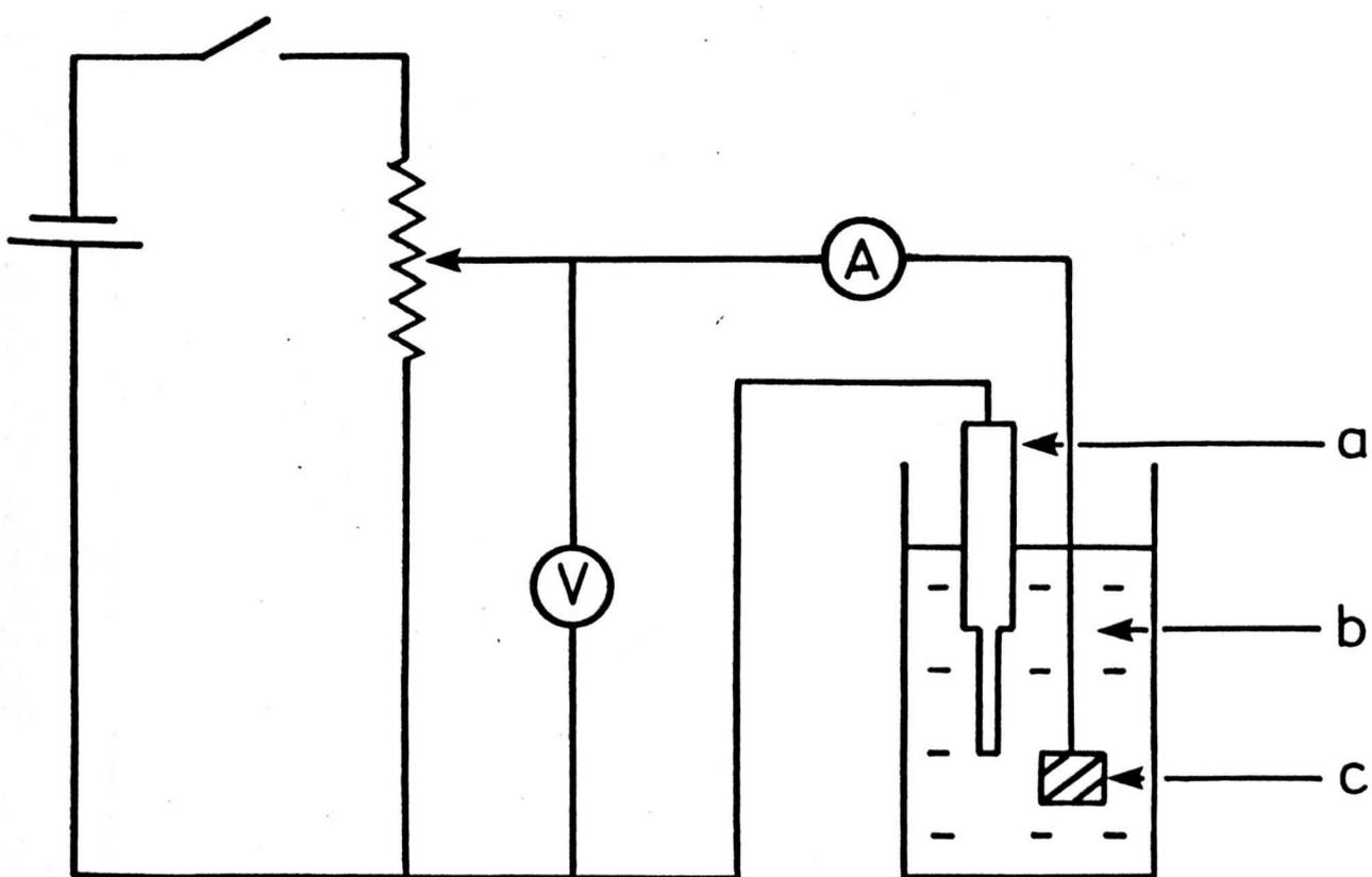
FIG. 2.1 Basic circuit for polarographic determination of dissolved oxygen.
