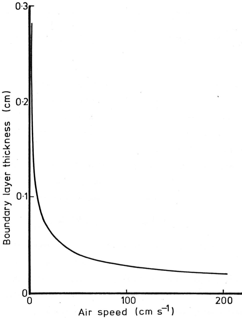
FIG. 6.14 Variation in boundary layer thickness with air speed for a leaf of width 0.5cm.
