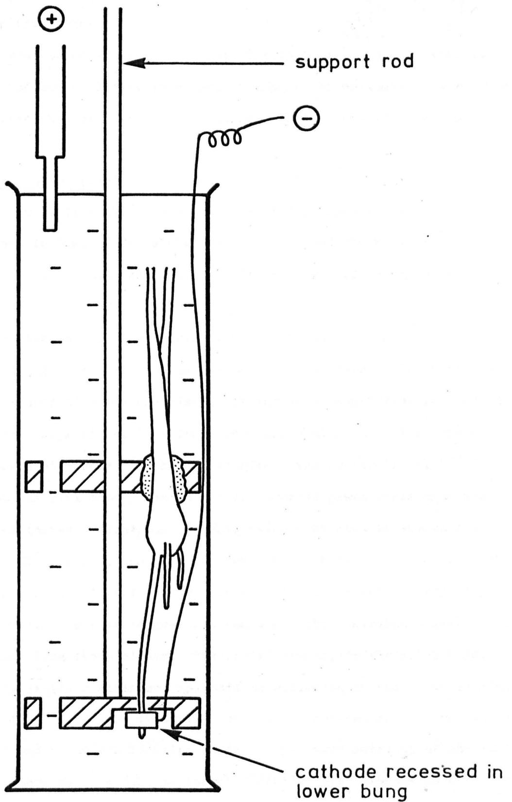
FIG.7.4 Apparatus used in diffusional resistance experiments.
