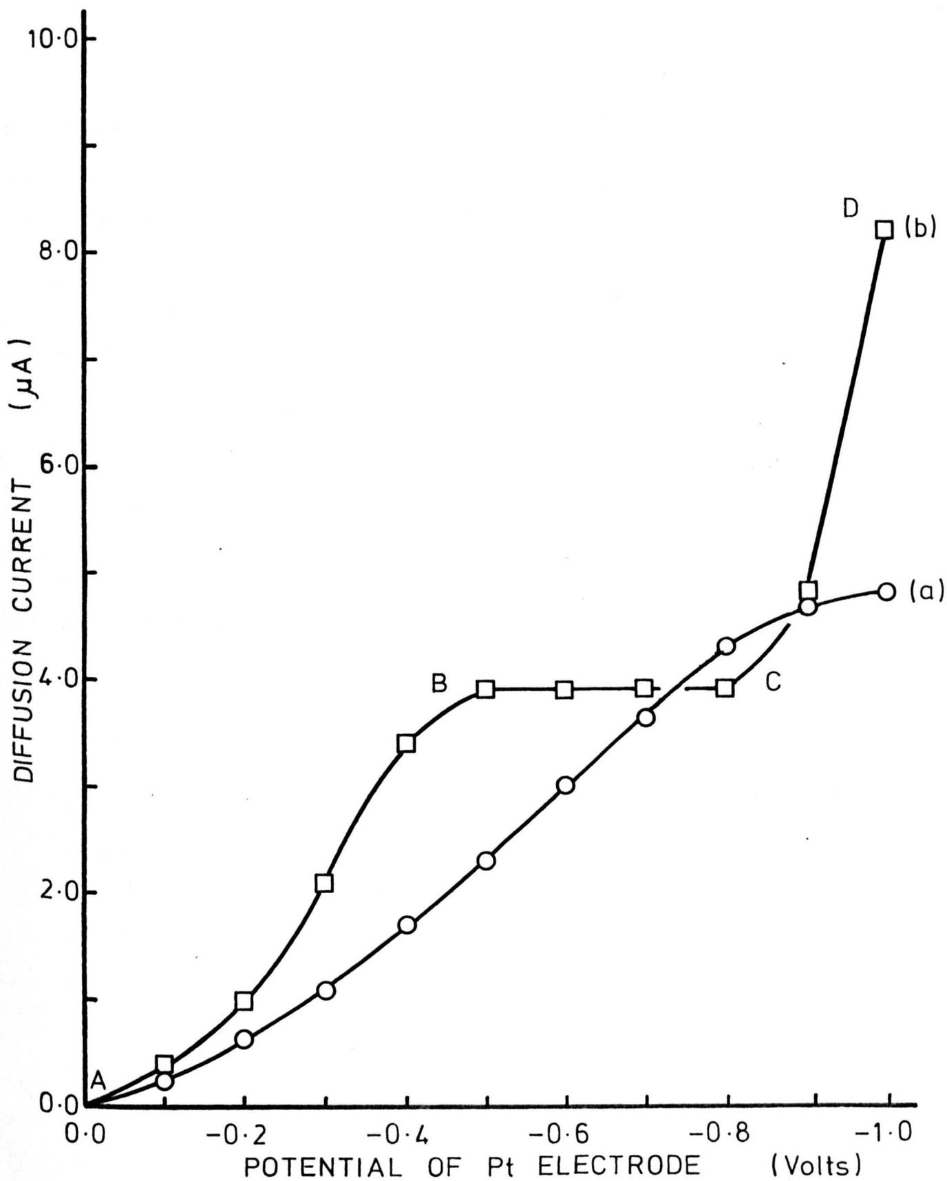
FIG. 2.2 Current-Voltage curves for air-saturated water at 23°C
