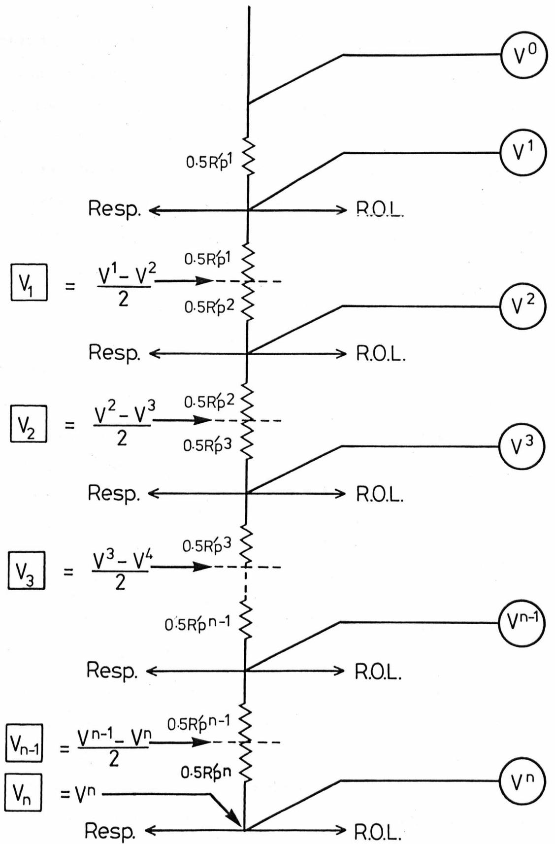
devices to replace the simple variable resistors,  $R'_R$ ; circuit details are given in Appendix 3. These devices allowed the desired respiration rate, once programmed, to remain independent of internal oxygen concentration until a pre-set value was reached, or until the oxygen concentration fell below that required for the efficient operation of the instruments (0.3 - 0.4%). The constant current devices also facilitated respiratory programming along the length of the root.
