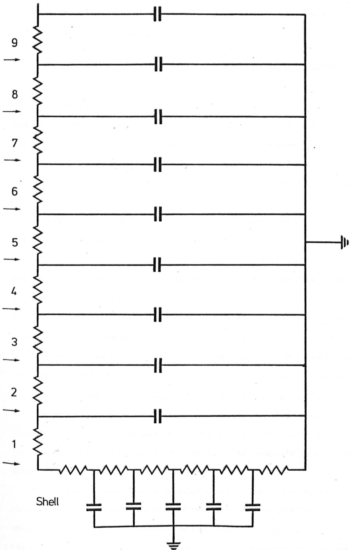
40V supply; after disconnection the capacitors discharged their "oxygen" to the respiratory devices and through the liquid shell. During this time the R.O.L. and the oxygen concentration at various points were monitored on a twin-channel recorder.
