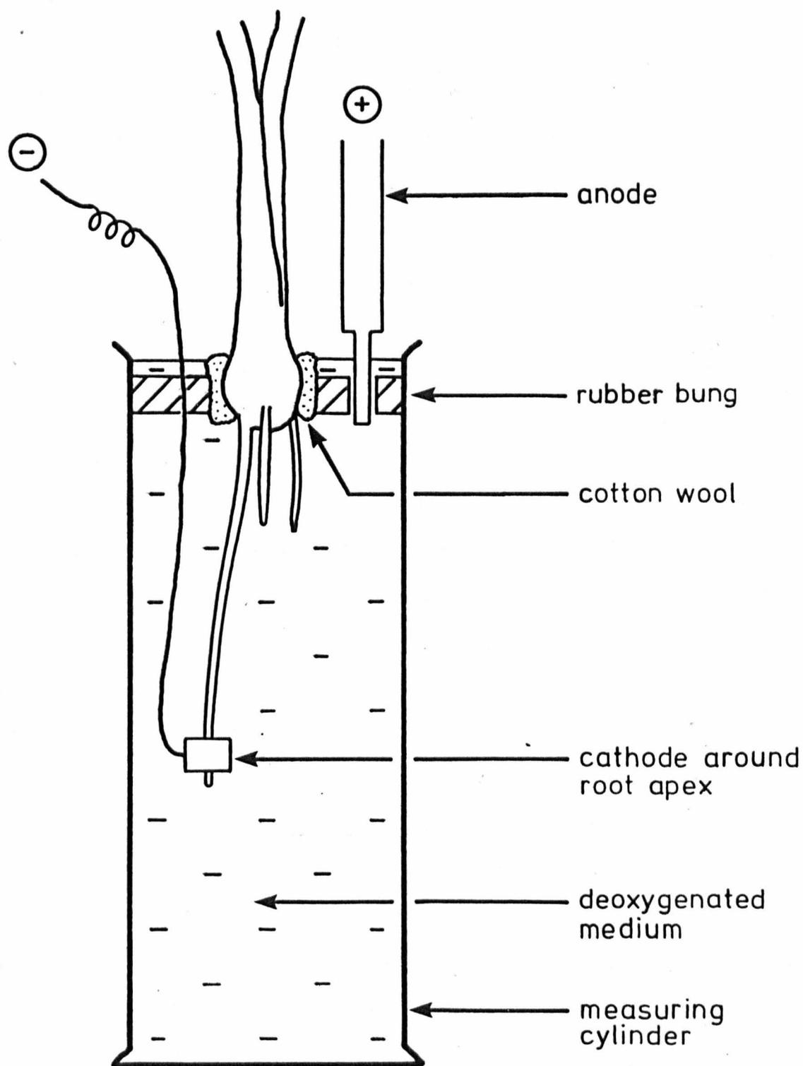
FIG. 2.5 Basic experimental assembly for the measurement of radial oxygen loss from roots .
