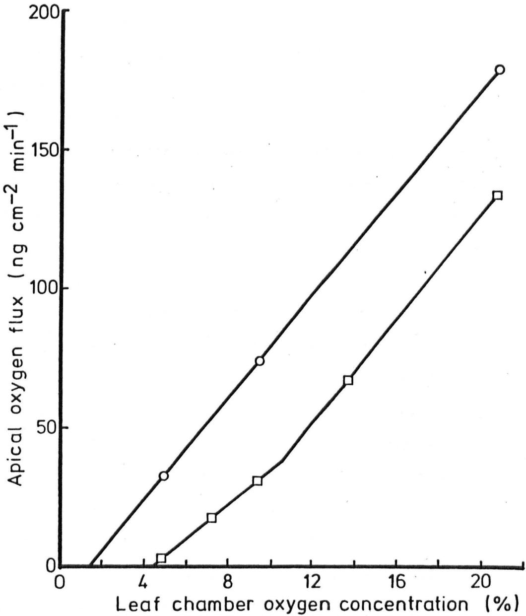
FIG. 4.2 Experimental relationships found between leaf chamber oxygen concentration and oxygen flux from the apex of a rice root at 3°C (○) and 23°C (□)
