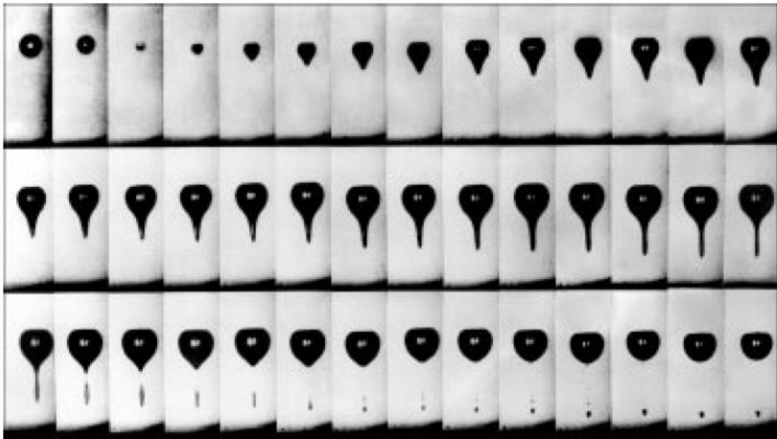
Fig. 2.11. The microjet of a laser-generated spherical bubble in water in the vicinity of a plane solid boundary at the bottom, observed at 300, 000 fps. The frame size is 6.7 \times 2.7 \text{ mm}^2 [78].
