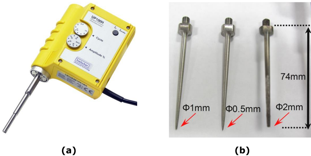
Fig. 3.16. (a) A photo of the UP100H ultrasound processor (from Hielscher Ultrasonics GmbH) used in the experiments, and (b) the sonotrode with 0.5 mm, 1 mm, and 2 mm tip diameters.
