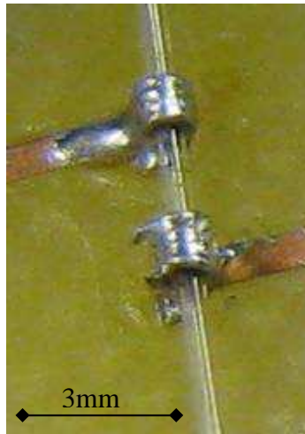
Figure 4.4: Wire wrapping electrode cell
