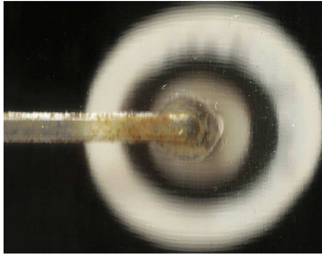
Figure 6.6: LOC channel showing blockage deposits from river water
