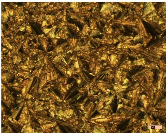
**Fig. 4.18** The Smectic A mesophase of compound **54** using OPM, on cooling, at 171 °C
