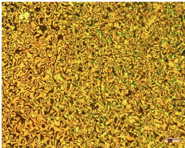
**Fig. 1.25** A typical nematic Schlieren texture (Compound **46** on cooling at 130 °C)
