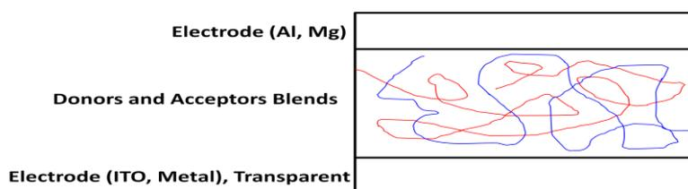
**Fig. 1.29** A simplified device of OPV cells for polymeric blends
