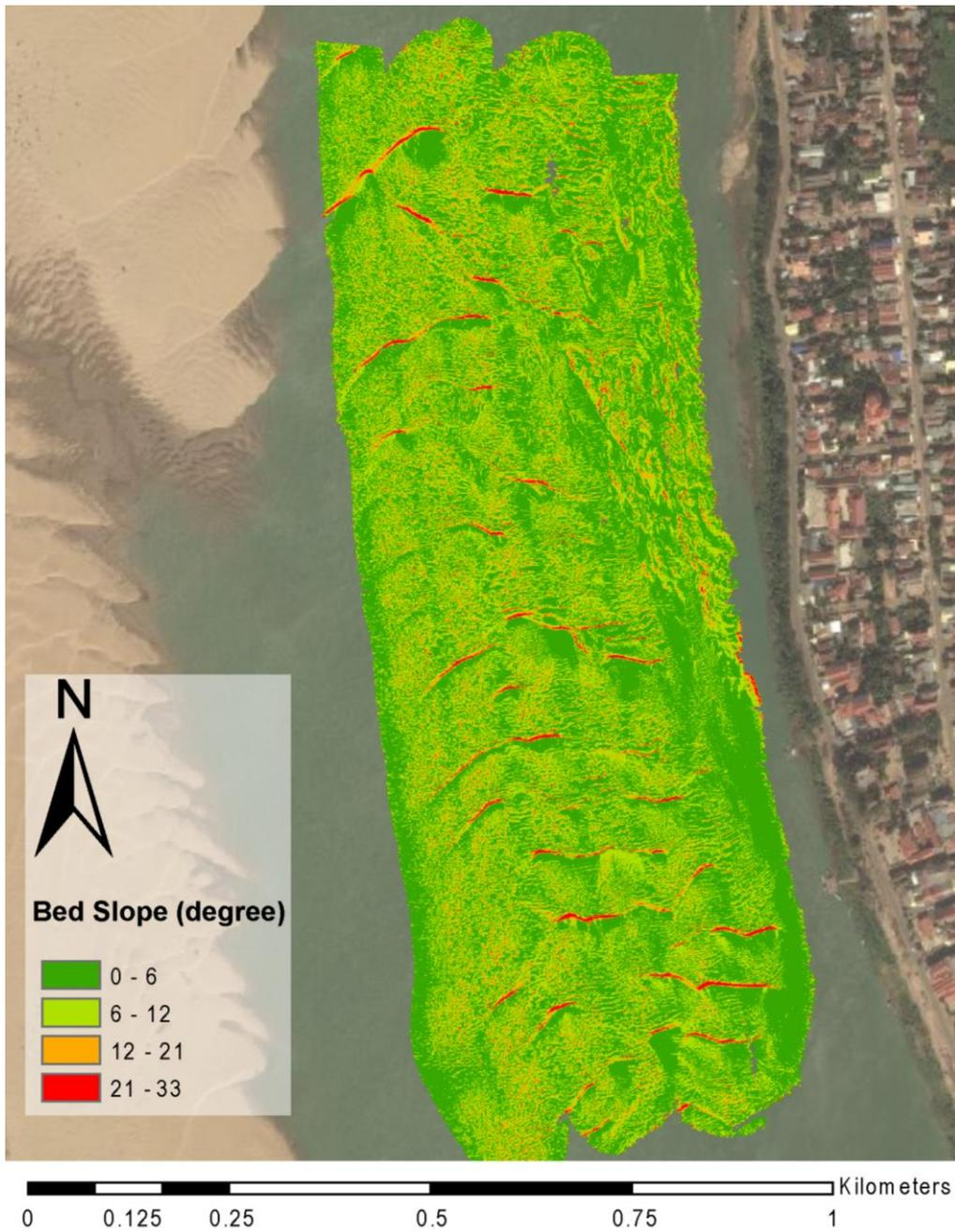
Figure 6-6. Local bed slope measured in degrees of the MBES bathymetry in Figure 6-5.
