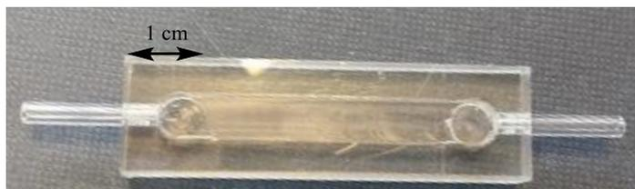
**Figure 2.3: Macrofluidic device that can be integrated with an electrode.**
