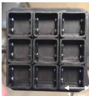
**Figure 3.1: A 3 x 3 array holder for 1 x 1 cm squared chips.**
