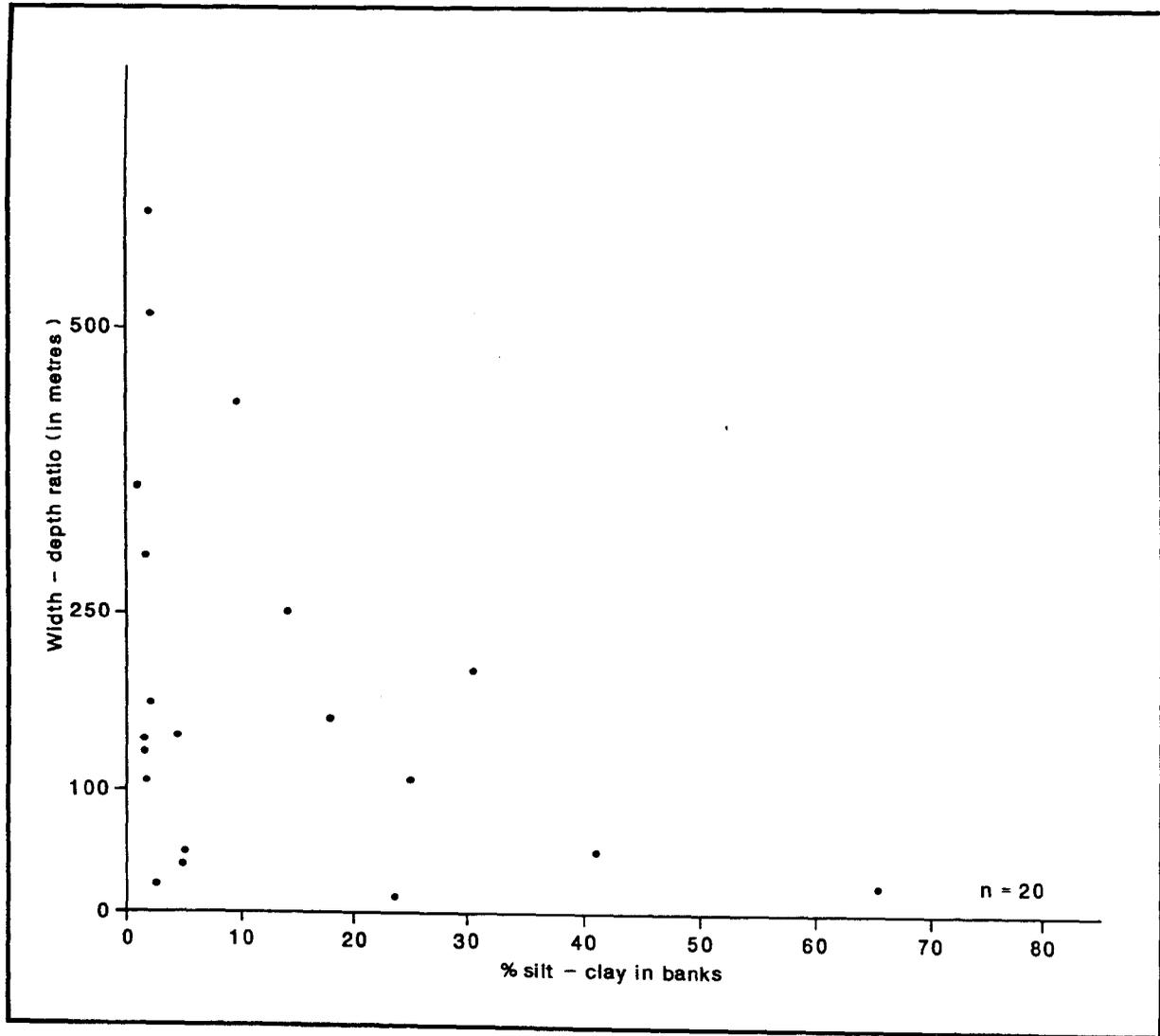
**Plot of % silt - clay in banks against width - depth ratio for a sample of 20 gravel-bed rivers - data from Mosley, unpublished.**
