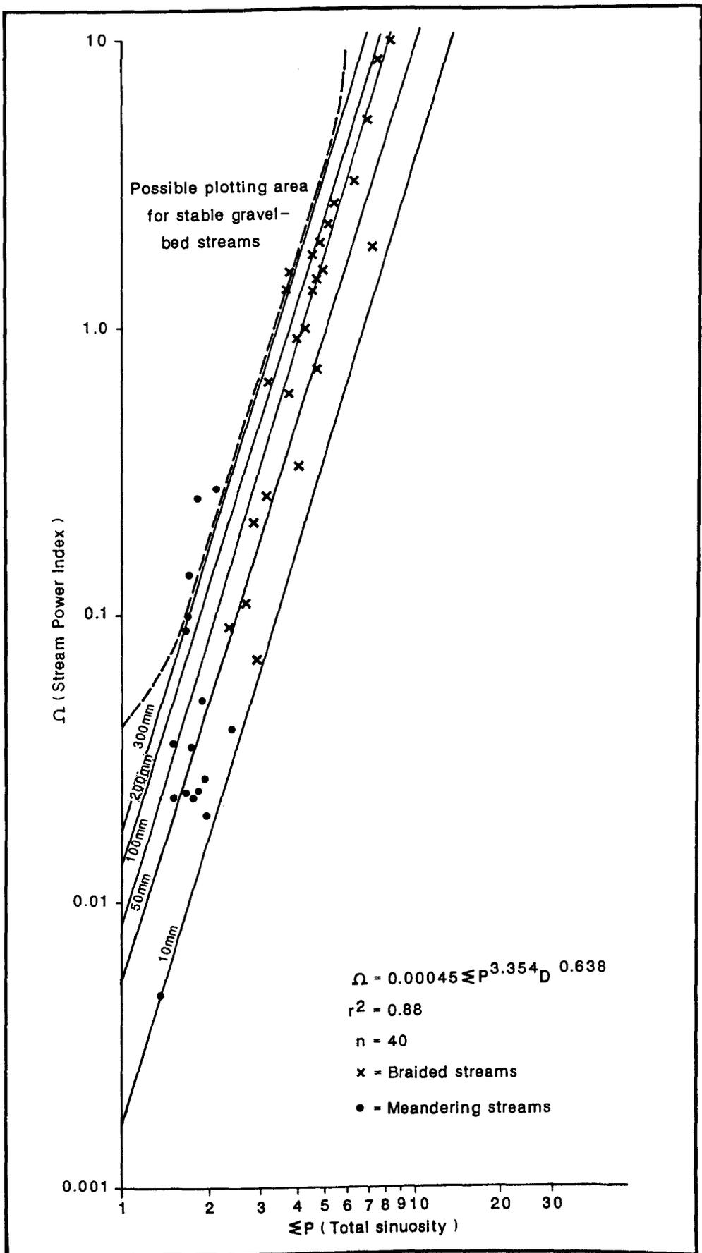
**Stream power plotted as a function of stream total sinuosity and grain - size**
