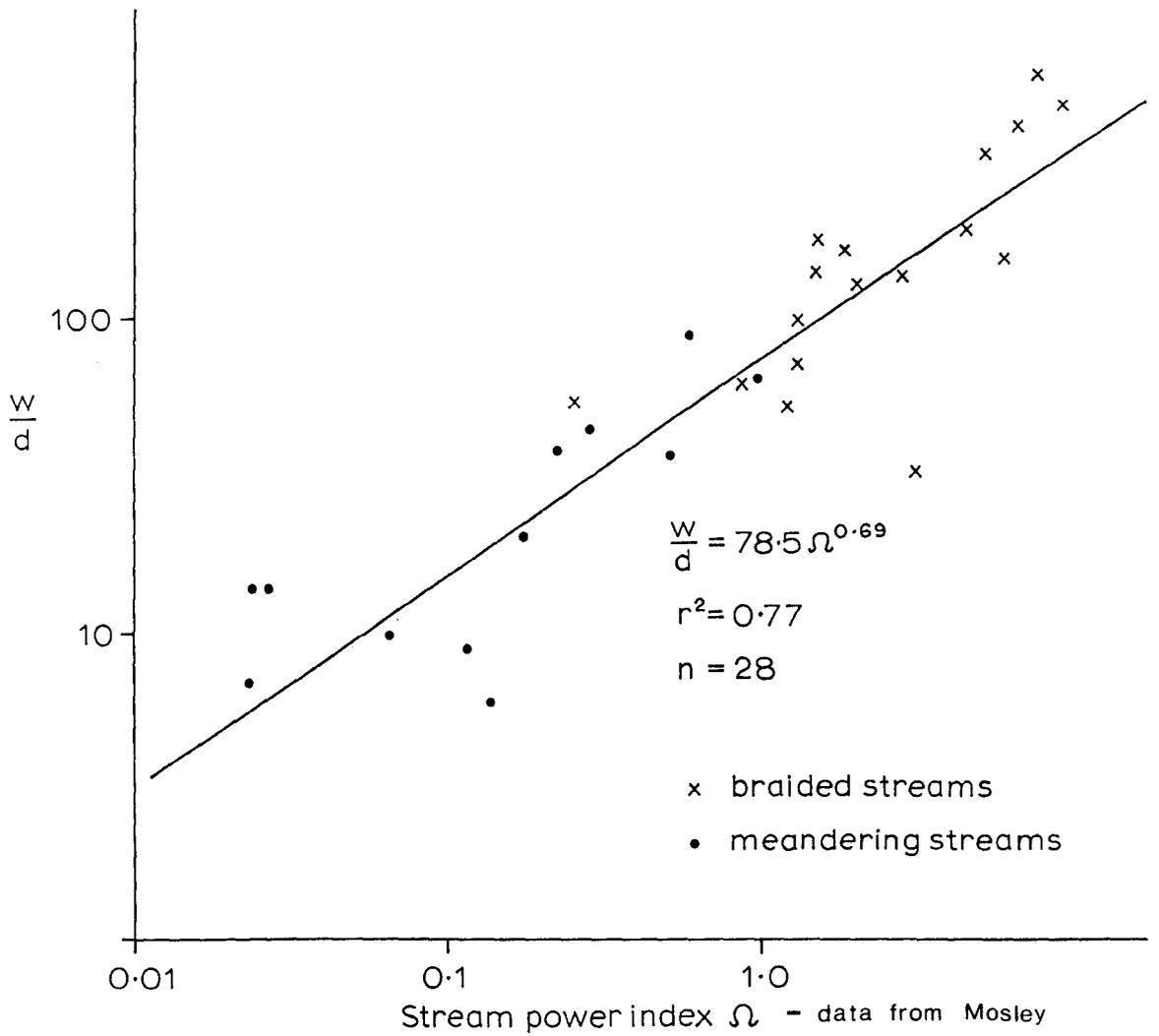
Figure 6.4 Plot of Width-Depth Ratio of Gravel-Bed Rivers against Increasing Stream Power
