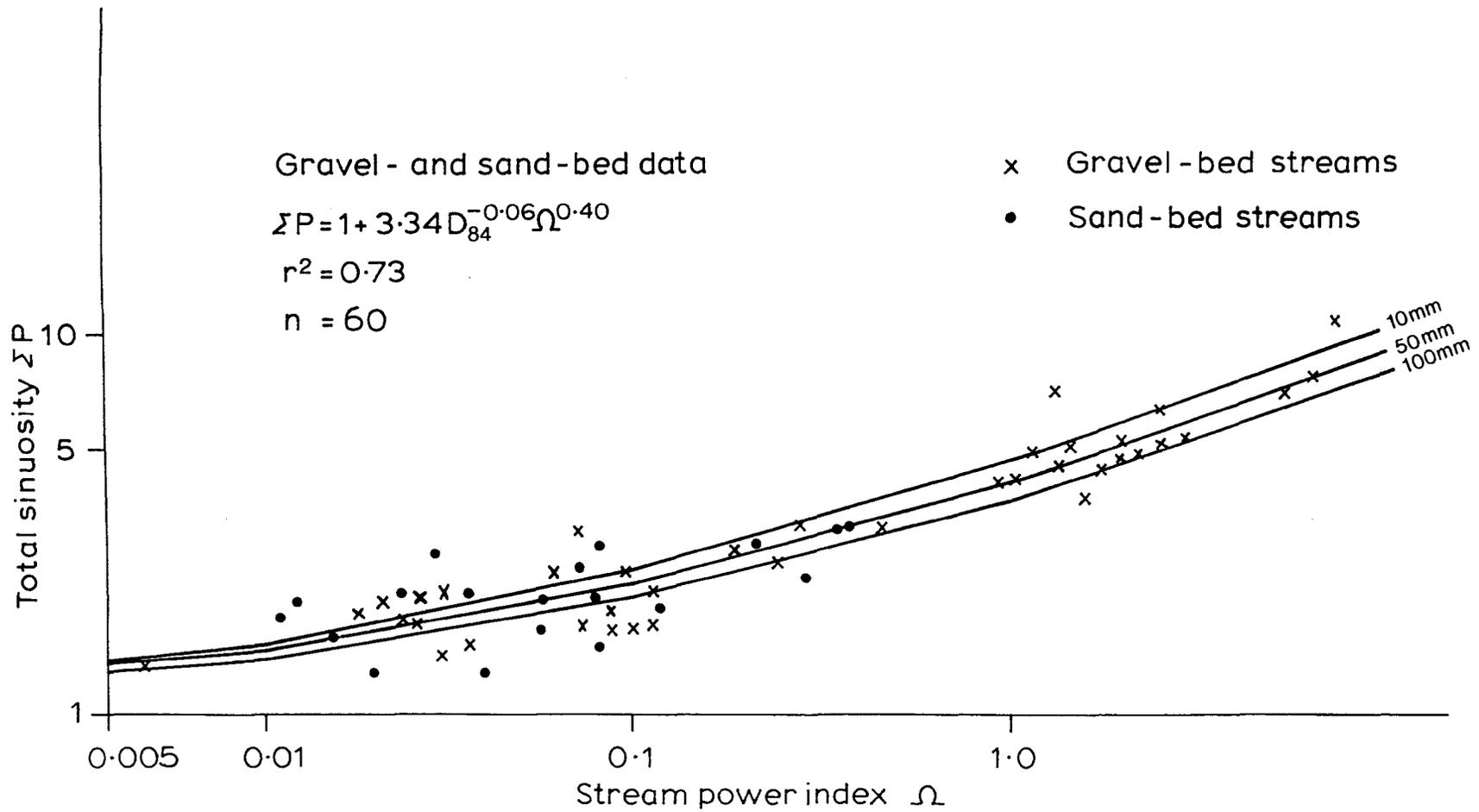
Figure 6.10 Multiple Regression of Total Sinuosity and Stream Power : Grain Size
