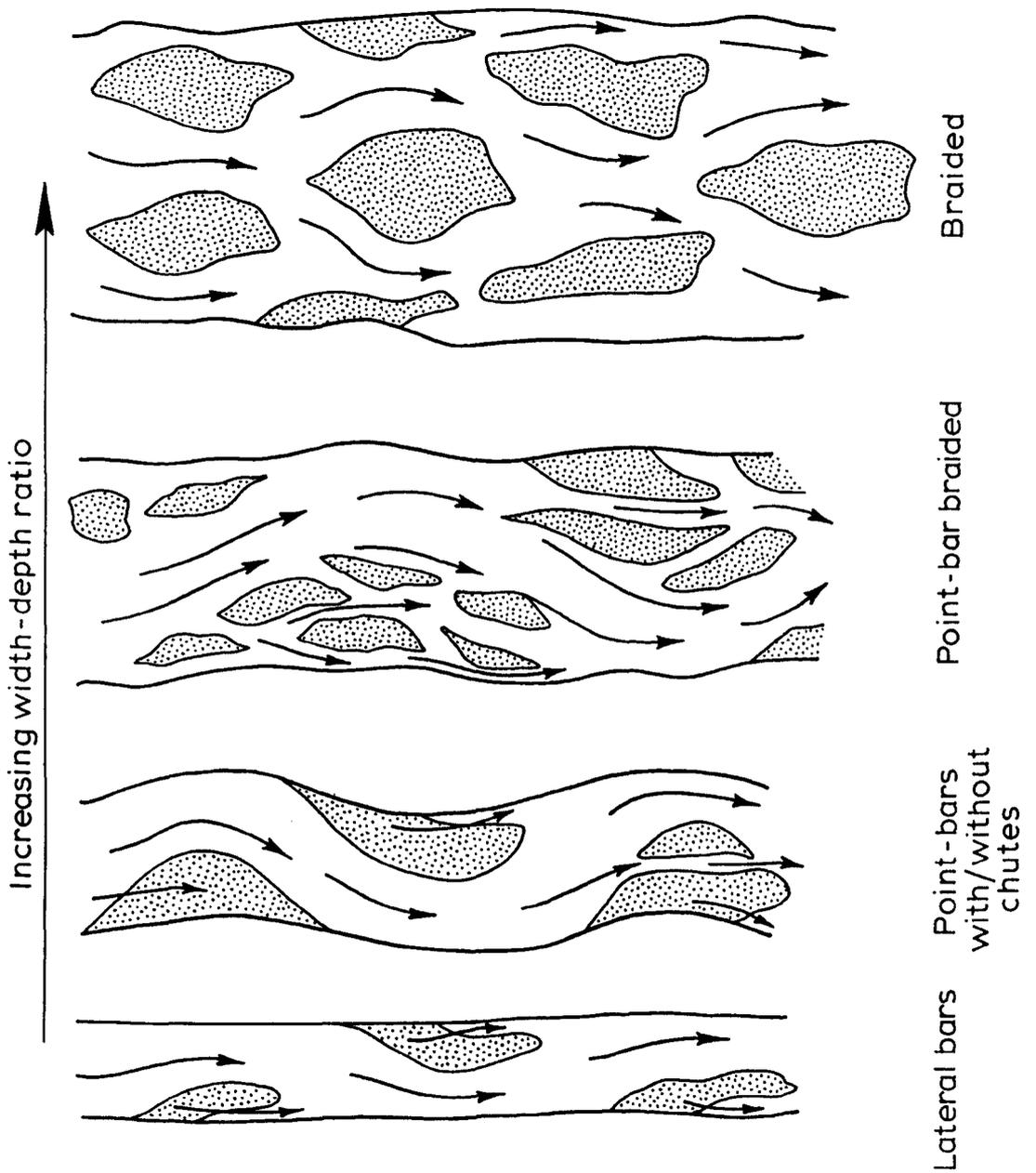
Figure 6.1 Continuum of bars in flume channels (after Schumm, 1972)
