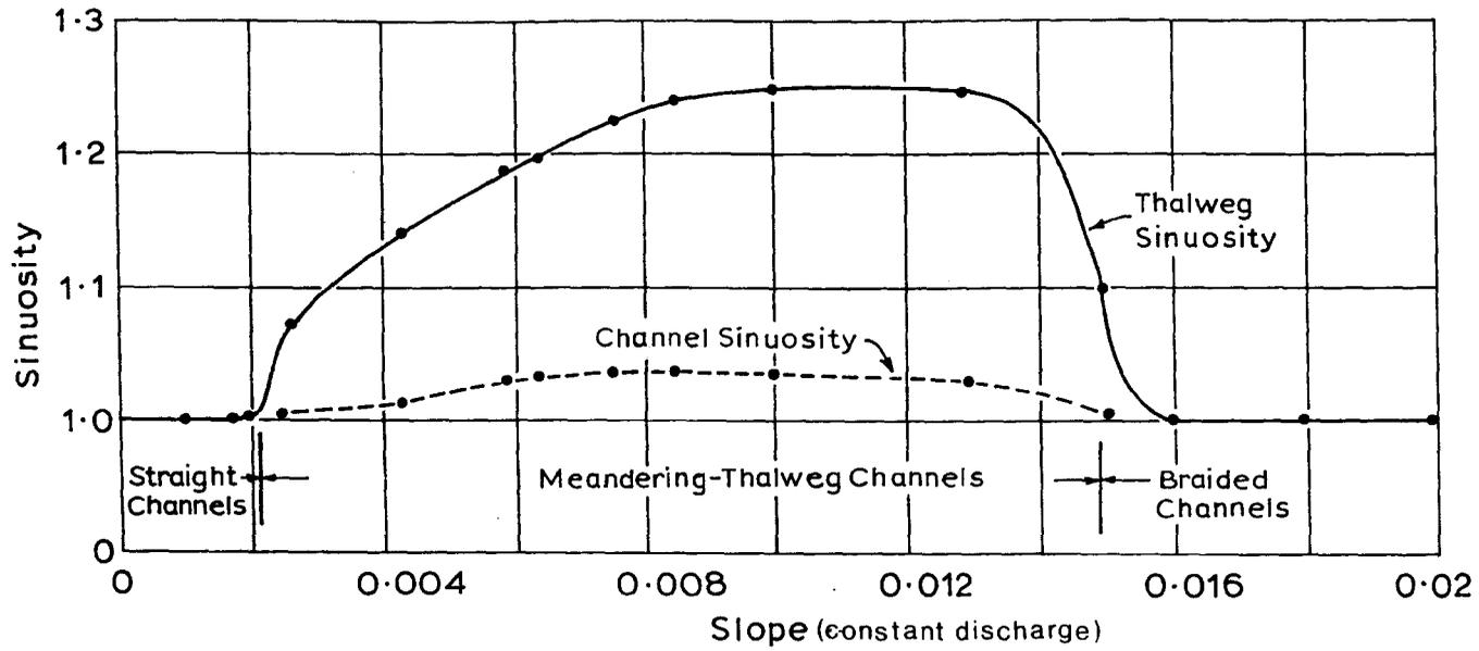
Figure 6.5 Changing Sinuosity in a flume channel at increasing slope (after Schumm & Khan, 1972)
