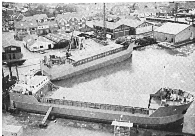
The two 499 g.r.t. motor barges "Lu" and "Wiggs" fitting out at the Danish shipyard Nordsovaerftet in Ringkobing. Both 45 m.-long vessels are now in service for Wilks Shipping, and will be followed by a third vessel in the early part of 1982.
