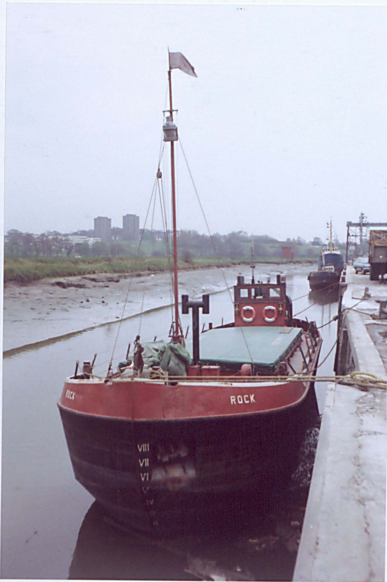
1 ROCK, L & R, 1961, 125 GRT, at Colchester. The low bulwarks fore and aft and the very low hatch coamings are evident.
