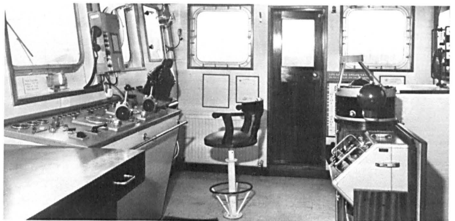
The wheelhouse is uncommonly roomy and well-equipped. Beyond the bridge control console is the radar and, above, the radio-telephone set.
