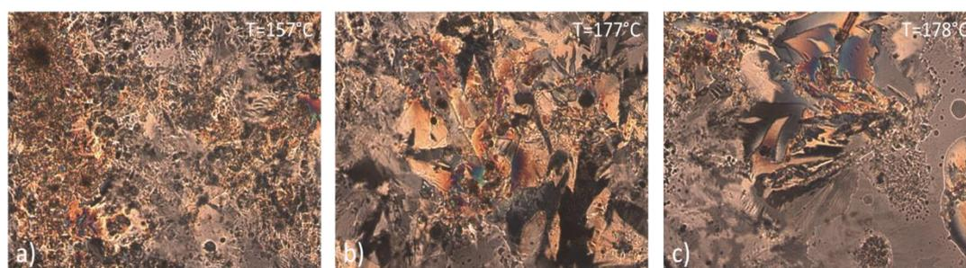
**Figure 8-10:** Textures obtained by OPM for compound 8-9. a) SmA at 157 °C, b) and c) nematic at 177 °C and 178 °C.
