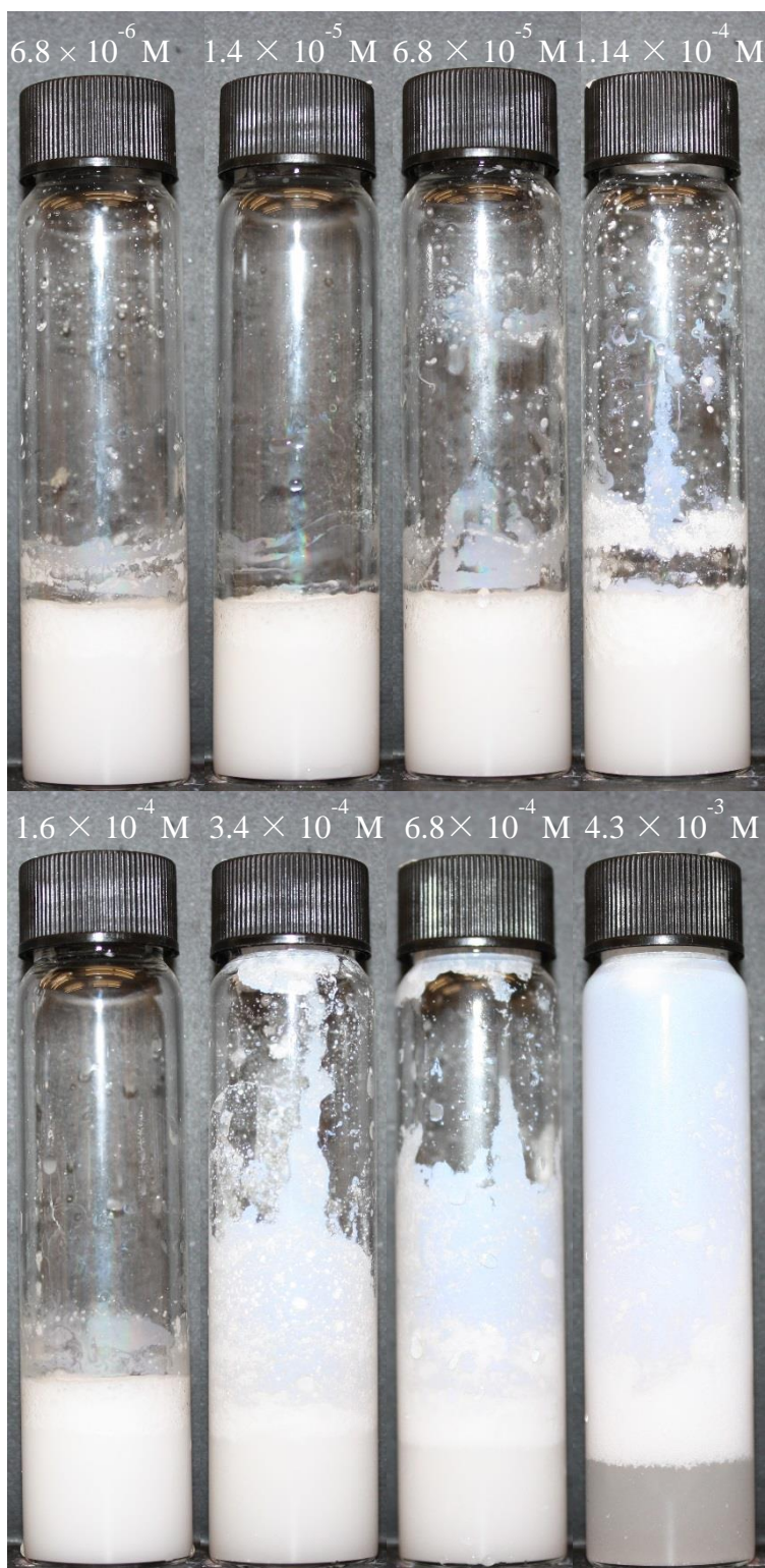
Figure 4.14. Images of aerated particle suspensions generated with 5 wt. % 2 \mu\text{m} diameter silica particles (hydrophobised to varying extents with 1H, 1H, 2H, 2H-perfluorooctylmethyldichlorosilane) in 5 ml water. Suspensions aerated for 60 seconds by homogenisation. Images taken using a Canon EOS450D camera at t=0 .
