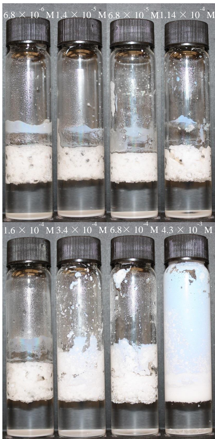
Figure 4.22. Images of aerated particle suspensions generated with 5 wt. % 2 \mu\text{m} diameter silica particles (hydrophobised to varying extents with 1H, 1H, 2H, 2H-perfluorooctylmethyldichlorosilane) in 5 ml 15 wt. % ethanol. Suspensions aerated for 60 seconds by homogenisation. Images taken using a Canon EOS 450D camera at t=24 hours.
