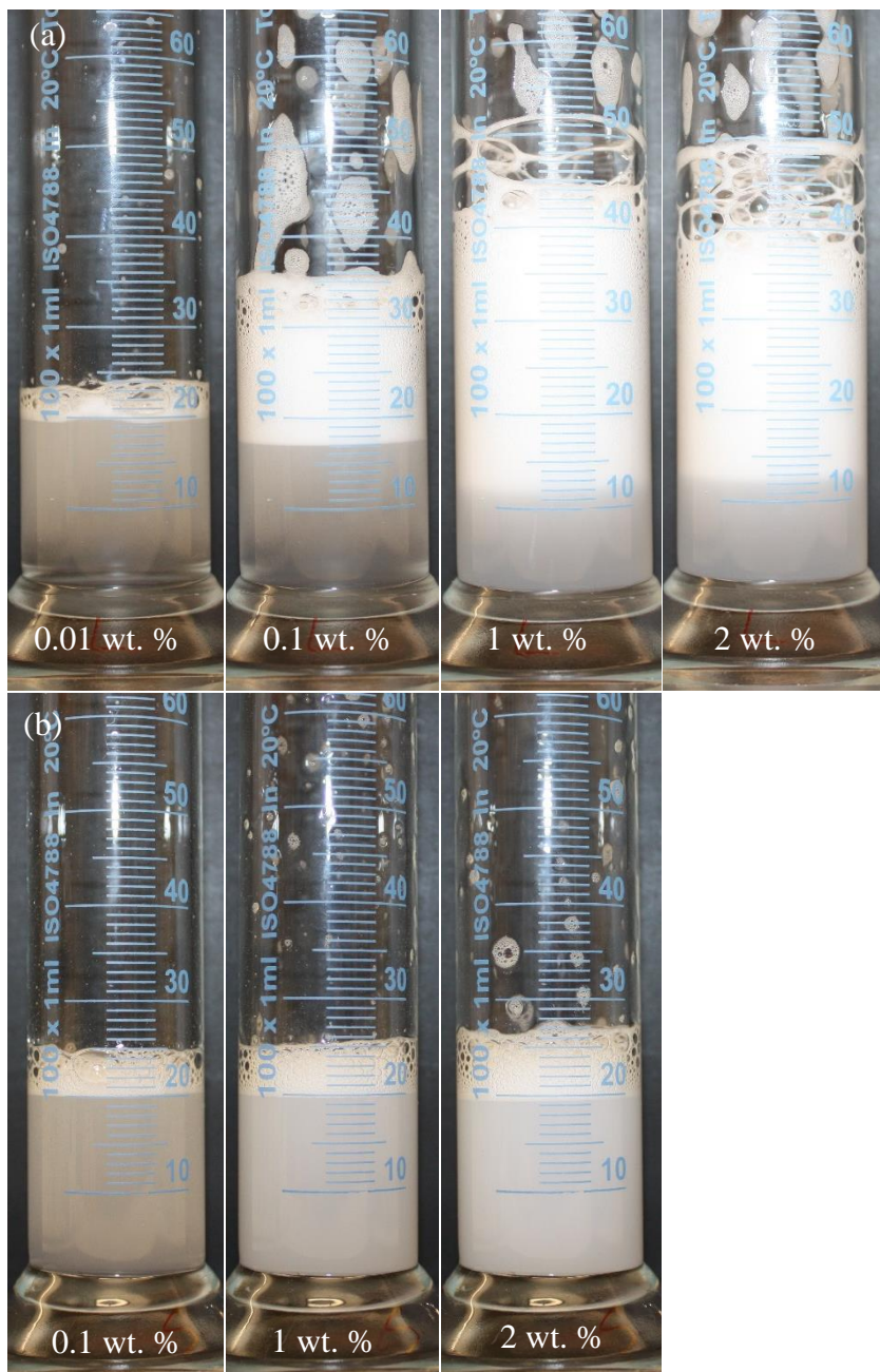
Figure 3.3. Foams generated by hand shaking (30 s) 20 ml surfactant solution (a) Lamesoft PO65 (b) Silsurf DI-2510 as a function of surfactant concentration (0.01-2 wt. %, left to right). Images taken with a Canon EOS450D camera immediately after generation.
