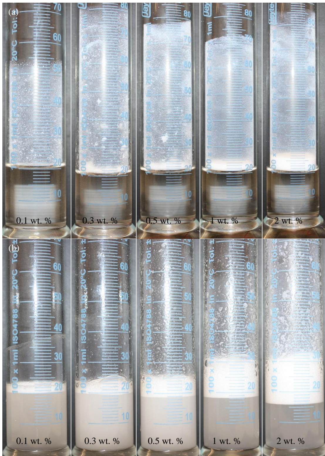
Figure 3.18. Images of aerated particle suspensions generated by hand shaking (30 s) 20 ml of (a) 20% SiOH fumed silica in water and (b) 47% SiOH fumed silica in water. Particle concentration increases from 0.1-2 wt. % (left to right). Images taken on a Canon EOS450D immediately after aeration.
