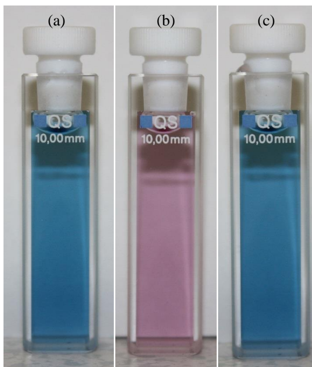
Figure 5.4. Images of cuvettes containing 2 ml 16 \mu\text{M} NBB dye and 1.4 ml Fenton reagents, or water after 20 minutes analysis in UV-visible spectrophotometer. (a) Appearance of all samples prior to analysis (b) after addition of 10 mM \text{CuSO}_4 and 100 mM \text{H}_2\text{O}_2 (c) after addition of 100 mM \text{H}_2\text{O}_2 only.
