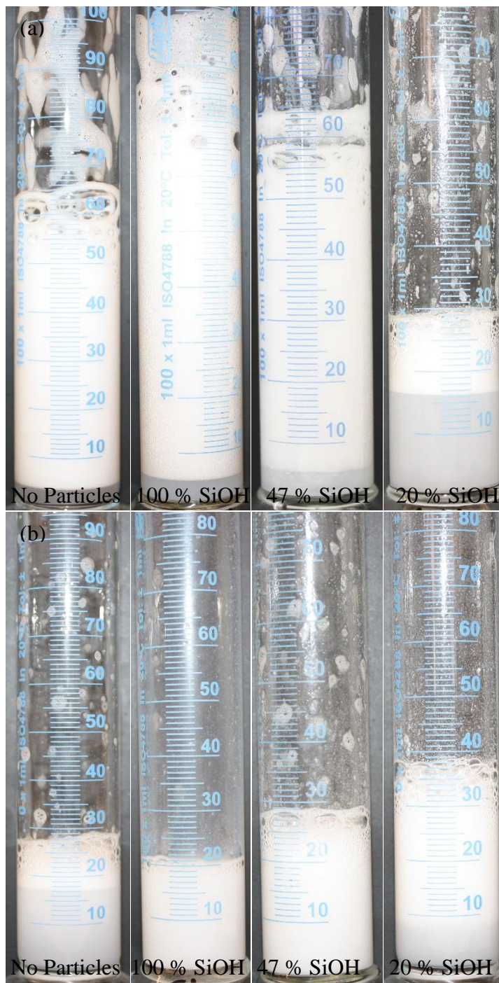
Figure 3.49. Images of foams generated by hand shaking (30 s) 20 ml of 1 wt. % surfactant with 1 wt. % fumed silica (20-100% SiOH) (a) Lamesoft PO65 and (b) Silsurf DI-2510. Images taken on a Canon EOS450D immediately after aeration.
