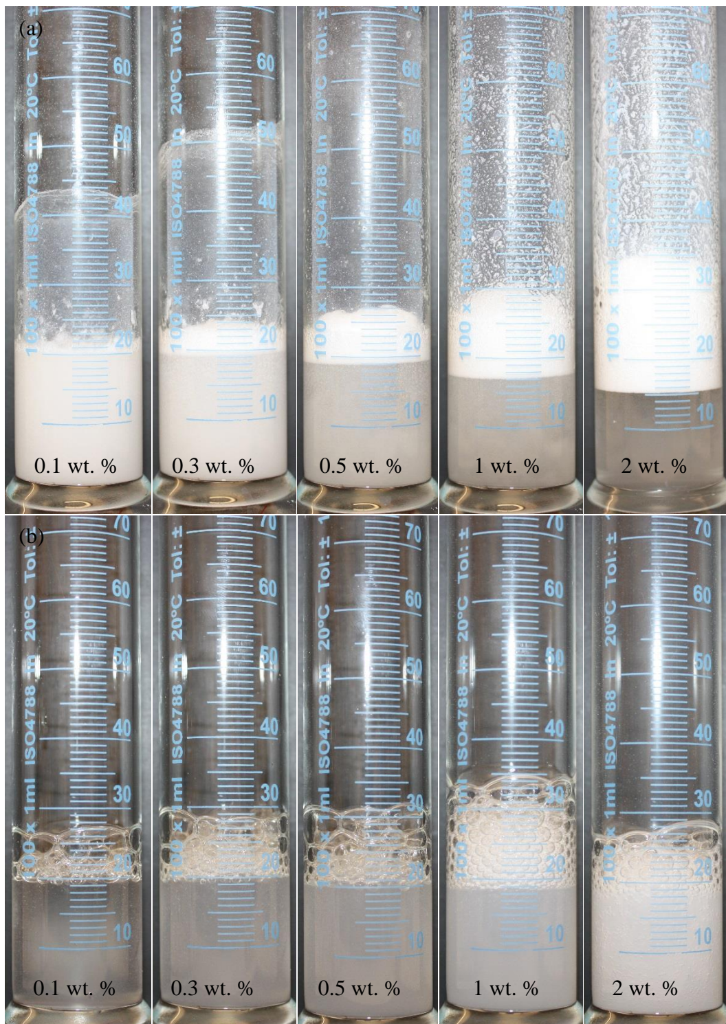
Figure 3.22. Photos of foams generated by hand shaking (30 s) 20 ml of 20 wt. % ethanol containing (a) 20% SiOH fumed silica and (b) 47% SiOH fumed silica. Particle concentration increases from 0.1-2 wt. % left to right. Images taken on a Canon EOS450D immediately after aeration.
