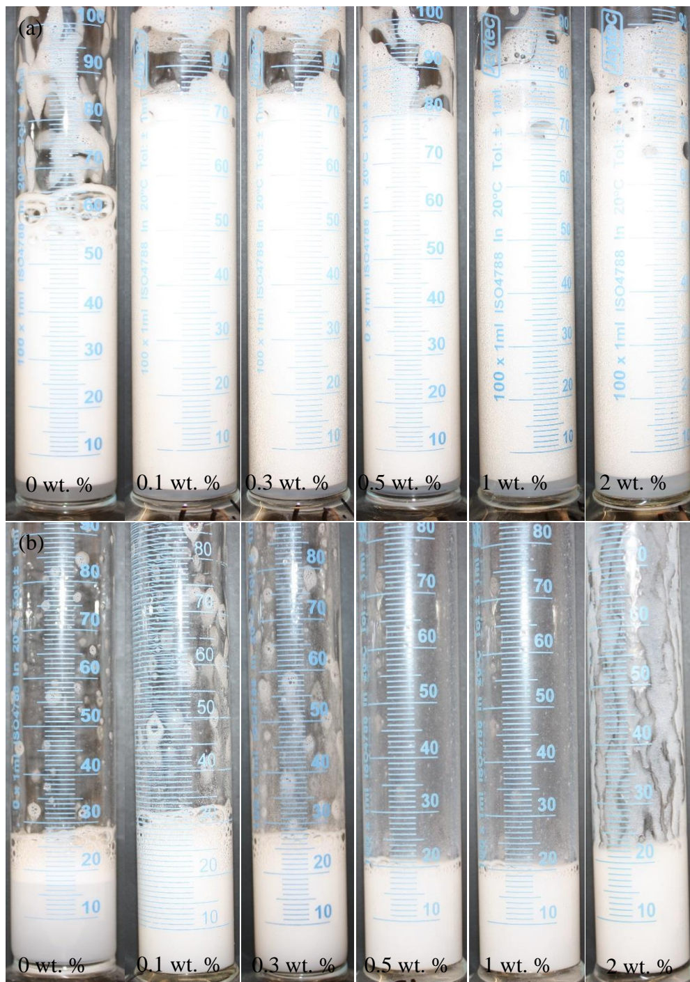
Figure 3.40. Photos of foams generated by hand shaking (30 s) 20 ml of 1 wt. % surfactant with 0-2 wt. % 100% SiOH fumed silica. (a) Lamesoft PO65 (b) Silsurf DI-2510. Images taken on a Canon EOS 450D immediately after aeration.
