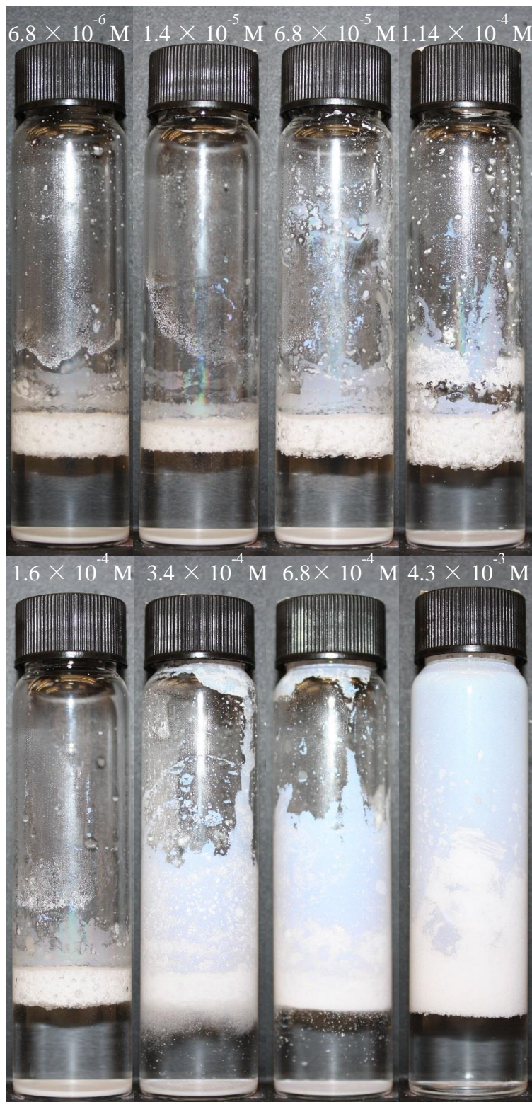
Figure 4.15. Images of aerated particle suspensions generated with 5 wt. % 2 \mu\text{m} diameter silica particles (hydrophobised to varying extents with 1H, 1H, 2H, 2H-perfluorooctylmethyldichlorosilane) in 5 ml water. Suspensions aerated for 60 seconds by homogenisation. Images taken using a Canon EOS450D camera at t=24 hours.
