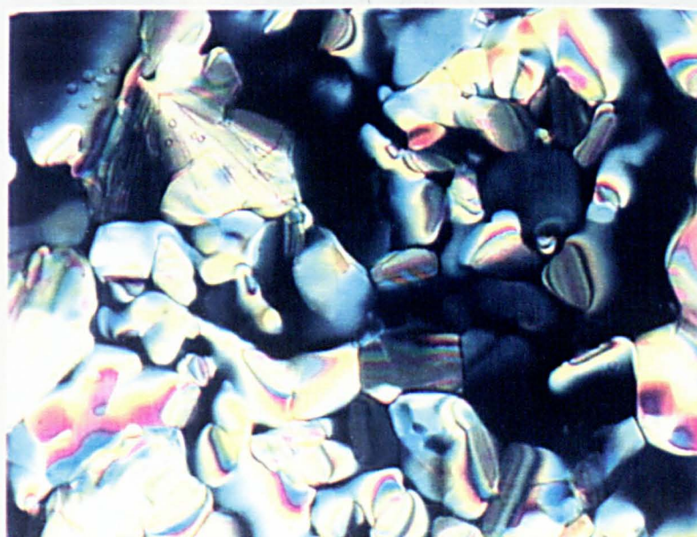
Plate 1.2 : Hexagonal ordered ( D_{ho} ) columnar mesophase exhibited by 2,3,6,7,10,11-hexakis(decyloxy)triphenylene at 67 °C on cooling from the isotropic liquid
