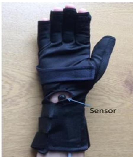
**Legend:** Each sensor was held in place at the wrist by passing the wire of the sensor under the Velcro straps of the data gloves.
