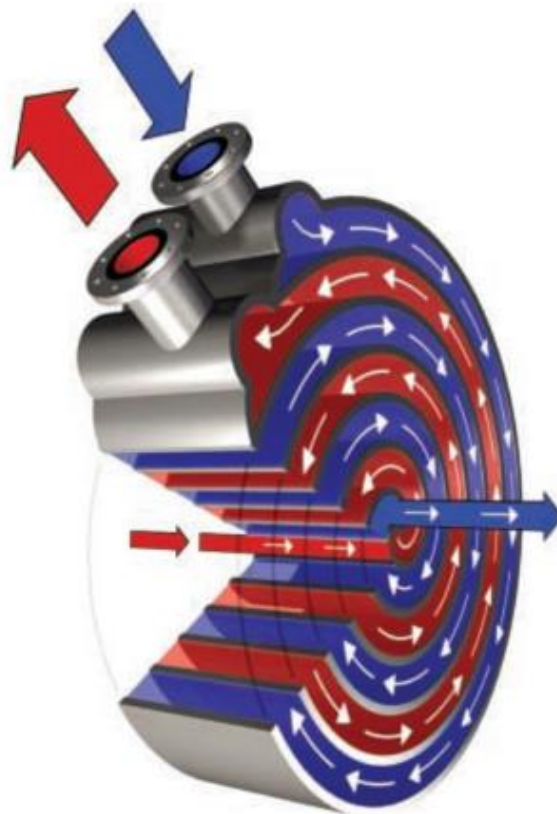
Figure 2-4 Spiral heat exchanger (courtesy of Alfa Laval) [158]
