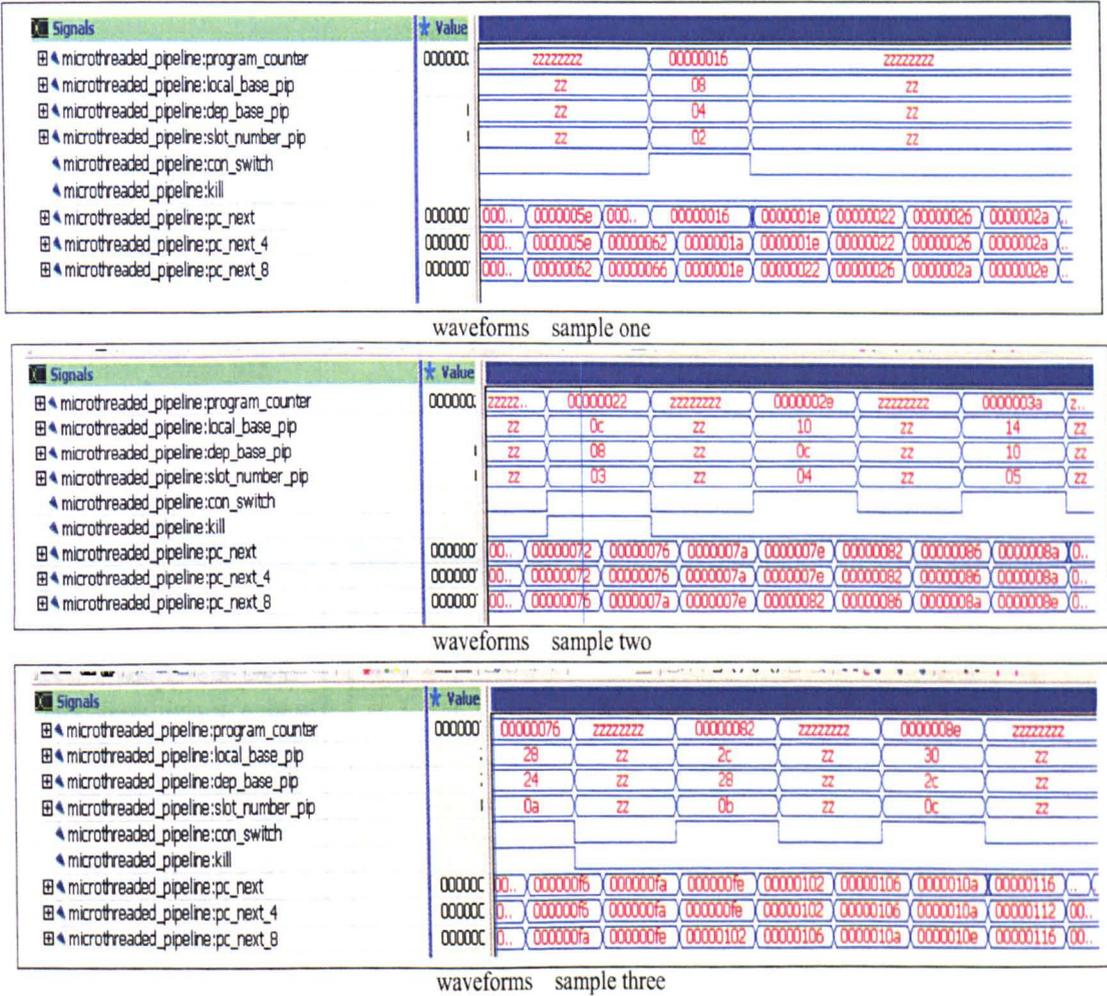
Figure D.4: Simulation waveforms showing microthreaded pipeline with context switch and kill instructions.
