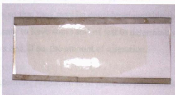
**Figure 3.7: Surface cured resin (Tack Free). Note also slight yellowing on cure.**
