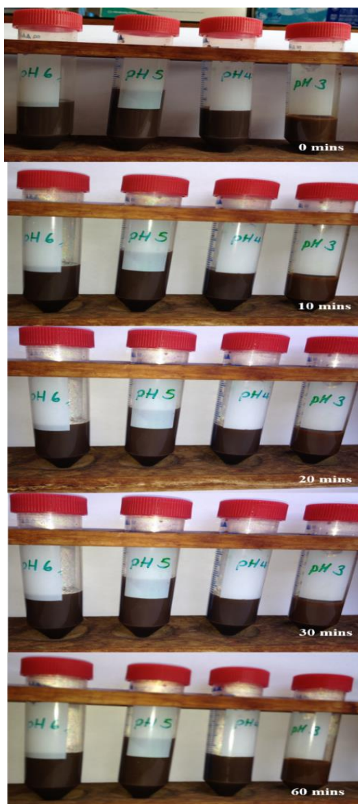
Figure 6-13 Aqueous suspensions of \gamma -Fe 2 O 3 coated with citric acid, prepared at different pH.
