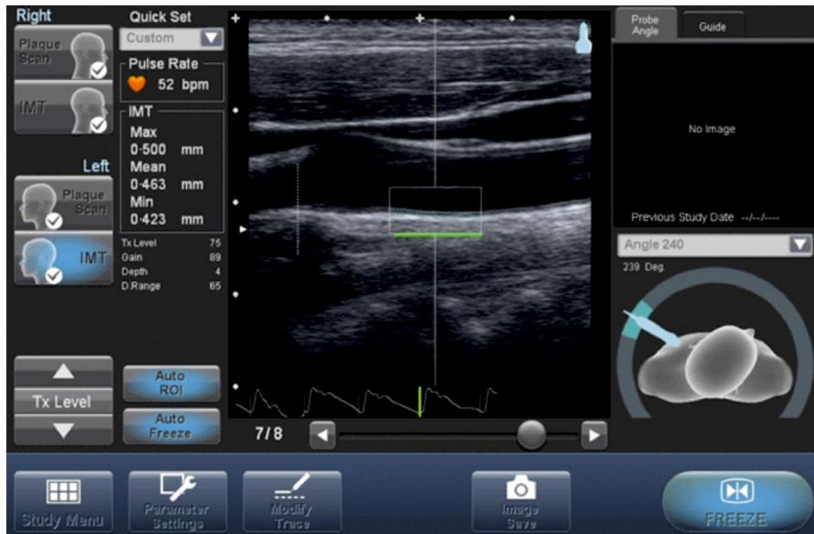
Figure 1 A screenshot showing C-IMT investigation where angle of examination is displayed and recorded using an integrated system (Bottom Right). The region of interest (ROI) is located within the white box (centre) and is parallel to a white vertical dotted line (centre-left). The distance between these two features measures 1 cm and allows the operator to measure the distance between the flow divider and the C-IMT measurement site during the scan.
