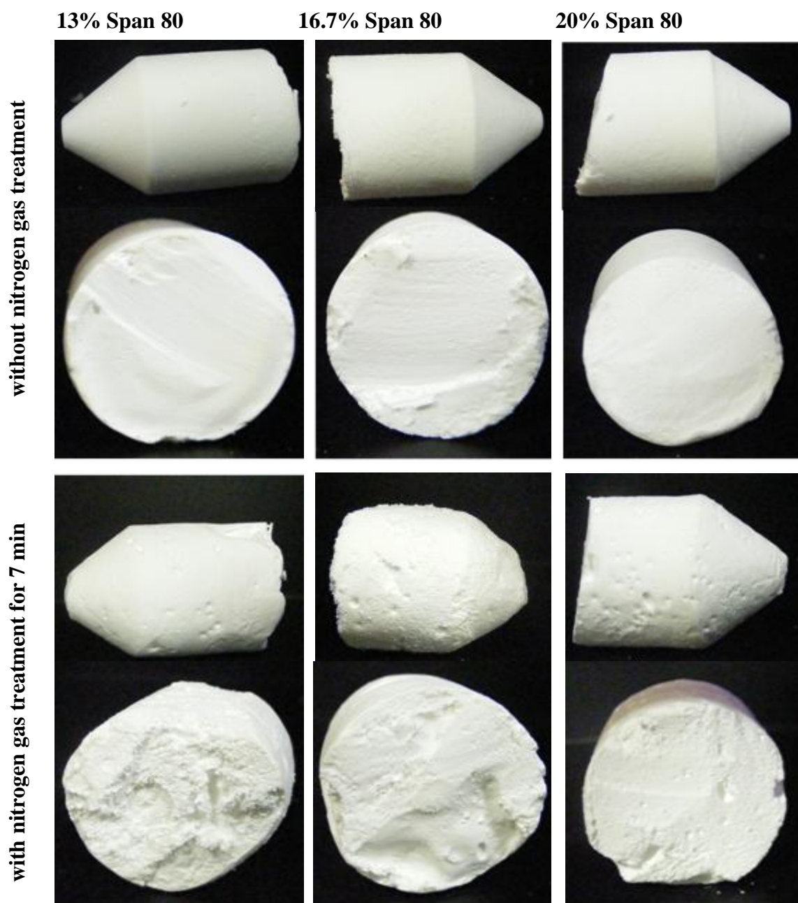
Figure 5.5. (a) Images of porous polymeric materials obtained after polymerisation of HIPEs of Styrene at volume fraction of water 0.8. All materials have been purified twice by Soxhlet extraction.
