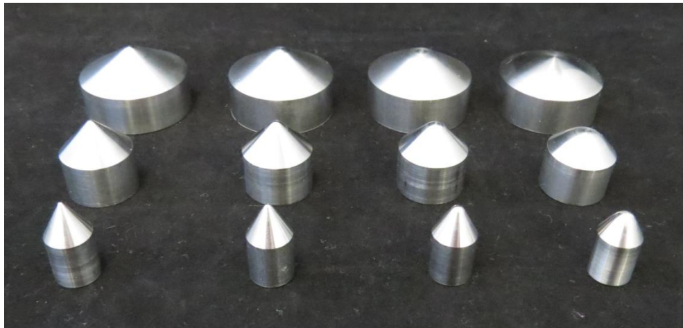
Figure 2.12 Stainless steel cusp models used in study, which were made in angles of 60°, 90° and 120° (front to back), and blunting distances B, C, D and E (left to right).
