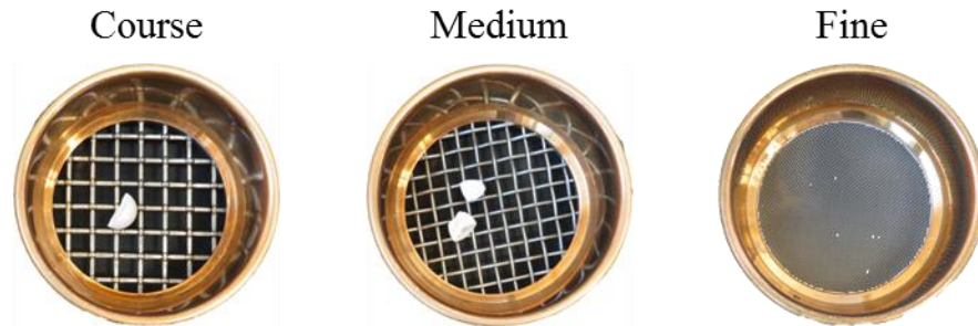
Figure 2.26 Examples of fragments for each size category. Images from E120 test runs.
