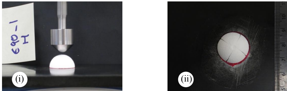
Figure A.29 E90 hollow hard object breakdown images: (a) E90 and hollow dome, (b) post compression image. Domes split into 2-4 pieces.
