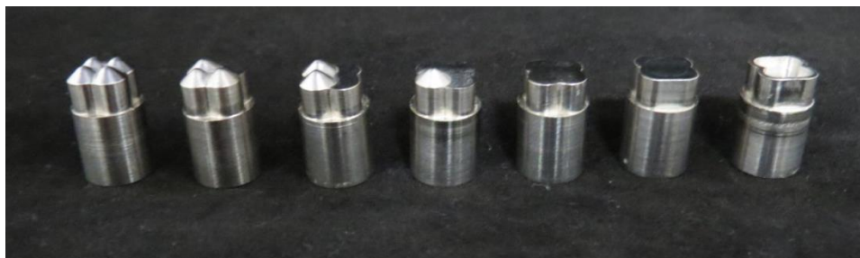
Figure 4.16 Stainless steel crown models used to investigate the effects of dental wear on mechanical performance in C.atys . Images from left to right; 4 cusp, 3 cusp, 2 cusp, 1 cusp, 0 cusp, 0 ridge, ridge.
