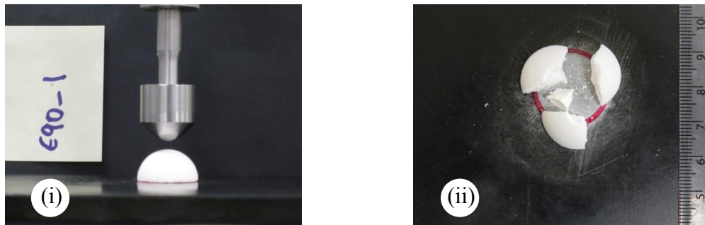
Figure A.31 E90 solid hard object breakdown images: (i) E90 and solid dome, (ii) post compression image. Domes typically split into 3-4 pieces and energetically moved apart at failure.
