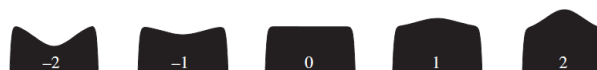
Figure 4.3 Series of 5 cusps used by Crofts and Summers (2014) to investigate the effects of concavity and convexity to fracture brittle snail shells.
