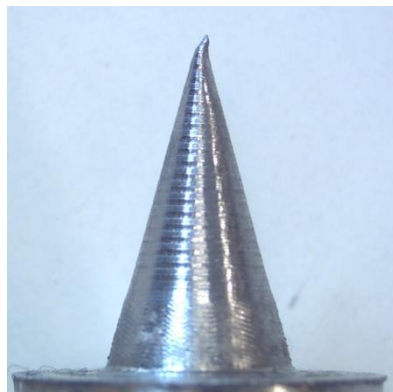
Figure 2.73 Image of a stainless steel B30 cusp with a deformed tip.
