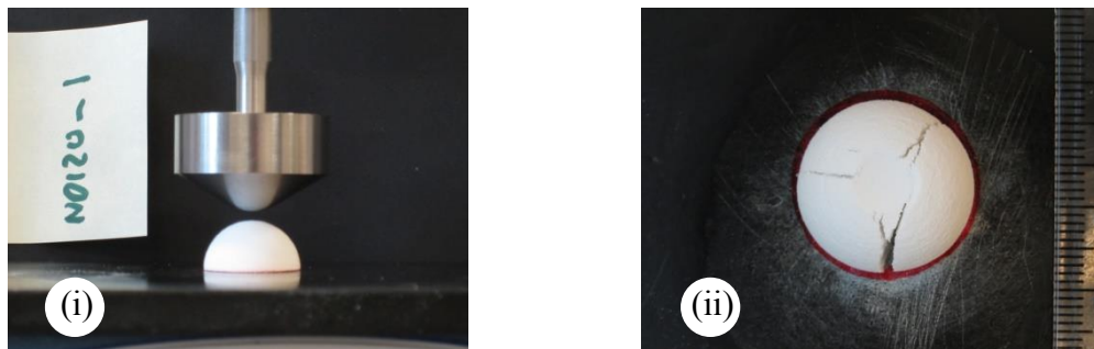
Figure A.43 D120 solid hard object breakdown images: (i) D120 and solid dome, (ii) post compression image. Domes typically split into 3 pieces.
