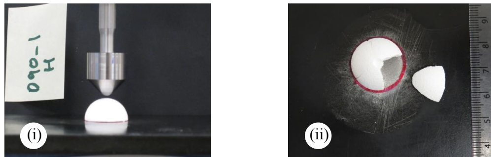
Figure A.25 D90 hollow hard object breakdown images: (i) D90 and hollow dome, (ii) post compression image. Domes split into 3-4 pieces and energetically moved apart at failure.
