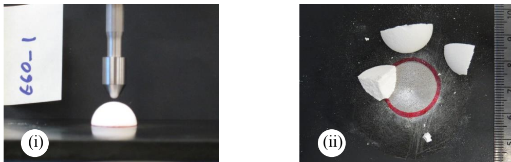
Figure A.15 E60 solid hard object breakdown images: (i) E60 and solid dome, (ii) post compression image. Domes split into 2-4 pieces and energetically moved apart at failure.
