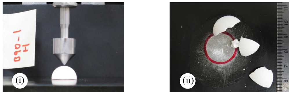
Figure A.17 B90 hollow hard object breakdown images: (i) B90 and hollow dome, (ii) post compression image. Domes split into 2-4 pieces and energetically moved apart at failure.
