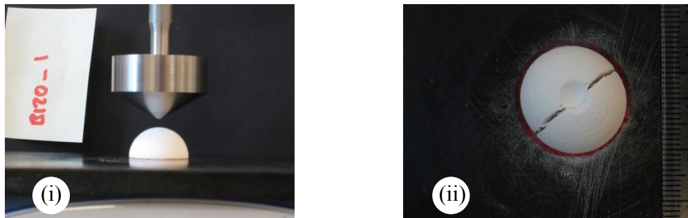
Figure A.35 B120 solid hard object breakdown images: (i) B120 and solid dome, (ii) post compression image. Domes typically split into 2-3 pieces.
