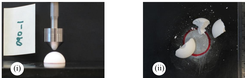
Figure A.27 D90 solid hard object breakdown images: (i) D90 and solid dome, (ii) post compression image. Domes typically split into 3 pieces and energetically moved apart at failure.
