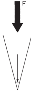
Figure 1.14 Schematic diagram of a sharp cusp that has a small area of initial contact, therefore maximises the amount of pressure when in contact with a food item. From Strait (1997).
