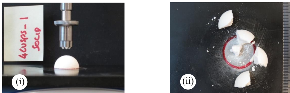
Figure C.7 4 cusps solid hard object breakdown images: (i) 4 cusps and solid dome, (ii) post compression image. Domes split into 2-4 pieces and energetically moved apart at fracture.
