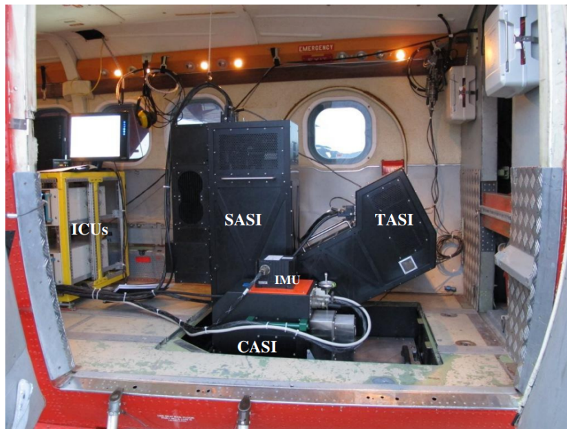
Figure 3.4: The sensor installation in the BAS Twin Otter aircraft (ITRES, 2012); Abbreviations are as follows: ICU, instrument control unit; IMU, inertial measurement unit.
