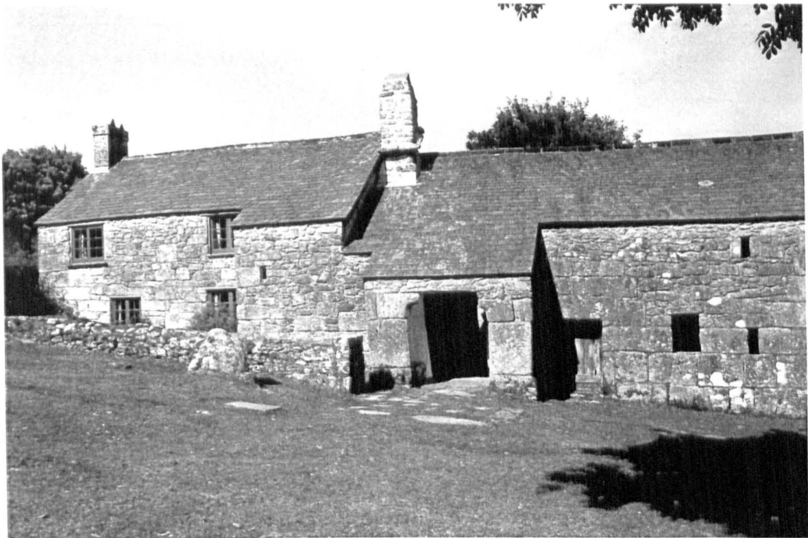
Plate 1 Longhouse, Lettaford, Dartmoor, Devon. An early building form in which humans and cattle were accommodated under one roof, separated by a cross-passage
