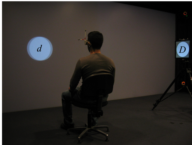
Fig. 6.4 Photograph of the experiment apparatus. The standard disc D is displayed on a LED monitor fixed to a tripod. The response d is displayed on the HIVE screen. When wearing the LCD shutter glasses the stereo separation is not visible to the participant and the disc is perceived to be 1m away. Note that the lighting conditions of the photograph are not illustrative of the actual experimental conditions. Aside from labelling the discs, the photograph image has not been manipulated.
