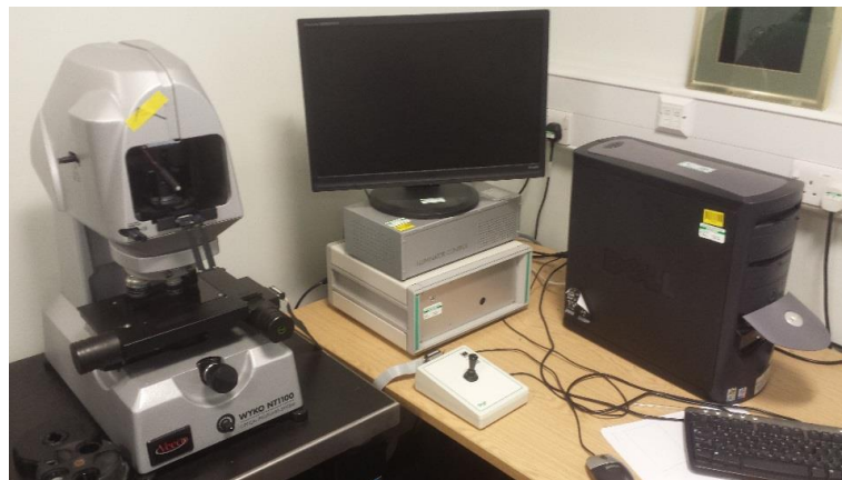
Figure 18- Veeco WYKO NT1100 white light interferometer
