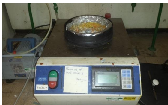
Figure 20-Spincoater machine used for coating thin film substrate on alumina discs.
