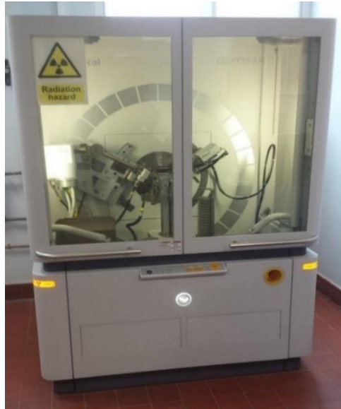
Figure 17-PANalytical, Empyrean X-ray diffractometer
