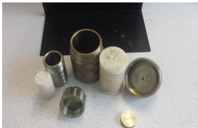
Figure 21-Autoclaves used for MOF synthesis process.
