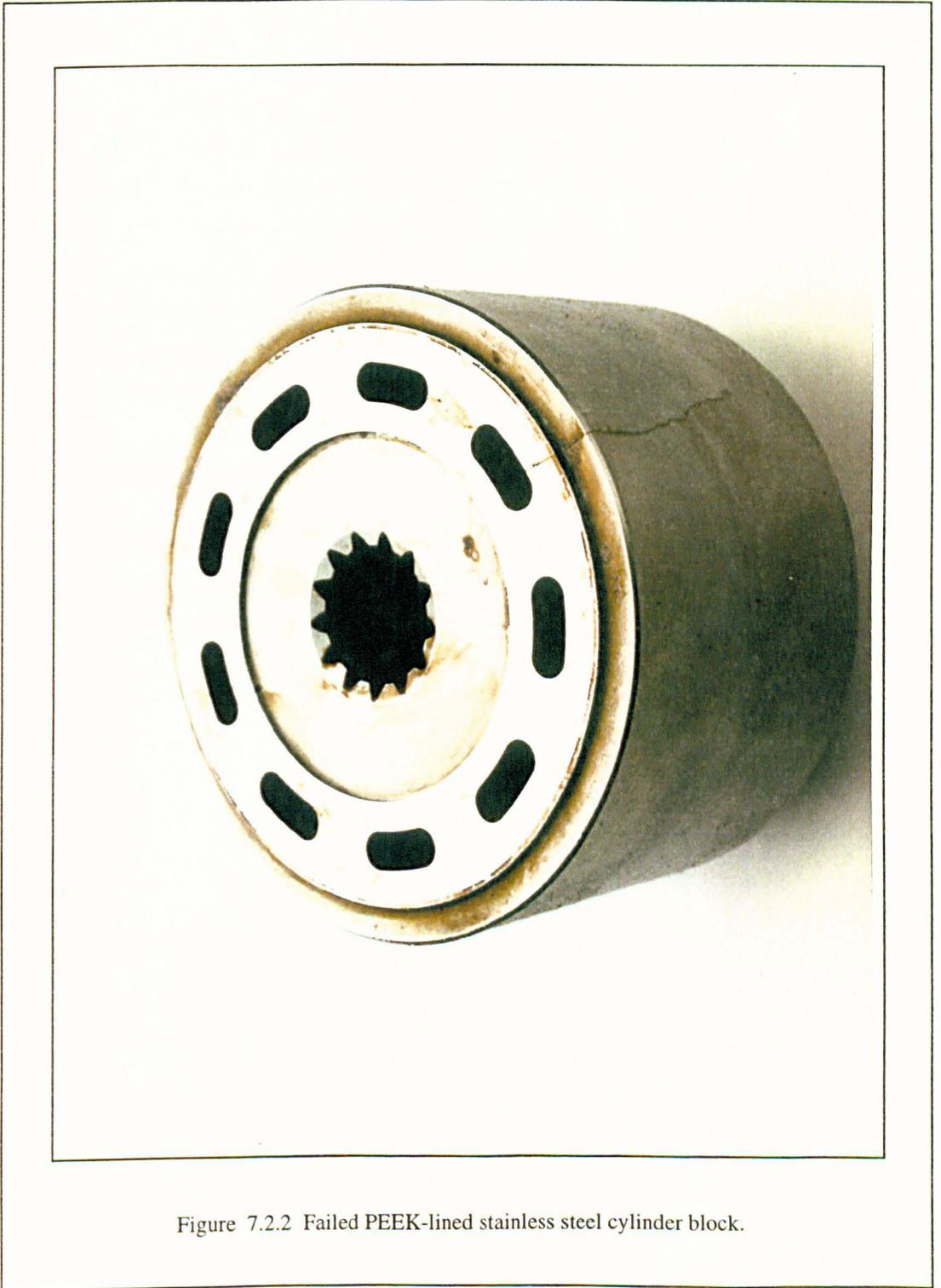
Figure 7.2.2 Failed PEEK-lined stainless steel cylinder block.
