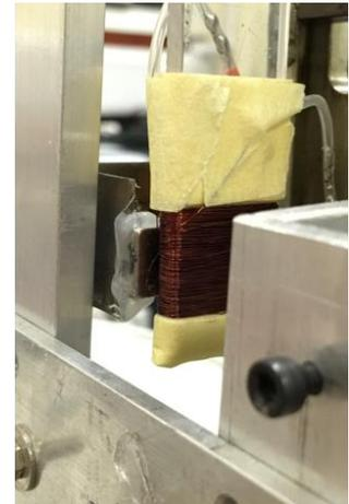
Figure 92: Dimensions of the coil and cantilever magnet and actual prototype.
