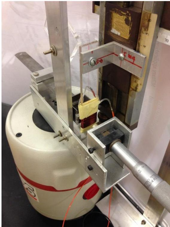
Figure 86: Placement of the bar coil within the prototype during the experiments.
