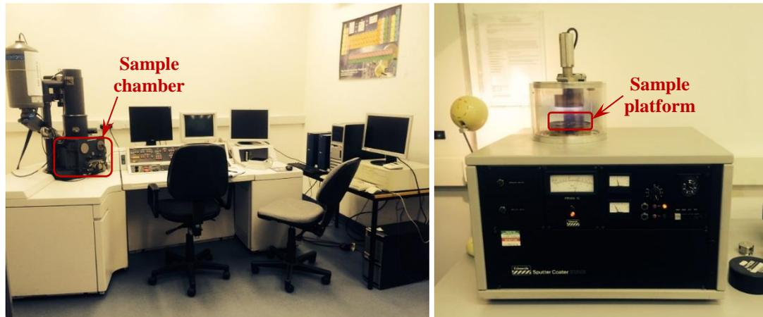
**Figure 3-17** Equipment used for scanning electron microscopy: (a) SEM operation system; (b) sputter gold coater.
