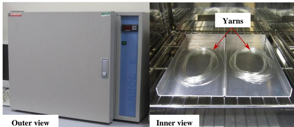
**Figure 3-14** Fan-assisted oven used for fibre annealing. Inner view shows the yarns were placed in aluminium trays to ensure uniform heat treatment and prevent movement from air flow.
