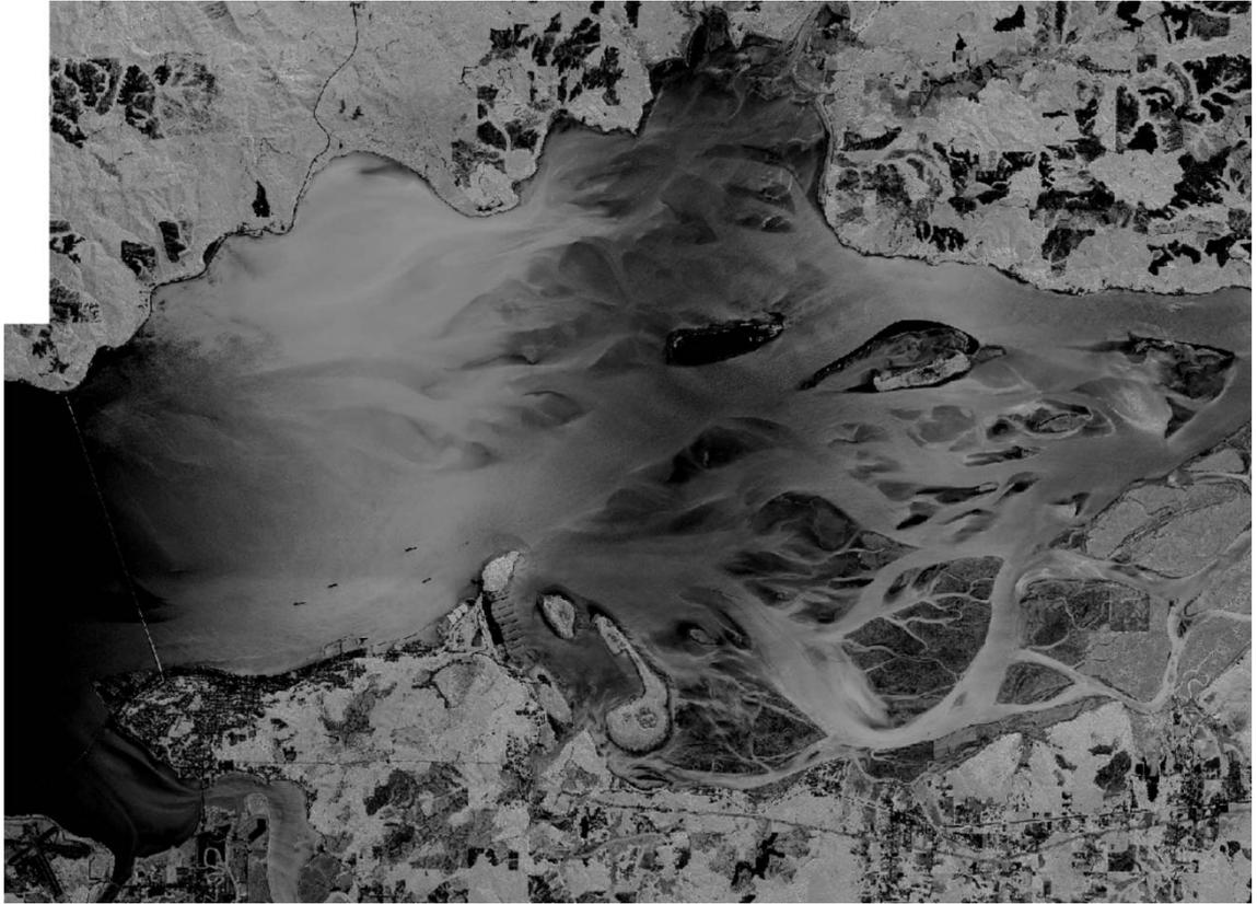
**Figure 2.32 Image of the Columbia River estuary showing sand bars present close to the water surface. Note the elongated tails visible at the seaward end of several bars. Fluvial flow is from the east.**
