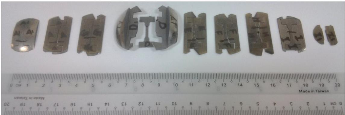
Figure 3.2 The dog-bone shape samples and other pieces cut from a button ingot using EDM.
