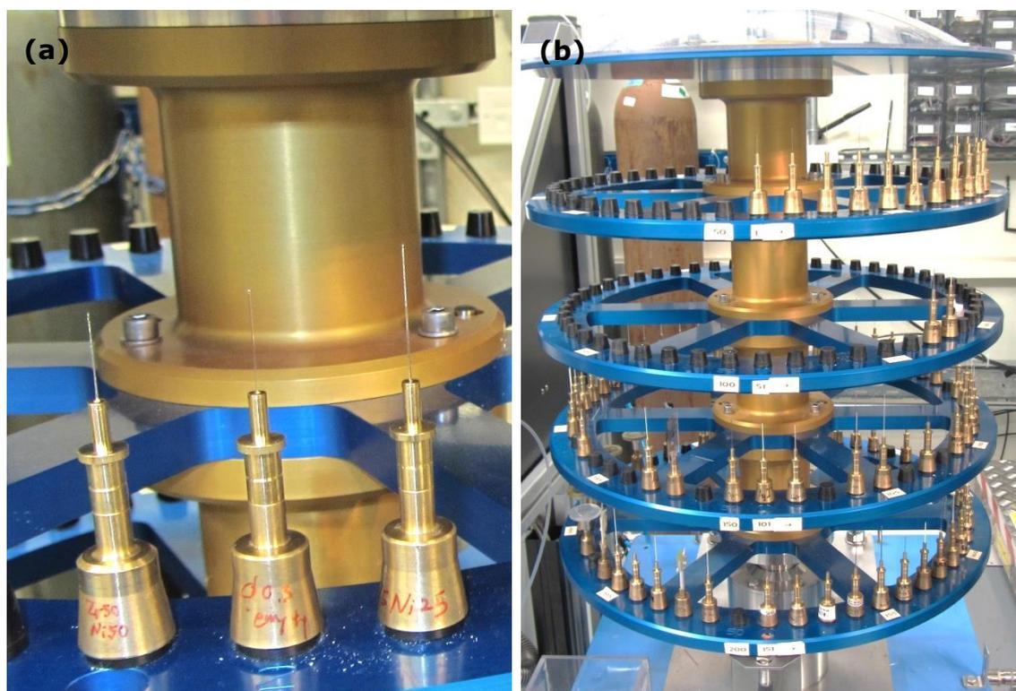
Figure 5.26 Samples prepared for the anomalous X-ray scattering experiments, (a) thin strips samples in the borosilicate capillary tubes and brass sample holders (b) samples placed on the carousel.
