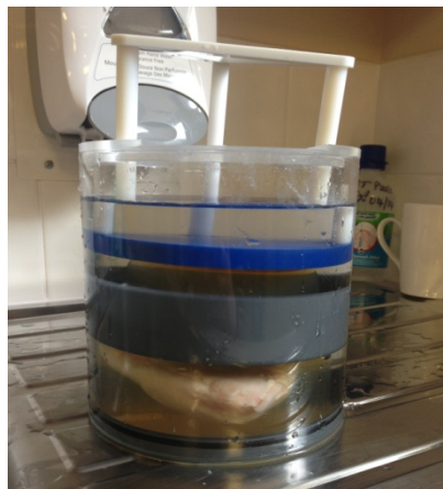
Figure 10.22: The turkey breast phantom in a container filled with degassed water with an acoustic window at the bottom and acoustically absorbent plate at the top.
