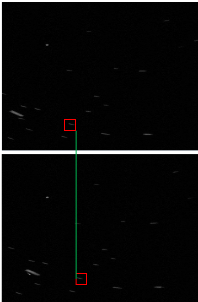
Figure 6.1: Micro-particle's position changes over the frames without overlapping with previous position. Images from experiment with analyte concentration of 100 nM and frame numbers are 7th and 8th respectively.
