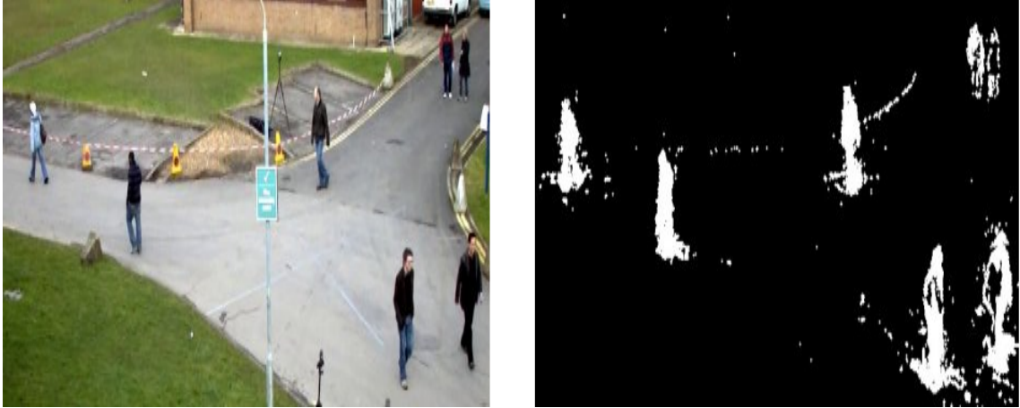
Figure 4.3: Background subtraction with application of several statistical and mathematical operations (Mixture of Gaussian) on 112th frame of the PETS sequence. Comparing Figure 4.2 and Figure 4.3 it can be seen that the amount of noise and discontinuity is less compared to the background subtraction using frame difference only shown in Figure 4.2. But still many discontinuity and noise can be seen in Figure 4.3, which can lead to erroneous detection (both positive and negative) of object(s).
