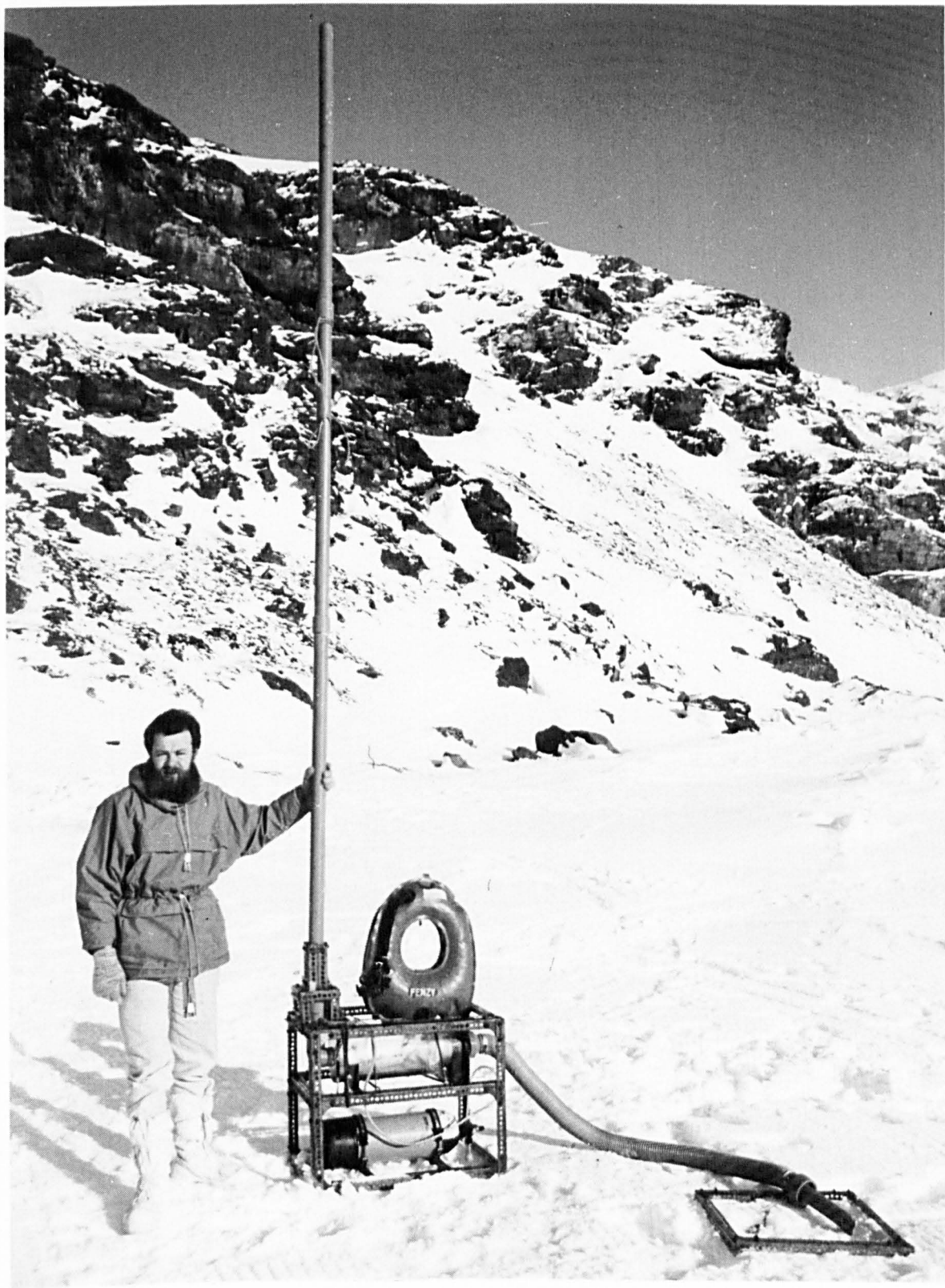
Fig. 30. The author pictured with the modified Hiscock and Hoare (1973) suction sampler assembled in it's working state. An inflatable air-bag was attached to the frame of the sampler to assist lifting to the surface after the sampling session was completed.
