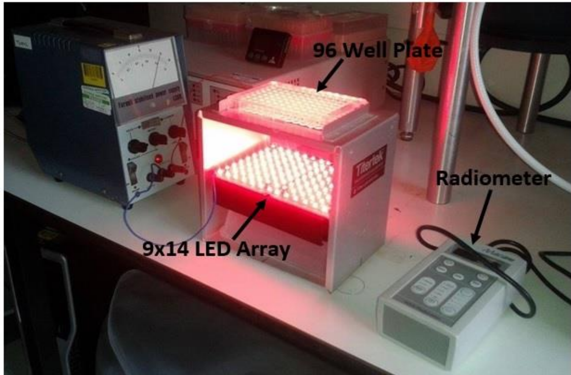
Figure 2.1: Setup of the equipment used in the photodynamic therapy treatment of cancer cell lines.
