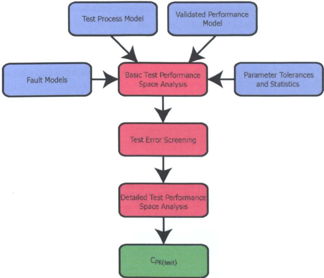
Figure 7-3 Block Diagram Showing the Main Elements of Test Capability Analysis
