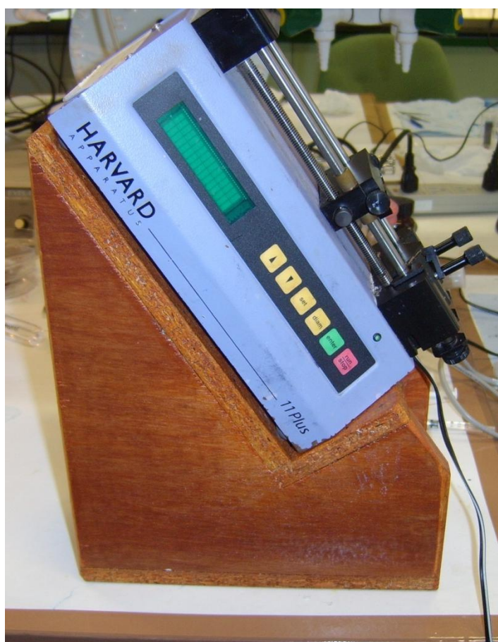
Figure 41: Syringe pump on wooden stand, constructed to ensure that the cells in the syringe did not settle to the sides of the syringe but were capable of being pumped through the chip.
