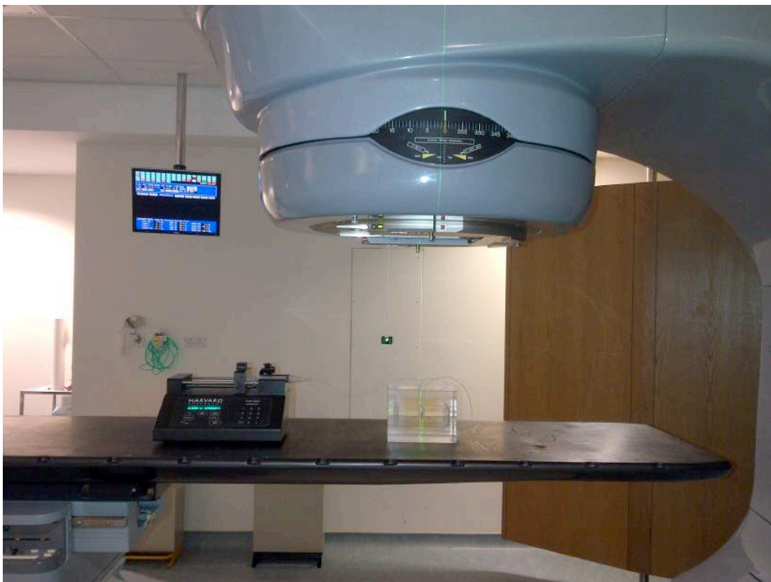
Figure 2.4 Photographs showing the linear accelerator (above) and the microfluidic device in the perspex block lined up with the head of the linear accelerator (below).
