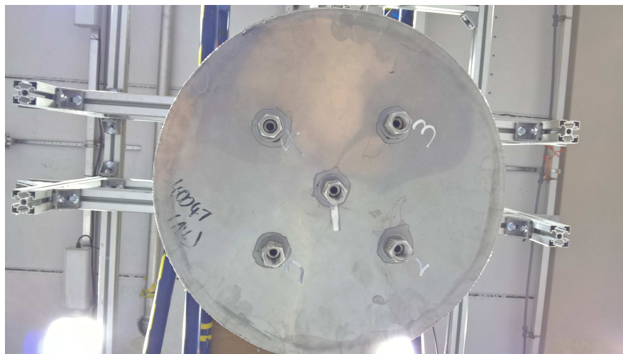
Fig. 6.3 Five pressure sensors installed at the bottom of the buoy.
