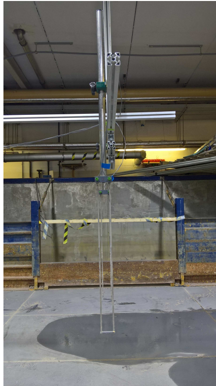
Fig. 6.8 Wave gauge installation for wave tank tests.
