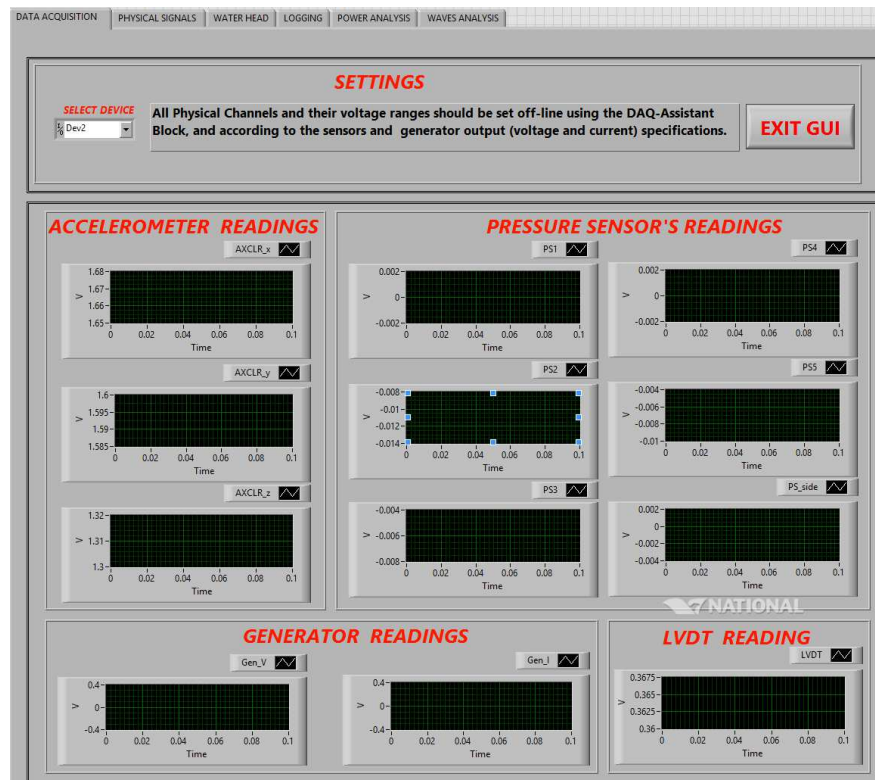
Fig. 6.11 Data acquisition GUI coded in LABVIEW™.
