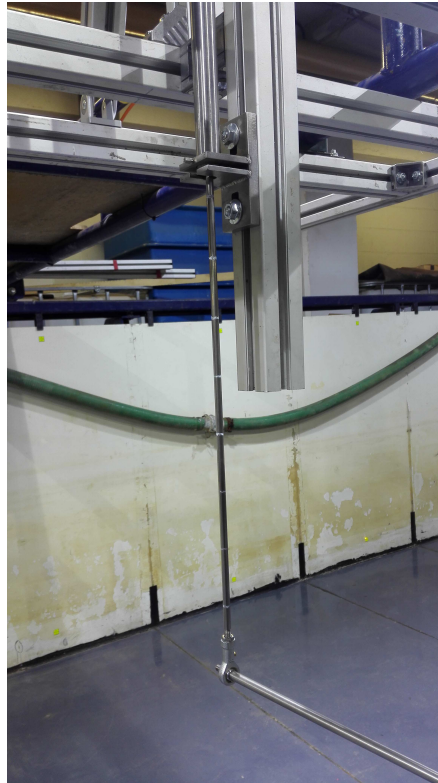
Fig. 6.6 The connection of the LVDT to the PAWEC and wave tank gantry.
