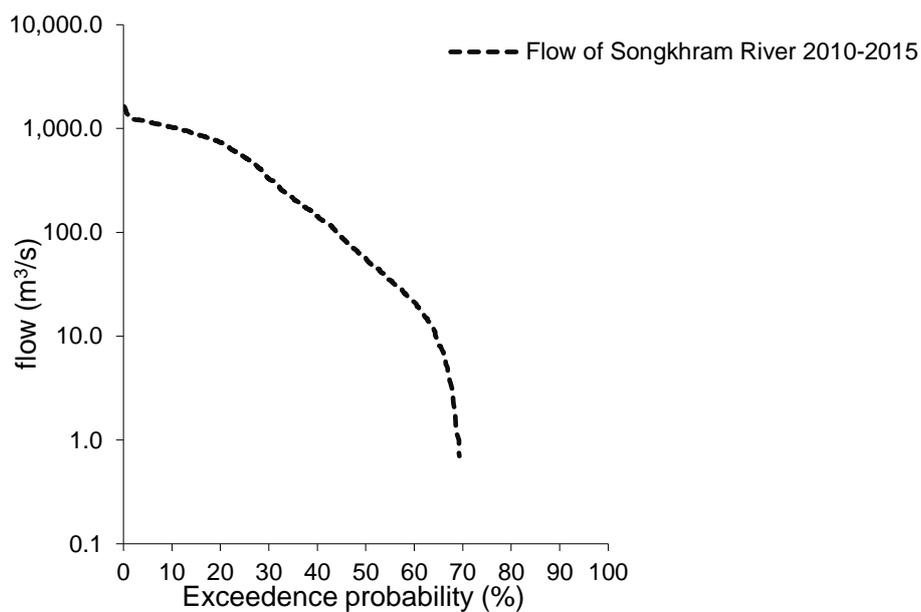
Figure 3.11 Flow duration curve of Songkhram River from 2010-2015. The flow duration curve in Songkhram River does not move towards 0 on the Y axis because the data comprise many zero flow days caused by watergate closure in the dry season.
