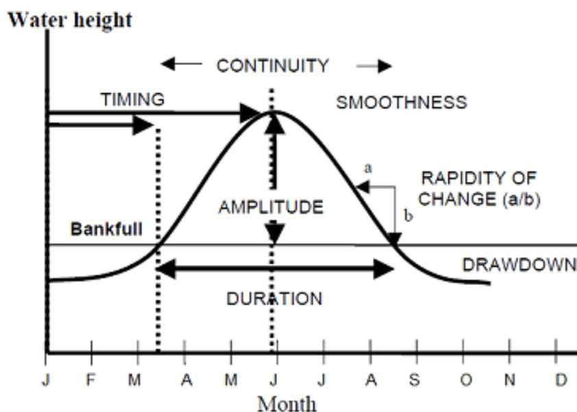
Figure 2.7 The important parameters of flood curve having biological significance (after Welcomme *et al.* 2004).
