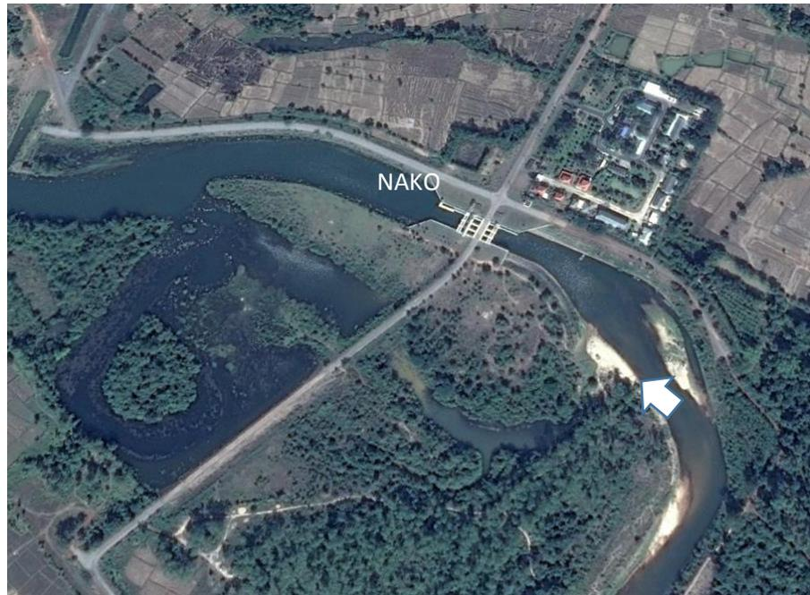
Figure 3.14 Disconnection of floodplain and the main stream river at the downstream of Na Koo watergate at the post-operation period (2011-2014). The arrow shows the disconnected floodplain caused by sedimentation at the downstream area of the Na Koo watergate.
