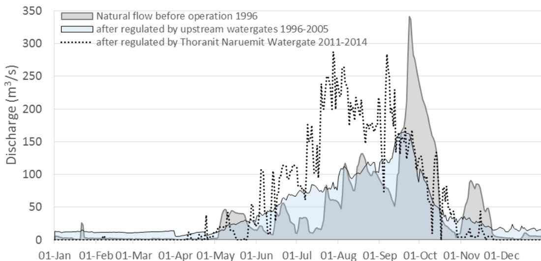
Figure 3.9 Annual discharge of Nam Kam River at the most downstream watergates (2011-2014) compared with the period before operation (1996-2005).
