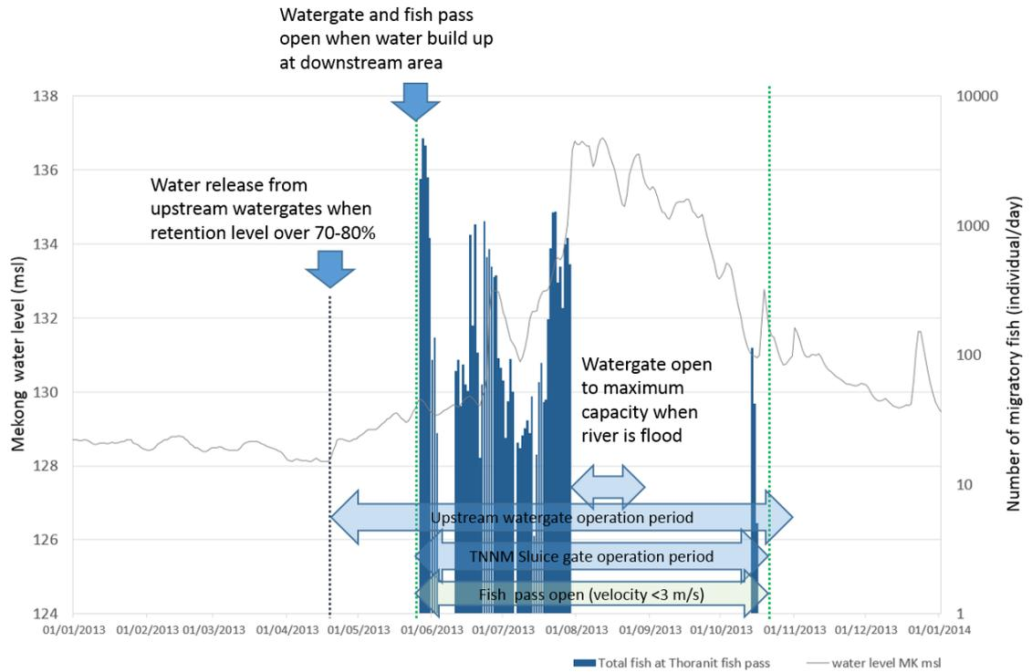
Figure 3.3 Flood cycle of the Mekong River and watergate and fish pass operation schedule in the Nam Kam River system.
