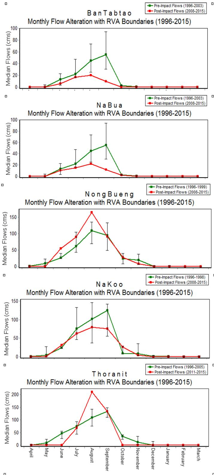
Figure 3.6 Median monthly flow alteration at each sampling sites in Nam Kam River and its tributary from pre-operation period and post-operation period of all watergates. The upper and lower boundary for RVA based on pre-impact data are also shown as upper and lower ranges of the pre-impact flow.
