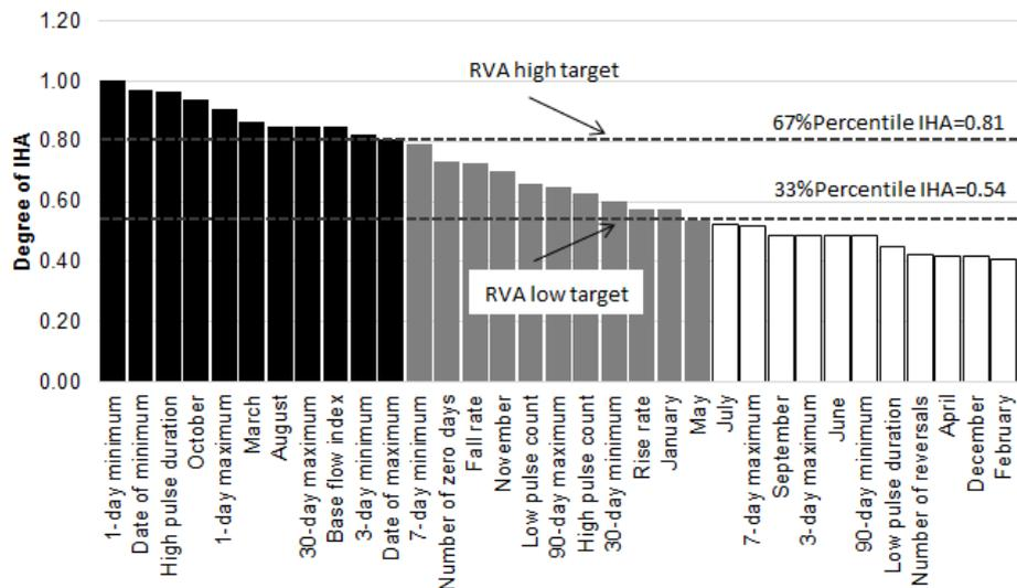
Figure 3.17 Ranked median absolute degrees and percentile value of 33 indicators of hydrologic alteration for 5 watergates on Nam Kam River system.
