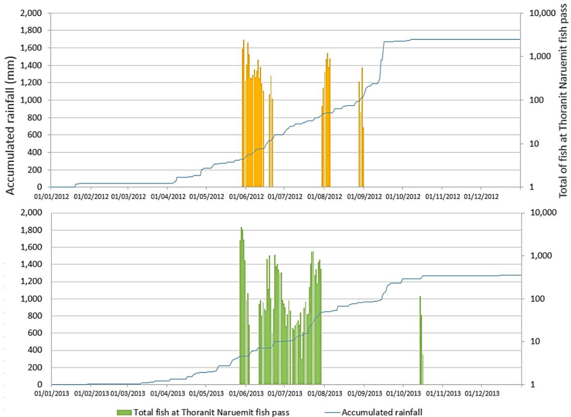
Figure 7.15 Accumulated rainfall at Thoranit Naruemit watergate and number of fish that migrated through the fish pass during 2012-2013. (Sources; Ngoichansri *et al.*, 2013 and this study)
