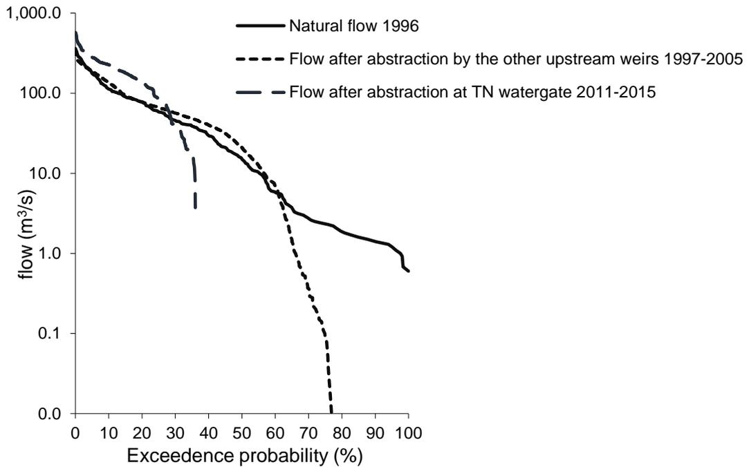
Figure 3.10 Flow duration curve of Nam Kam River at the most downstream watergate, Thoranit Naruemit. The flow duration curve after abstraction by the others upstream watergates does not move towards 0 on the Y axis because the data comprise many zero flow days caused by watergate closure in the dry season.
