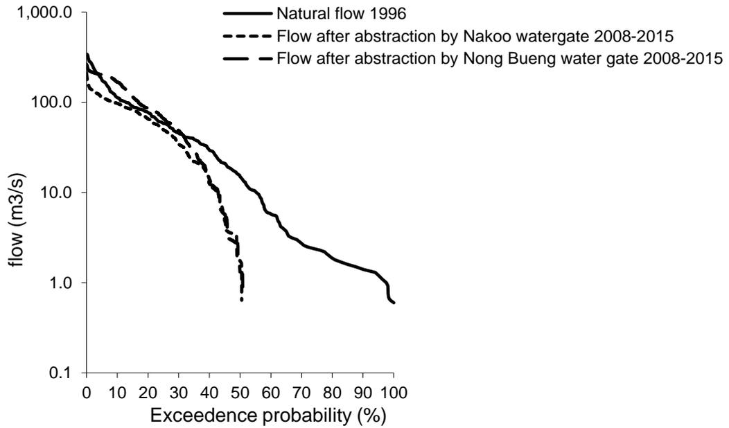
Figure 3.7 Flow duration curve of Nam Kam River before and after modification by upstream watergates (Nong Bueng and Na Koo). The flow duration curve after abstraction by Na Koo and Nong Bueng watergates does not move towards 0 on the Y axis because the data comprise many zero flow days caused by watergate closure in the dry season.
