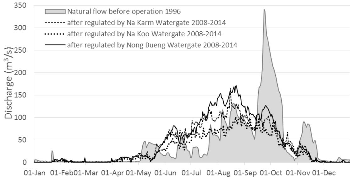
Figure 3.4 Annual discharges at three upstream watergates in the Nam Kam River before (1996) and after (2008-2014) upstream watergates construction.
