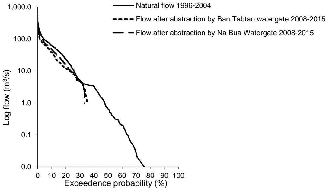
Figure 3.8 Flow duration curve of Nam Bang River before and after modification by watergate operation. The exceedence probability at the pre-alteration period does not reach Q100 because the river was stagnant more than 20 percent of the year. The flow duration curve after abstraction by Ban Tabtao and Na Bua watergates does not move towards 0 on the Y axis because the data comprise many zero flow days caused by watergate closure in the dry season.
