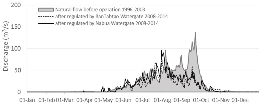
Figure 3.5 Annual discharges at two upstream watergates in the Nam Bang River before (1996-2003) and after (2008-2014) watergate construction.
