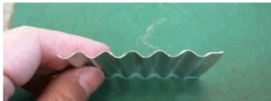
Fig. 4-18: Change of the corrugation form. Fig. 4-19: Final wave form in side view.
