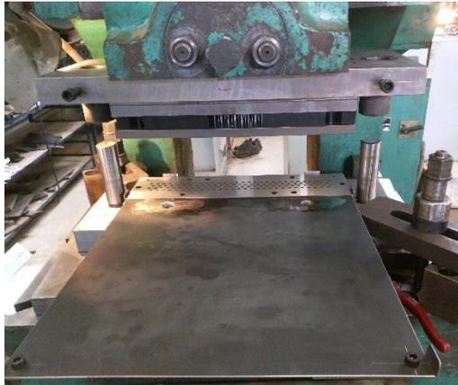
(a) Punching mould in position
