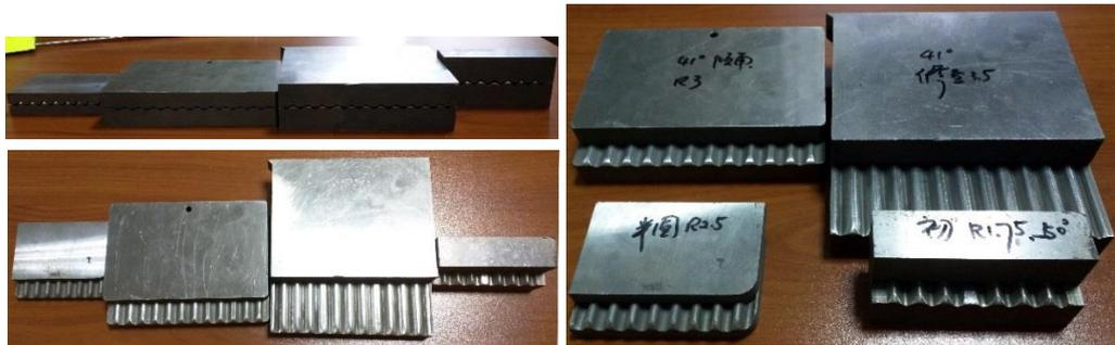
**Fig. 4-16:** Some of the small-scale sheet moulds for trial.
