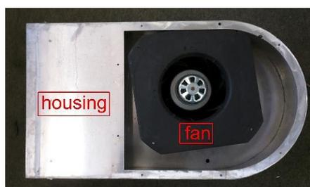
**Fig. 4-41: Fan and housing.**
