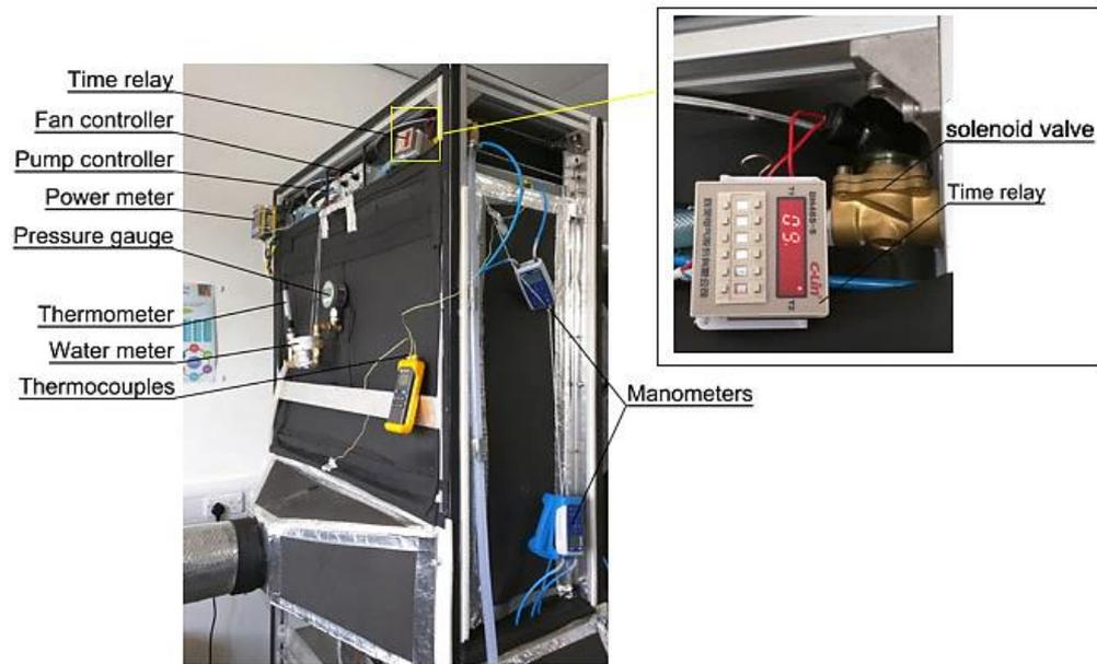
**Fig. 5-6: Layout of the measurement instruments and control elements.**
