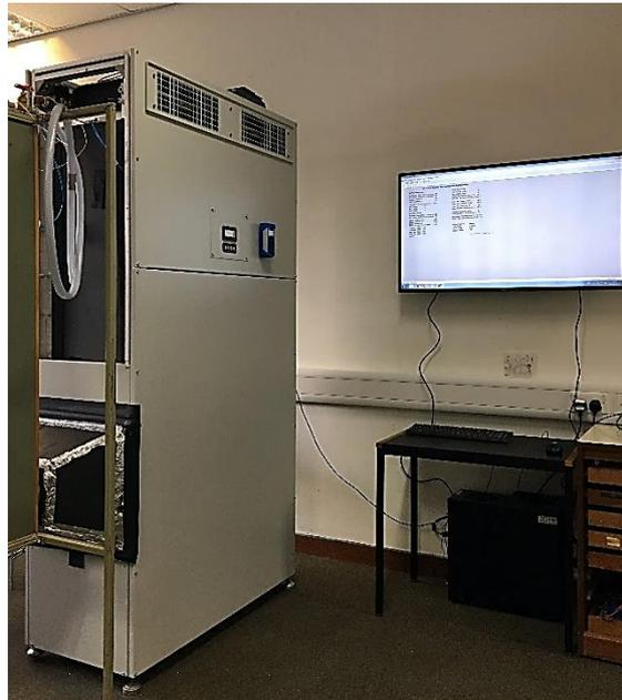
**Fig. 5-11: The proposed dew point air cooler prototype in demo operation.**
