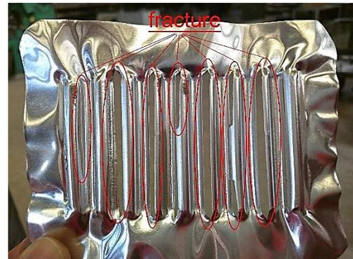
Fig. 4-15: Fractures after mould pressing.
