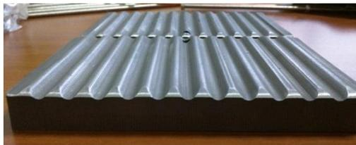
Fig. 4-14: Trial mould pair.
